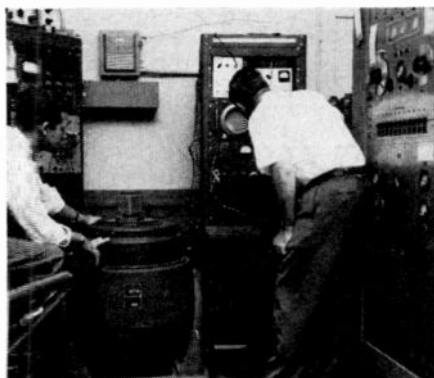
This vibrator for measuring conformance to M I-Specs is an important part of the extensive equipment in Bourns Reliability Assurance Laboratory.
