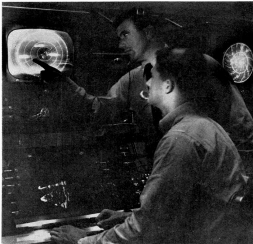
Televised markers (known as shrimp boats) identify radar blips as incoming planes in new scan-conversion system for air traffic control
