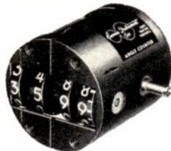
ANGLE COUNTER 1503. Counts from 000.0° to 359.9° and returns to 000.0; Input speed: 1800 rpm max. int., 500 rpm cont.; Weight: 2.5 oz.; O.D.: 1.310 in. Typical of many Bowmar designs currently being manufactured.
