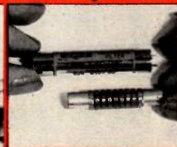
Weldmatic pressure gage reads firing force...calibrated from 0 to 50 lbs., insures exact weld pressures from job to job. (Right) Welded filter cartridge and completed miniaturized Collins filter.
