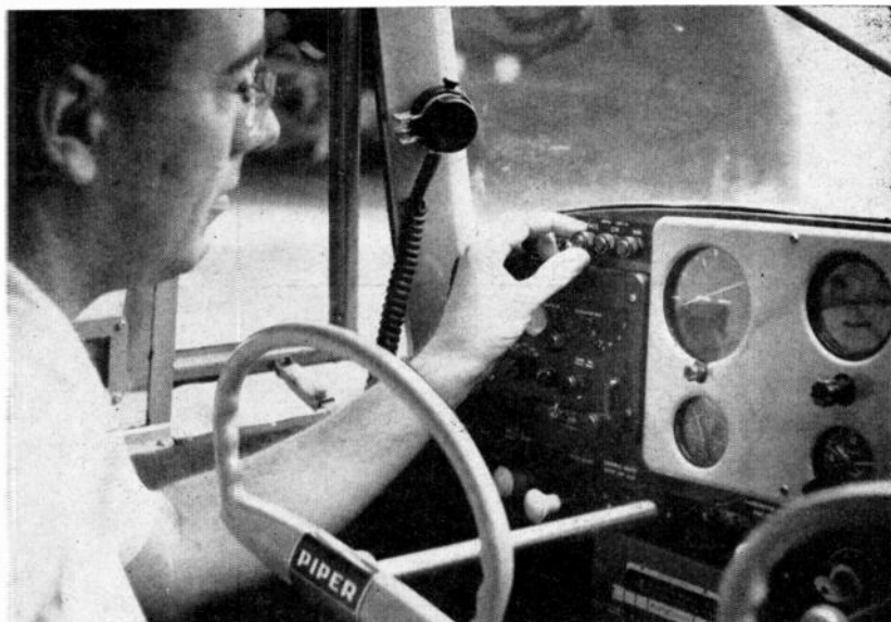
FIG. 3—Pilot adjusts brightness of indicator on marker beacon receiver. Reverse side of front panel is specially labeled to permit vertical mounting
