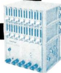
MINIATURIZED AMPLIFIERS STACKED ON POWER SUPPLY
