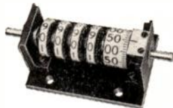
SPECIAL DECIMAL COUNTER 2660. Counts from 000000 to 999950 with return to 000000, in 50-unit increments. Input speed: 1000 rpm max. int., 300 rpm cont.; Weight: 3 oz.; Length: 2.33 in. Typical of many Bowmar designs currently being manufactured.
