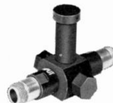
New solid-state limiters that protect receivers without external bias.
