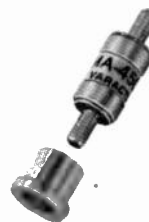
New Varactor diodes that reduce receiver noise to as low as 1 db.
