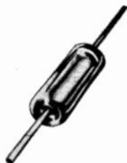
New computer diodes with recovery times lower than 4 m \mu secs.
