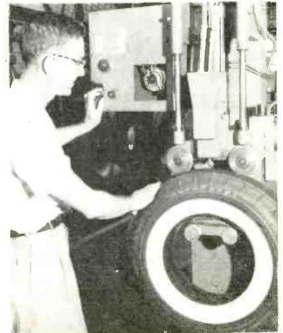
Variations in tire tread thickness are recorded at Goodyear electronics laboratory
