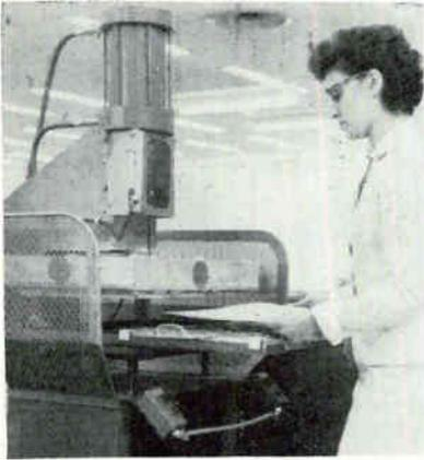
Tray is placed in machine and covered with coated card
