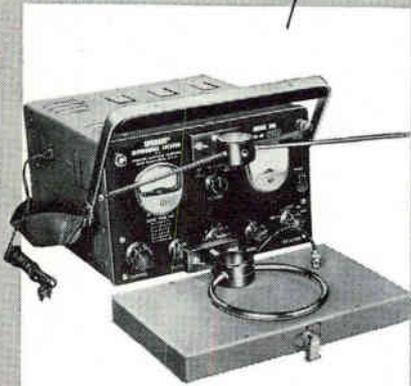
This improved instrument is a compact, rugged and highly sensitive interference locator—with the widest frequency range of any standard available unit.
