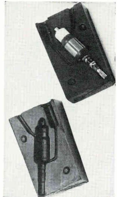
strips should be introduced before mold half is poured, at those areas subject to greatest flexing. Use special silicone release agents in the epoxy mold each time, to minimize sticking of potting compound.
