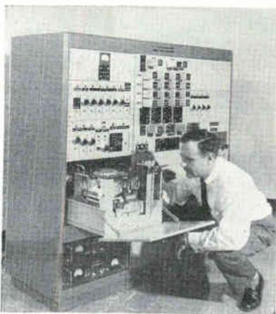
**THE FRONT COVER**—Overall view of the analog computer. The left hand cabinet contains the power supplies, the output recorder and two rows of amplifiers. The center cabinet has the plug board for the analog networks, the meters for reading temperatures and heat flow, and storage space for spare networks. The right-hand cabinet contains two rows of amplifiers and the radiation function generator
