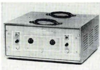
put impedance selection 4, 16, 64, 600 or 2,400 ohms. Frequency response of the matching transformers is 30 cps to 150 kc  $\pm$  2 db at extreme impedance values. The transformers can handle up to 20 w of power with distortion at less than 1.5 percent.
