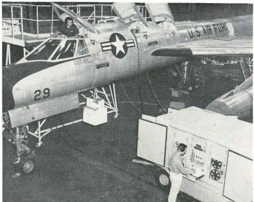
Computer on wheels (lower right) makes 750 tests of the B-58's control system in 90 minutes. Without the "go" or "no go" equipment, spot testing takes two days. Unit, built by Eclipse-Pioneer div. of Bendix, simulates all command signals to the Hustler autopilot from the air data computer, accelerometers, gyros, radio navigation gear and other air-environmental and direction references
