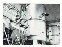
Vertical Ram hydrogen atmosphere furnace
