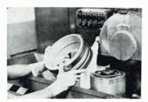
Jig for surface grinding
