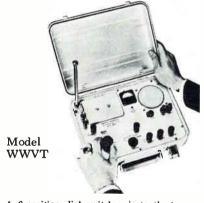
A 6-position dial switches instantly to any Standard Frequency — 2.5, 5, 10, 15, 20 or 25 mc. It is small, light-weight and rugged sealed metal case and potted components, all transistorized and battery operated, and has better than 2 mv sensitivity. Priced at
