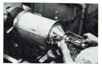
Machining copper parts
