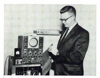
New damping material, developed to reduce structural response to white noise, is examined by R. C. Henshaw, Lord's manager of operations, after evaluation test. Panel is constructed of a special broad-temperature-range elastomer sandwiched between metal sheets, and bonded to them. These structures are available in sections or laminated panels which may be added to existing hardware
