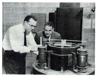
Internally-damped cantilever beam (right) and conventional aluminum beam (left) tuned to the same frequency are examined by J. Ruzicka, development engineer, and E. Pietz, President of Barry. Their damped beams utilize viscoelastic materials sandwiched between metal plates. These techniques, which now help solve missile vibration problems, will be explained at the coming IRE show
