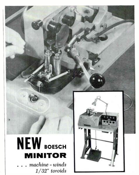
The coil shown above is a 1/32" residual I.D. toroid being wound by machine on Boesch's new Model MW400 MINITOR. It's the smallest machine-wound coil ever made (only half as large as the smallest previously available), and it can only be wound on MINITOR!
