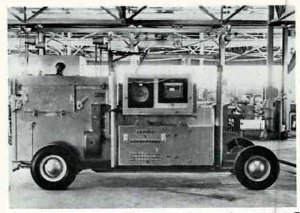
Electronic controller-recorder programs temperatures of -100 to 200 F to test missile components in Cook Electric's environmental unit
