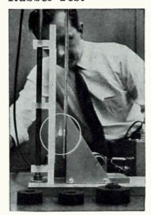
Impact of steel ball on test material electronically measures energy absorption for Chevrolet designers
