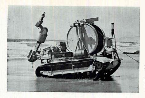
RUM (Remote Underwater Manipulator), returning from Pacific floor, carries sonar, four tv cameras, mercury vapor lights — powered and transmitted via cable (right)
