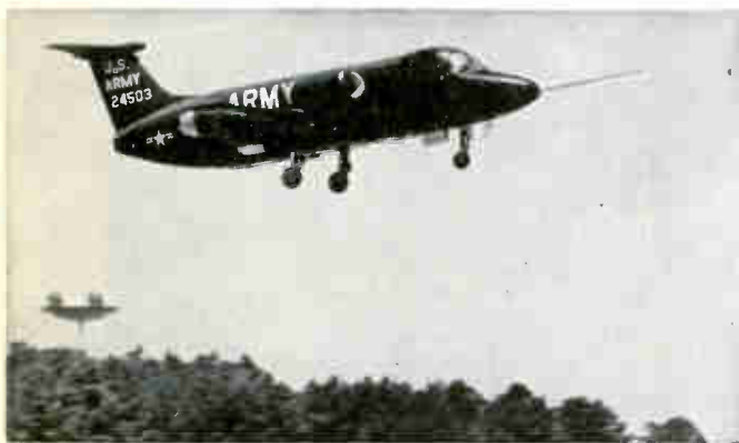
TILTING PROPELLER system is used in Curtiss-Wright VTOL aircraft. Full scale mock up shows two of the four props. Speed range planned is zero at hover, 460 mph in regular flight
