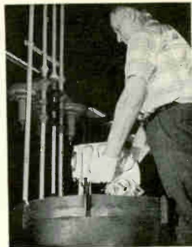
TUBE ASSEMBLY is removed from furnace making metal-ceramic seals
