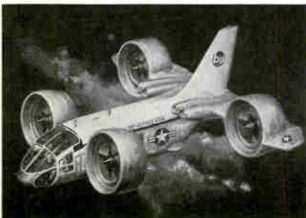
VTOL TRANSPORT uses ducted propellers in artist's illustration of research aircraft built by Bell Aerosystems Co. Speeds to 350 mph in conventional flight are expected in this military craft
