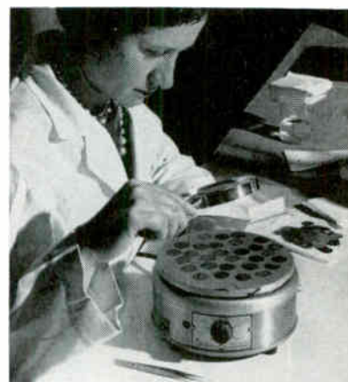
PROCESS has minimized rejects of disks subjected to microscopic inspection for flaking porosity and adherence
