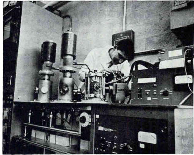
Micron-thin coatings, applied to bearings and other rolling and sliding surfaces by Erica Fliege and A. F. Kaspaul of CBS Laboratories (left) may hold important promise for aerospace components. At right, electrical and mechanical tests on slip ring assemblies coated with the dry lubricants show that operating life of these assemblies in high vacuum and high pressure systems can be extended up to 100 times
