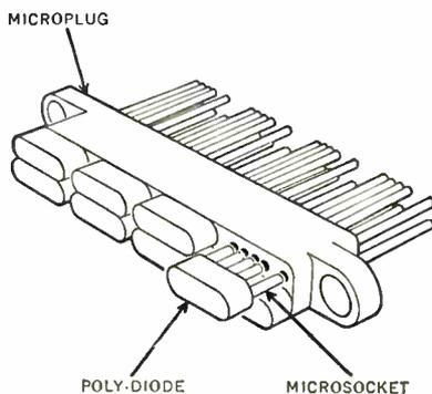
Nanopins\*, currently under development, are for those who wish to incorporate a quick-disconnect capability into their modules on .025 centers. It is identically constructed to the Micropin, but is half its size.
