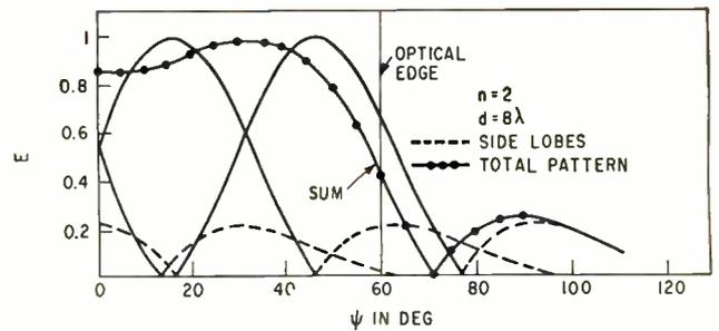
FIG. 3—Calculated synthesis of Cassegrainian pattern
