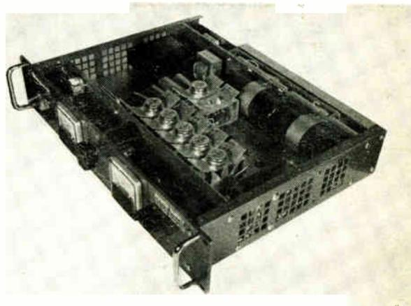
*Power supply equipped with plug-in radiators illustrates open construction and shows efficient circulation attained in stacked racks*
