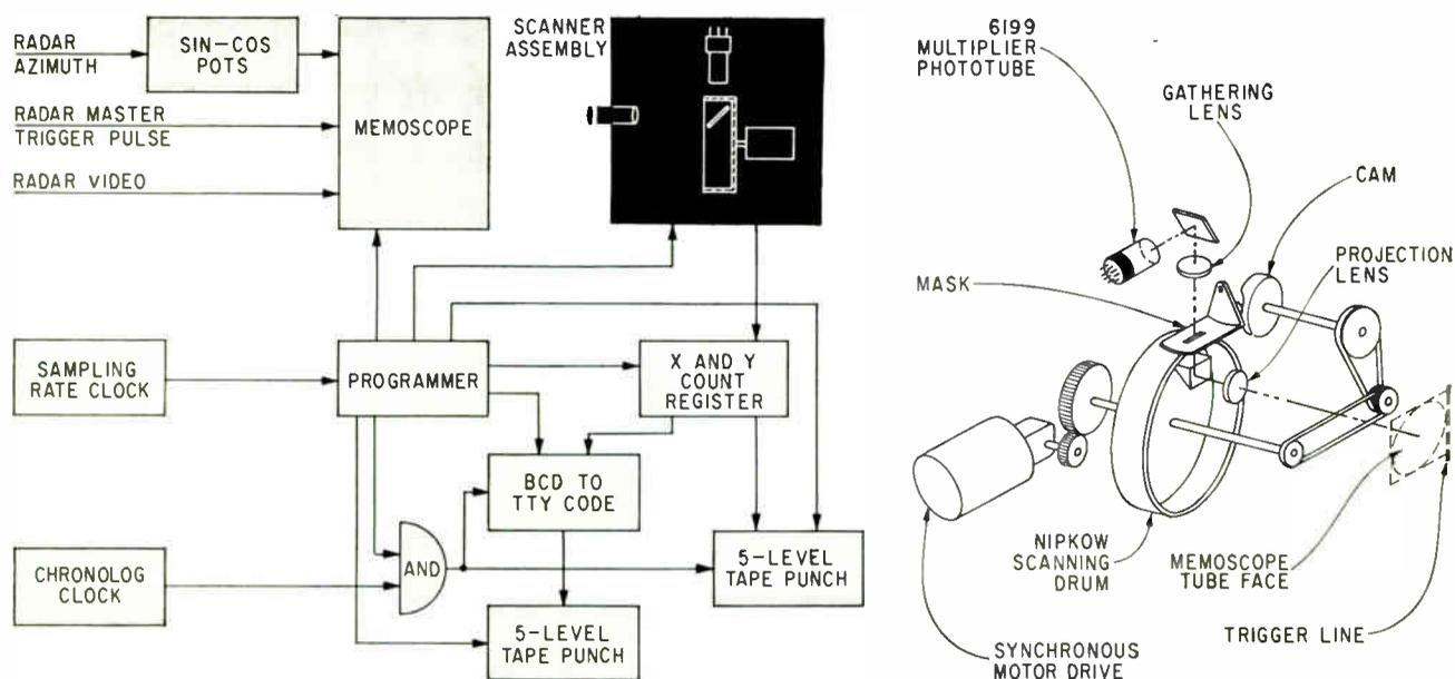
Block diagram of scanning system (left); optical and mechanical components of scanning system (right)
