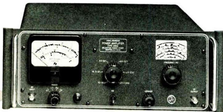
The new Signal Generator Power Amplifier Type 230-A is the ideal solution to your high RF power requirements including receiver testing, wattmeter calibration, antenna testing, filter and component testing, and attenuation measurements. The amplifier may be conveniently driven with any conventional signal generator and is designed to reproduce AM, FM, and pulse modulation characteristics of the driving generator with minimum distortion.
