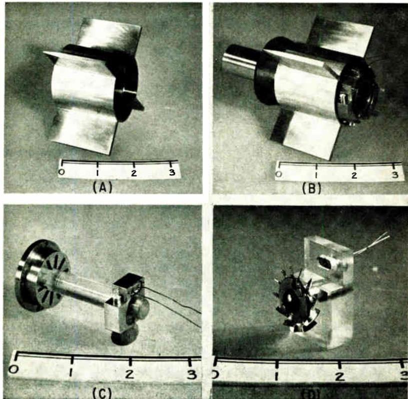
FIG. 4—Finned tail (A) has internal mirrors on inside surface that successively reflect light to tachometer (B). Phototransistor in (C) receives light pulses from reflecting faces of gear teeth. An angular reflection model is shown in (D)
