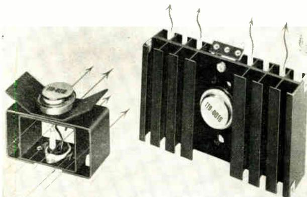
*Forced air stream applies lateral circulation of air in heat sink at left. Heat sink at right illustrates a typical convection cooler*
