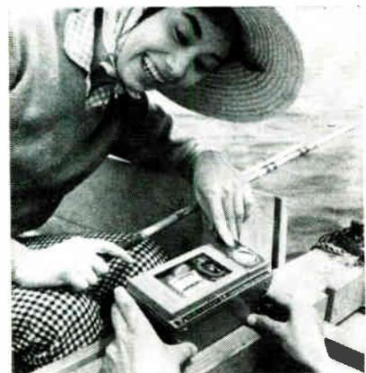
*Nippon Electric calls this gadget a fish camera. It's a transistor sonar set. Frequency is 200 Kc, maximum depth 200 feet, price in Tokyo \$110*
