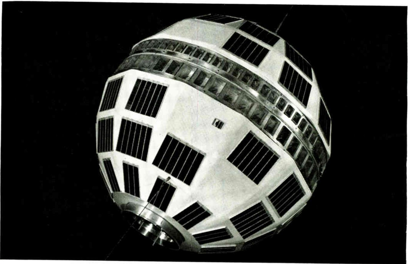
*Model of Telstar experimental communications satellite. The dual row of slotted antennas can be seen around the equator of the sphere. Patches of solar cells on the shell convert sunlight into electricity to provide power.*
