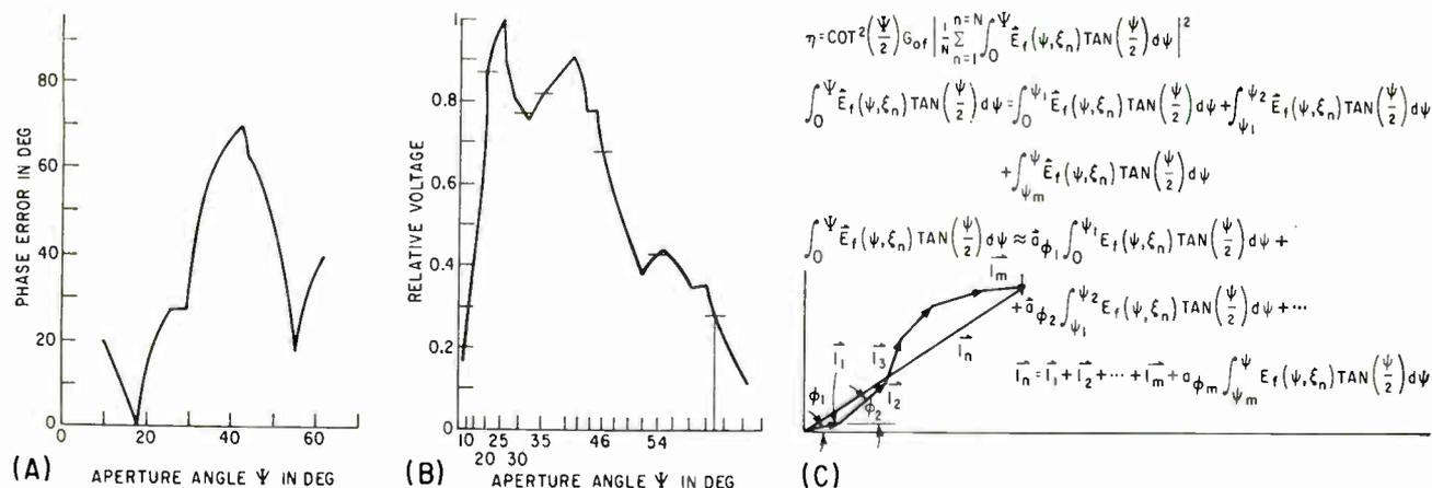
FIG. 7—Phase error plot, 45-deg plane,  $\theta = 18.4$  degrees (A); aperture integration plot, 45-deg plane,  $\theta = 18.4$  degrees (B); and vector integration diagram (C)
