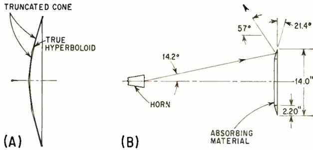
FIG. 2—Conical approximation (A); scatterer (B)
