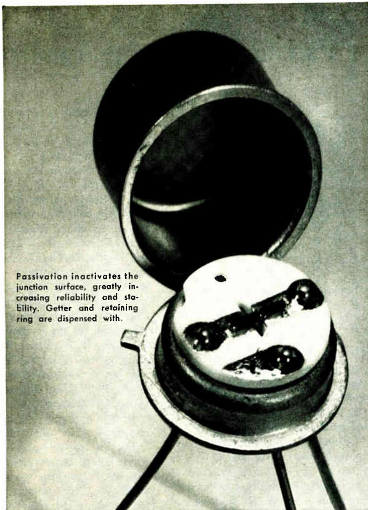
Passivation inactivates the junction surface, greatly increasing reliability and stability. Getter and retaining ring are dispensed with.
