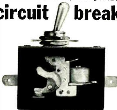
Most circuit breakers (and all fuses) depend on thermal effect for actuation. The Heinemann circuit breaker operates on magnetic flux. Its actuating element is a solenoid coil. It senses actual load current directly.
