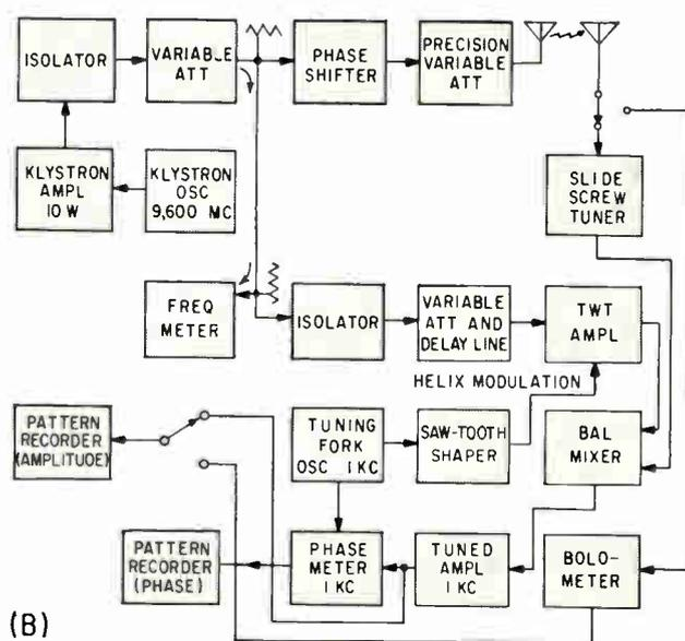
FIG. 6—Spillover plotted against flange angle (A), and Serrodyne phase measuring system (B)
