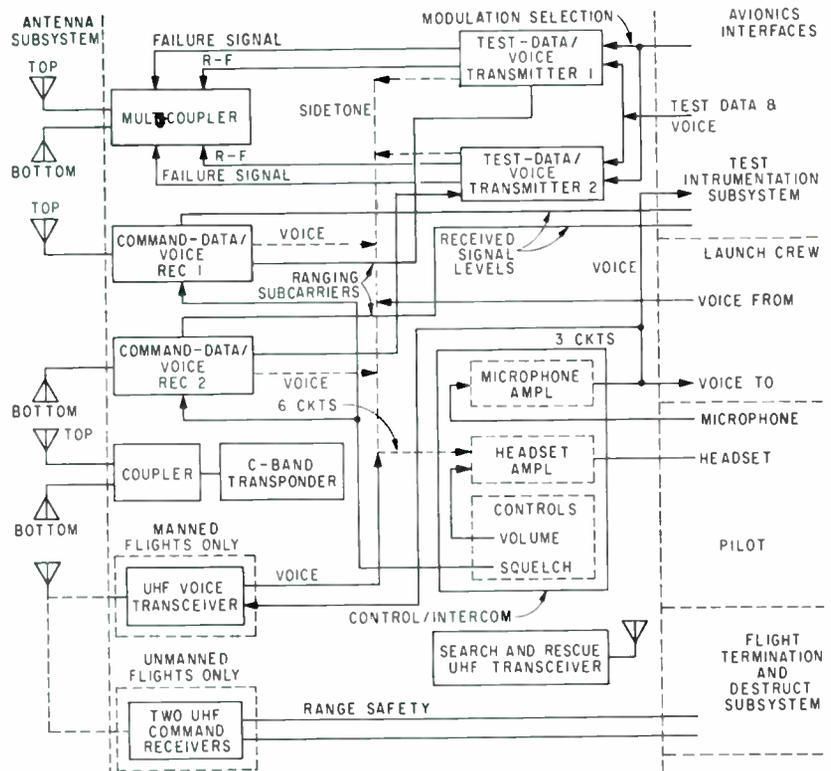
Airborne equipment—two transmitters and the microphone amplifier in the control panel are the airborne portion of the shf vehicle-to-surface link. Two receivers, converter decoders, and pilot's headset amplifier in the control panel are the surface-to-vehicle shf link
