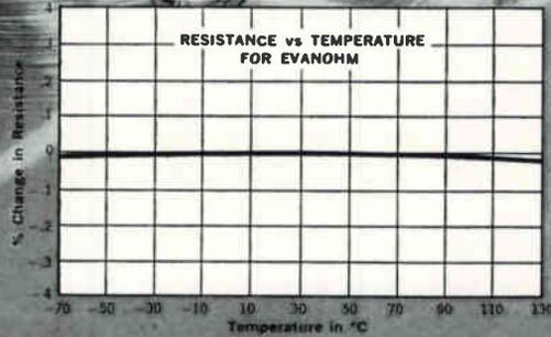
Specify EVANOHM for exceptional stability over wide temperature ranges. This WBD precision resistance alloy provides high specific resistance, low temperature coefficient and low thermal EMF to copper. It is especially recommended for high reliability applications... resistors, precision instruments, missiles and critical equipment. Available in bare wire, enameled or insulated.
