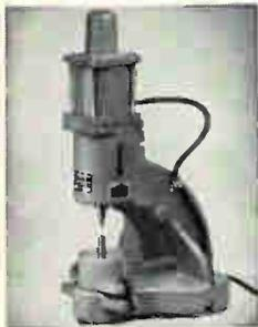
**SHORT RUNS:** Electropunch — sets hand-fed terminals twice as fast as conventional methods, solves terminal setting problems for as little as \$163. All electric. Foot-switch operation.
