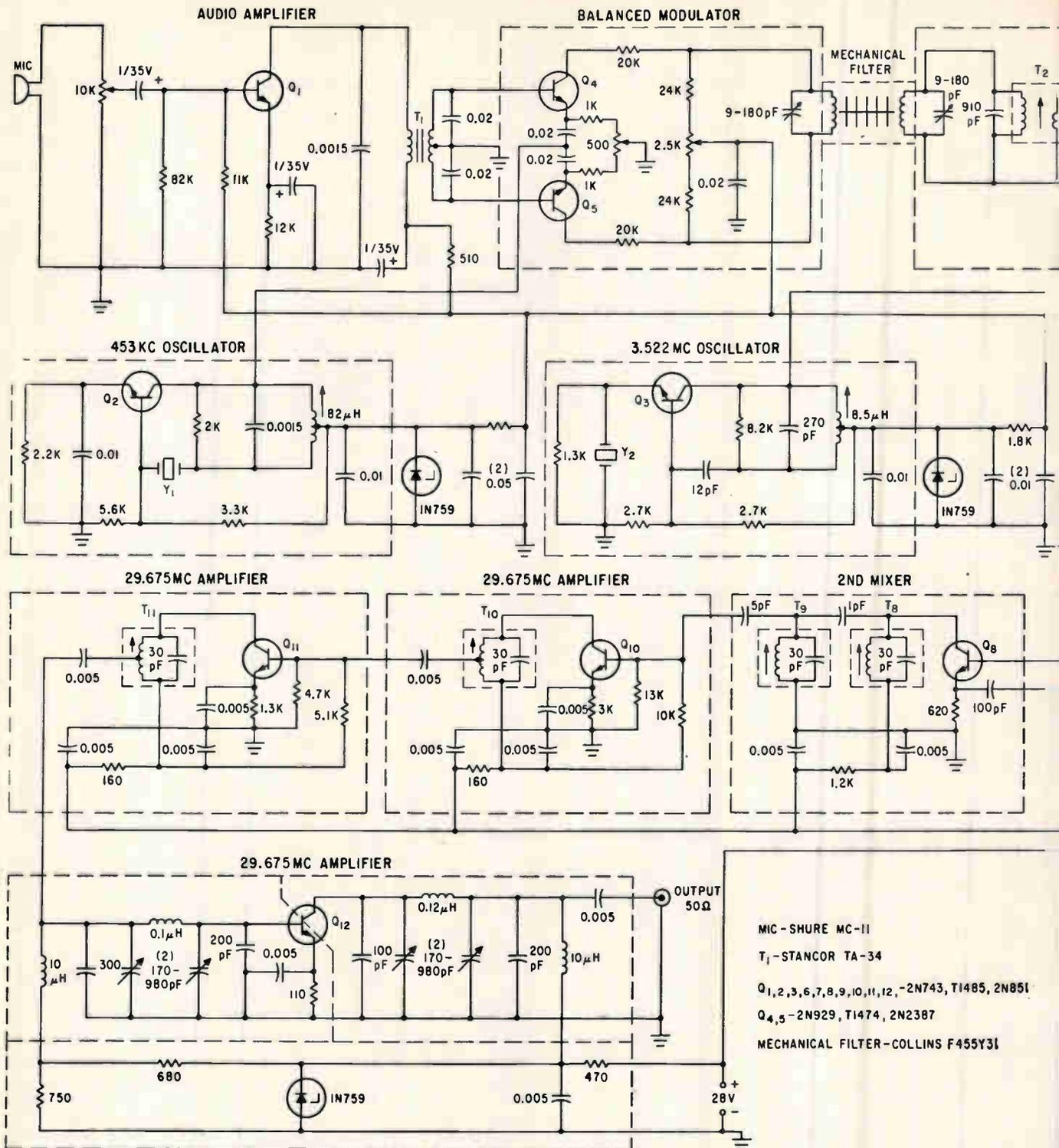
UPPER OR LOWER SSB frequency synthesis can be obtained with this 10-meter single-sideband exciter—Fig. 2
