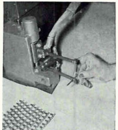
CONTACT CONTAMINATION is one of the major causes of trouble in relays and choppers, and a major source of contamination is the solder flux used for making internal connections and sealing the cans. Cambridge Scientific Industries, Cambridge, Md., has therefore turned to spot welding for internal connections in their choppers and to heliarc welding for sealing the can.
