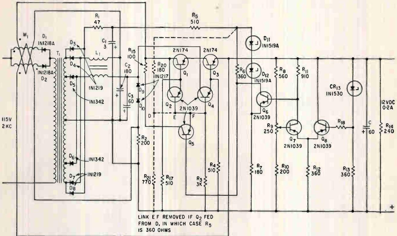
THIRD SUPPLY delivers bias to zener  $D_{11}$  and control transistors. Alternative method of controlling auxiliary output is shown by dotted connections—Fig. 3
