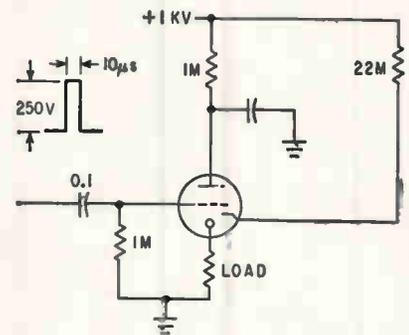
ators, and have been used as high energy film markers, photomultipliers and shunting devices. The sketch shows typical operation in a trigger circuit. (302)
