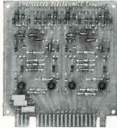
Here's an economical way to provide for clocked reset in a flip-flop register operating reliably at speeds up to 10 mpps. Any number of flip-flops can be used, and all can be reset simultaneously by the single reset command.
