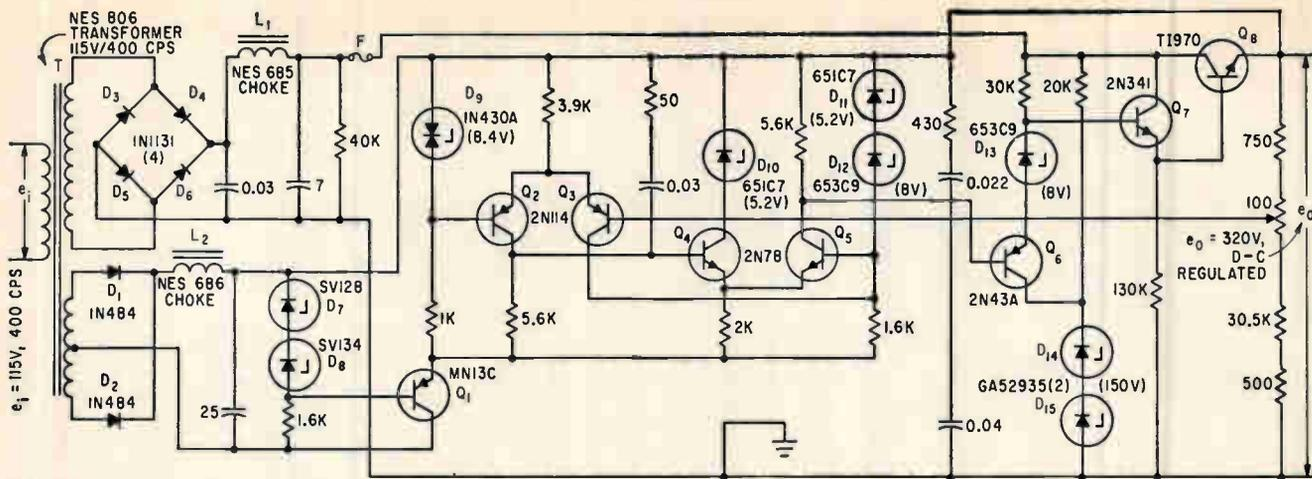
REFERENCE POWER SUPPLY relies on a temperature-compensated silicon junction zener diode as the basic reference element with precision wire-wound resistor network to obtain error signal—Fig. 2
