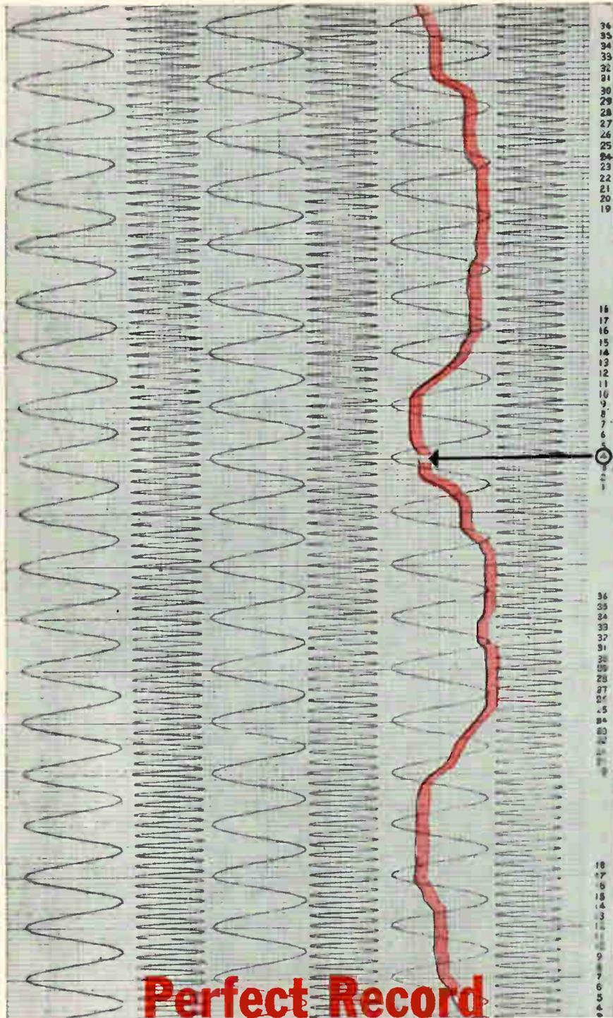
CEC's Type 5-123 Multi-channel, Direct-print Recording Oscillograph gives you: complete front access; twelve discrete speeds from 0.1 to 160 ips; easily interchangeable, self-contained major modules; direct rack mounting; 36 or 52 active channels; trace numbering; and optional DATAFLASH for record access time sixty times faster than any other printout process. All of which adds up to a perfect record every time. More data? Call your CEC office or write for Bulletin CEC 5123-X5.
