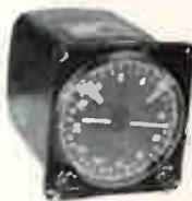
Mfr. Summers Gyro-scope Company. 115 volt A.C., 400 cycle, 3 phase. Contains direct reading gyro with caging mechanism and power failure indicator. Hermetically sealed case. 5" dia., 0 to 360°
