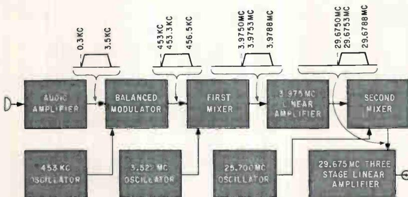
SSB EXCITER for upper sideband frequency synthesis—Fig. 1
