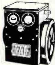
Type AG, frame 364Y, 7.5 kw, 3428 rpm, pi .95 Star connected 120/208 3 phase, 22 amps. Delta connected 120 volt single phase 6 amps. Self excited. Complete with control box, voltage regulator, AC voltmeter and frequency meter. Shaft 1" dia., 2" long; overall dim. of unit: 21" x 6 1/2" x 20".
