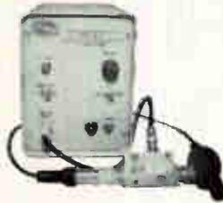
The AEL Modulator is a typical application of AEL solid state crystal switches for square wave or pulse modulation of signal sources to achieve greater power output with wide frequency bands
