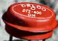
This is the new DTS-400 from Delco Radio . . . one of the highest voltage silicon power transistors available. The DTS-400 offers  $V_{ce0}$ ,  $V_{cb0}$  and  $V_{cs}$  of 400 volts. Because of its high voltage capabilities and its ability to withstand high temperatures, this transistor offers a significant advancement in the art of power conversion.
