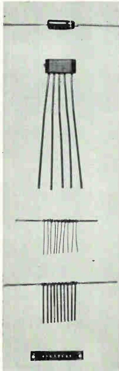
*DIODE UNITS illustrate evolution from standard glass component, top, to direct-wired poly diode with four junctions plus common lead, next. Third unit from top is ribbon strip with leads welded, followed by ribbon strip with sweat-soldered connections. Bottom unit is ribbon strip in matrix for direct mounting on etched circuit board connectors.*
