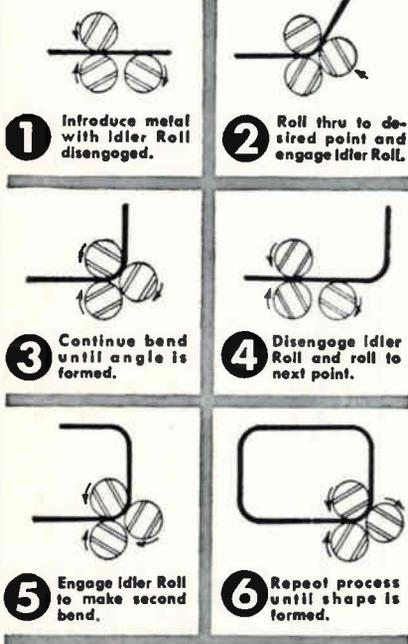
Forming small and large circles without flat spots and a variety of other sheet metal shapes is easily accomplished on the Di-Acro Roller with its exclusive cam actuated Idler Roll. Rear roll indicators allow operator to quickly return to a previous setting. Eight models from 6" to 42" forming width.
