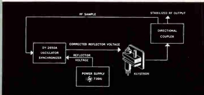
The DY-2650A is essentially a crystal-controlled superheterodyne receiver terminating in a phase comparator. An oscillator sample is mixed with harmonics of the rf reference to produce an intermediate frequency of 30 MC, which is compared in phase with the 30 MC reference. For stabilizing a klystron, the resultant phase error voltage is added in series with the klystron reflector power supply voltage.
