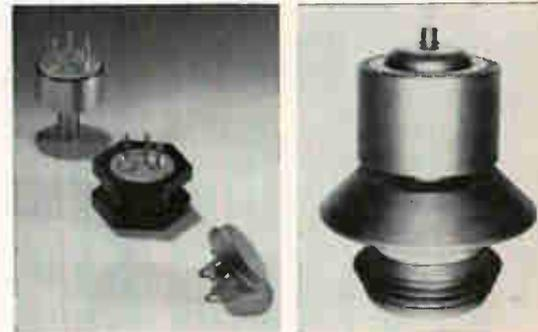
NEW FLAT PACK (left center is being used by Minneapolis-Honeywell for 65-amp transistors. Eimac is showing vapor-cooled high-power tetrodes (right)
