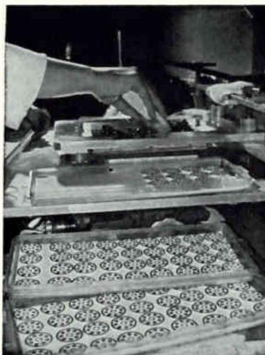
METALIZING COMPOUND is applied to octal tube headers by silk screen process
