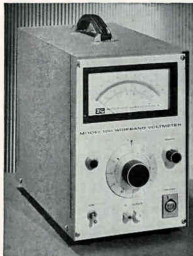
taneous viewing during measurements. When used as a wideband preamplifier, output impedance is 50 ohms with a rise time of less than 6 ns. Gain stability is assured by over 100 db of negative feedback. There is a complete absence of low-frequency jitter either due to amplifier noise or line transients. Change of range is by interstage attenuator.
