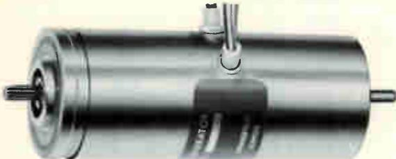
**NEW** FEATURE ADDED TO SIZE 10 and 11 MOTOR GENERATORS Sangamo's standard size 10 (.938" dia.) and size 11 (1.062" dia.) servo motor generators are now available with a rear shaft extension to permit mechanical coupling and/or speed checks after the unit is installed. Positive alignment is assured by the use of three ball bearings in each unit.
