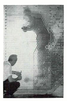
NO LOSS in physical strength and more electrical efficiency is claimed for metallized plastic antenna lens shown above. Sperry's SPG-49 radar, which is used to guide the Navy's Talos shipboard air defense missile, has plastic lens system that company says produced twice the signal gain of an earlier metal version.
