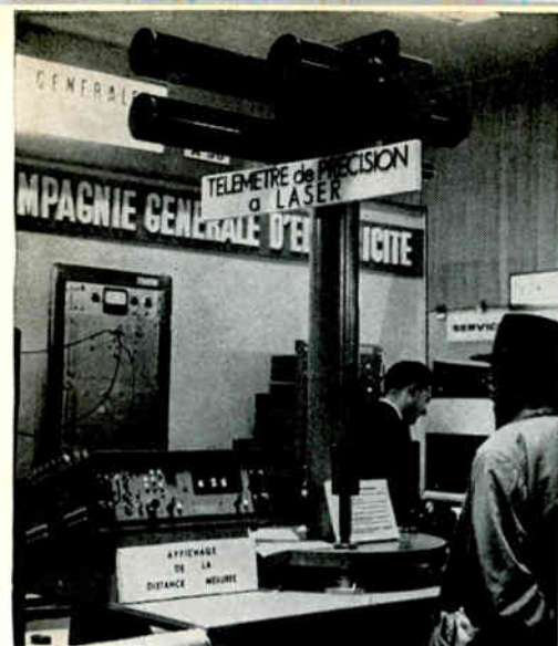
RUBY-LASER telemeter shown by CSF directly reads out range with an accuracy of 2 meters at 10 kilometers
