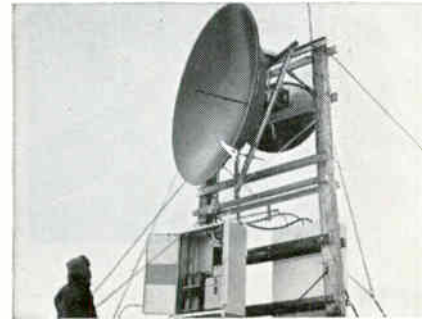
Merrimack Valley Laboratory, Mass. We were increasing the capabilities of a new microwave system designed for low-cost telephone and television communications over distances up to 200 miles. This system is based on advances in solid state technology.
