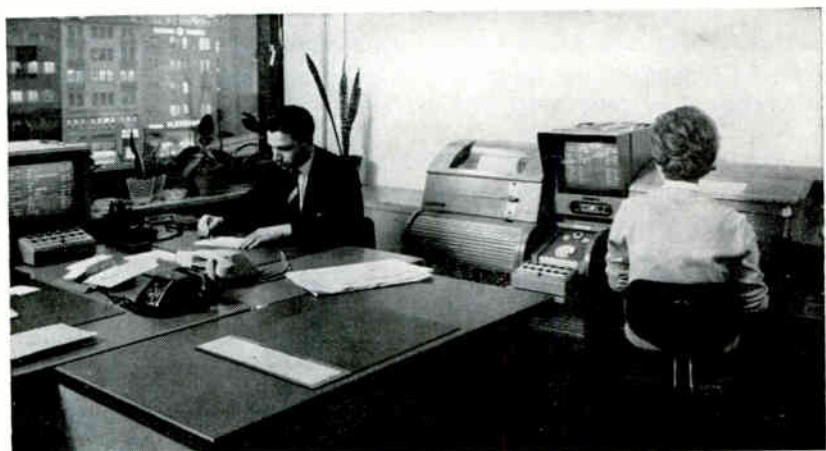
STOCK EXCHANGE in Duesseldorf, Germany, has installed stock quote display on which brokers can remotely post prices of stocks they specialize in. Brokers can also review prices with closed circuit tv system (above) that the exchange plans to extend through Ruhr region
