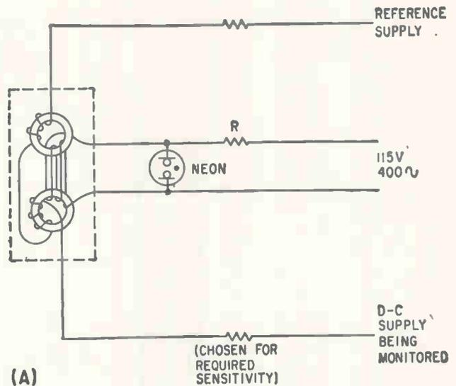
REDUCED inductance of saturated core (A) permits of different polarity (B), two control windings are
