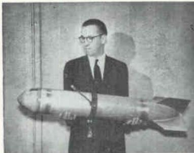
BOMB-SHAPED transmitter is fitted in flight with vertical 10-ft dipoles above and below, and a 18-foot trailing dipole
