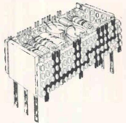
**TYPICAL ministac circuit with wiring on side mouldings; dark side-sections are wiring punched from standard material**
