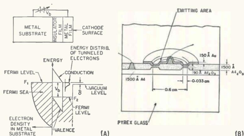
**ENERGY relations (A) and one type of construction (B) for tunnel cathodes**—Fig. 6
