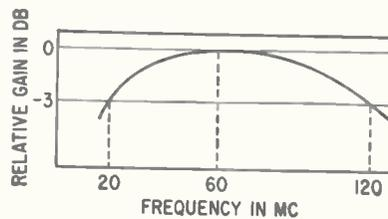
GAIN characteristic of a single log i-f stage—Fig. 2
