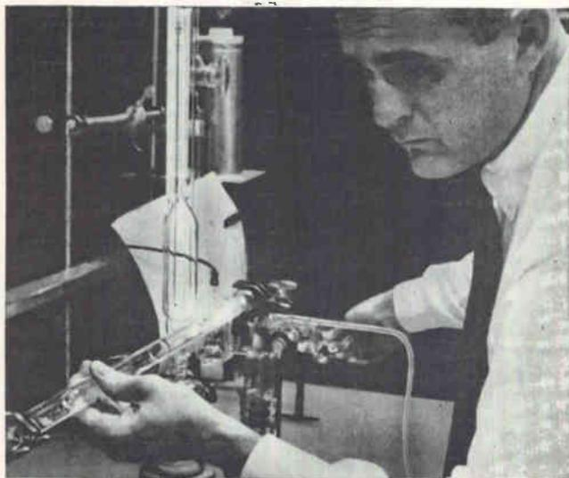
*In this method of preparing ultrapure gallium arsenide, gallium reacts with arsenic in a quartz tube with oxygen added under pressure to suppress dissociation of  $\text{SiO}_2$ .*
