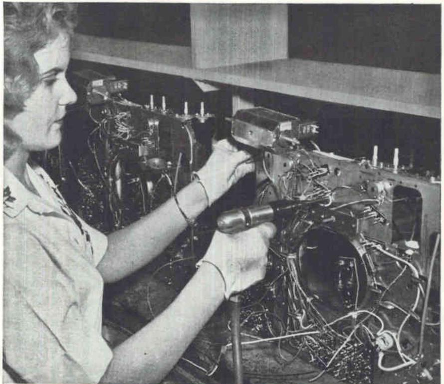
Make permanent, solderless connections that remain gas tight under severe corrosion and vibration conditions. More than 15 billion connections have been made this way—without a reported electrical failure.
