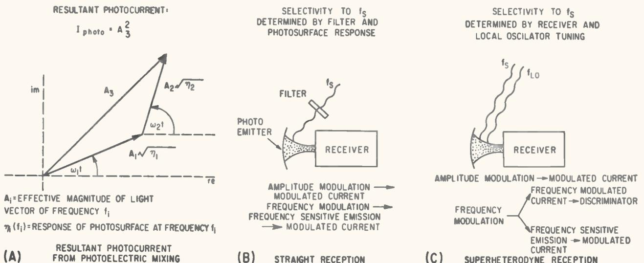
PRINCIPLES of photoelectric mixing (A), examples of modulation detection (B) and (C) by interaction with the electrons, and Siegman's frequency-modulation detector (D). These techniques may provide a way to generate submillimeter
