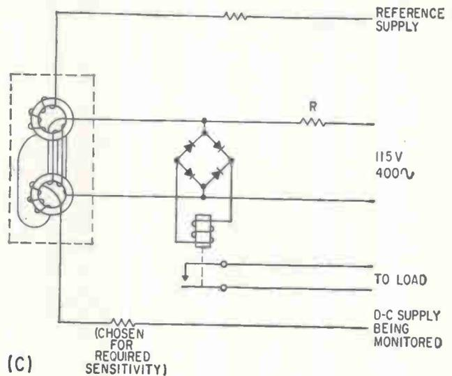
high value of 400-cycle current, turns off indicator through large drop in  $R$ . With reference and monitored supplies used. Sensitive relay can be used instead of indicator lamp (C) if remote indication is needed
