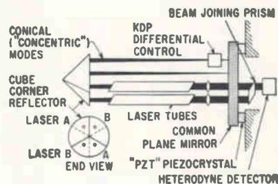
**DOUBLE CAVITY** for laser frequency standard described by Gordon Gould, of TRG, would have two independent laser oscillations going through the same reflector. Expected accuracy of locking onto center of spectral line is 1 part in  $10^{11}$
