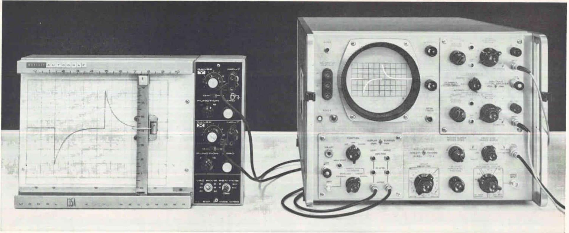
High resolution, permanent recordings of waveforms displayed on the hp 175A 50 MC Oscilloscope are now possible with the new hp 1782A Display Scanner Plug-in.
