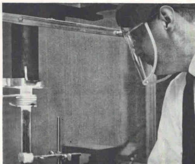
*In this alternative method, gallium arsenide crystals are pulled from gallium and arsenic melted in aluminum nitride crucibles, which do not liberate silicon contaminants.*
