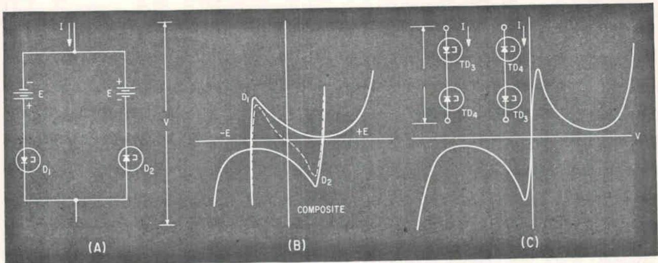
TUNNEL DIODE pair (A) produces the composite volt-ampere curve of (B). A series diode combination produces the curve of (C)—Fig. 1
