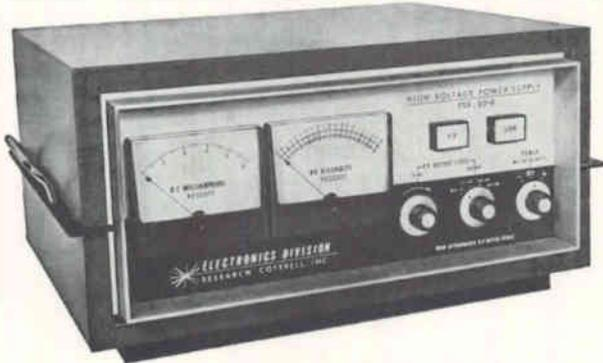
PSR Series, pictured above offer these important features: Range 5 to 30 KV, 2 to 30 MA • Regulation  $\pm .05\%$  • Ripple .1% RMS • Completely Solid State Circuitry • Light Weight • Rack Height 8 $\frac{3}{4}$ " maximum • Dry Insulation • Overload Protection • Reversible Polarity • Simplified Controls; coarse and fine voltage, ON-OFF meter reversing switch • Triple-Range Kilovoltmeter and Milliammeter. Write for New 1963 High Voltage Bulletin.
