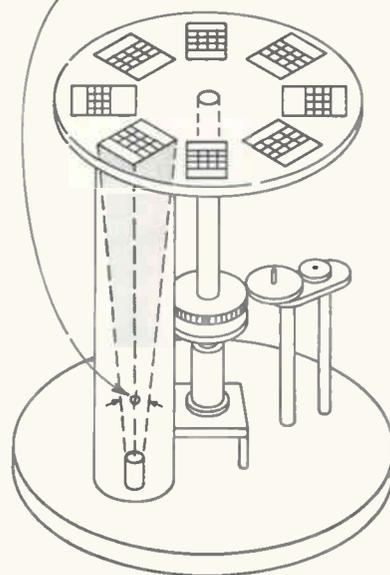
SEQUENTIAL process equipment (left) (vacuum chamber removed) deposits films on successive substrates with separate firings of source material. Diagram (right) shows how substrates are located far enough away from source material to subtend small area of minimum vaporization angle thus getting high depositional accuracy—Fig. 2
