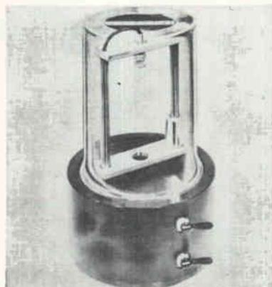
**Vacuum Chamber Tests Solid State Detectors**
