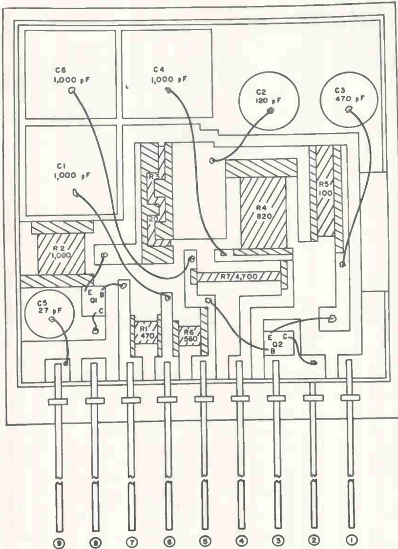
PHYSICAL LAYOUT of a log i-f module with resistors, capacitors and transistors identified—Fig. 4
