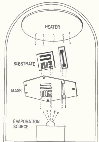
FABRICATION of thin-film circuits is performed using a vacuum evaporation system—Fig. 3
