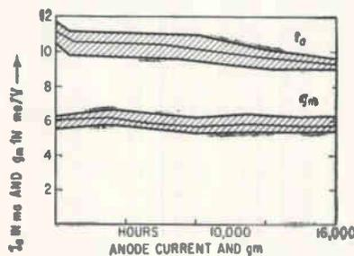
in blocking oscillator and similar circuits. Maximum pulse duration is 5 microseconds, peak plate voltage is 1,000 volts. (302)
