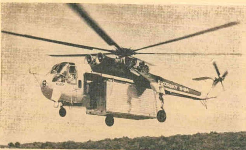
SOLID-STATE , semiconductor load cells allow pilots of Sikorsky S-64 Skycrane helicopters to control engine torque more accurately during lifting and in-flight operations. The cells, developed by Fairchild Camera & Instrument, include a convoluted-cylinder load-sensitive element coupled to a silicon semiconductor strain gage
