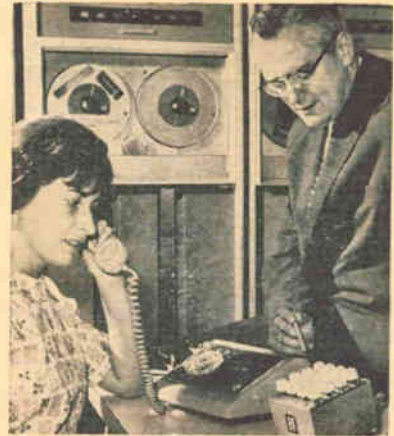
KEYBOARD (lower right) transmits inquiries over commercial telephone lines to a modified Honeywell computer, which processes them and responds with a voice answer. The system can handle as many as 28 different inquiry routines
