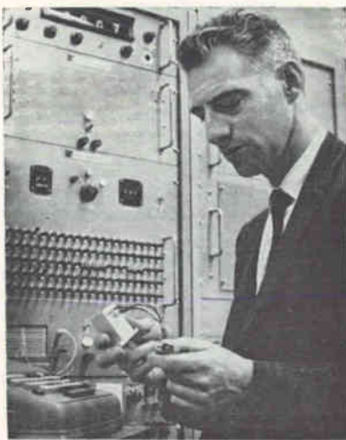
AUTHOR examines a servo accelerometer, one of a hundred incorporated in the automatic testing system
