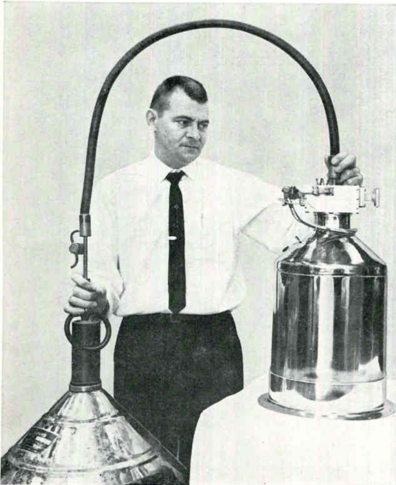
TRANSFER from storage dewar to operational maser dewar
