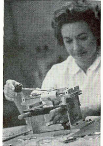
AUTOMATIC processing equipment is employed in the Helipot Ceramic Engineering department to form the basis of cermet resistance elements
