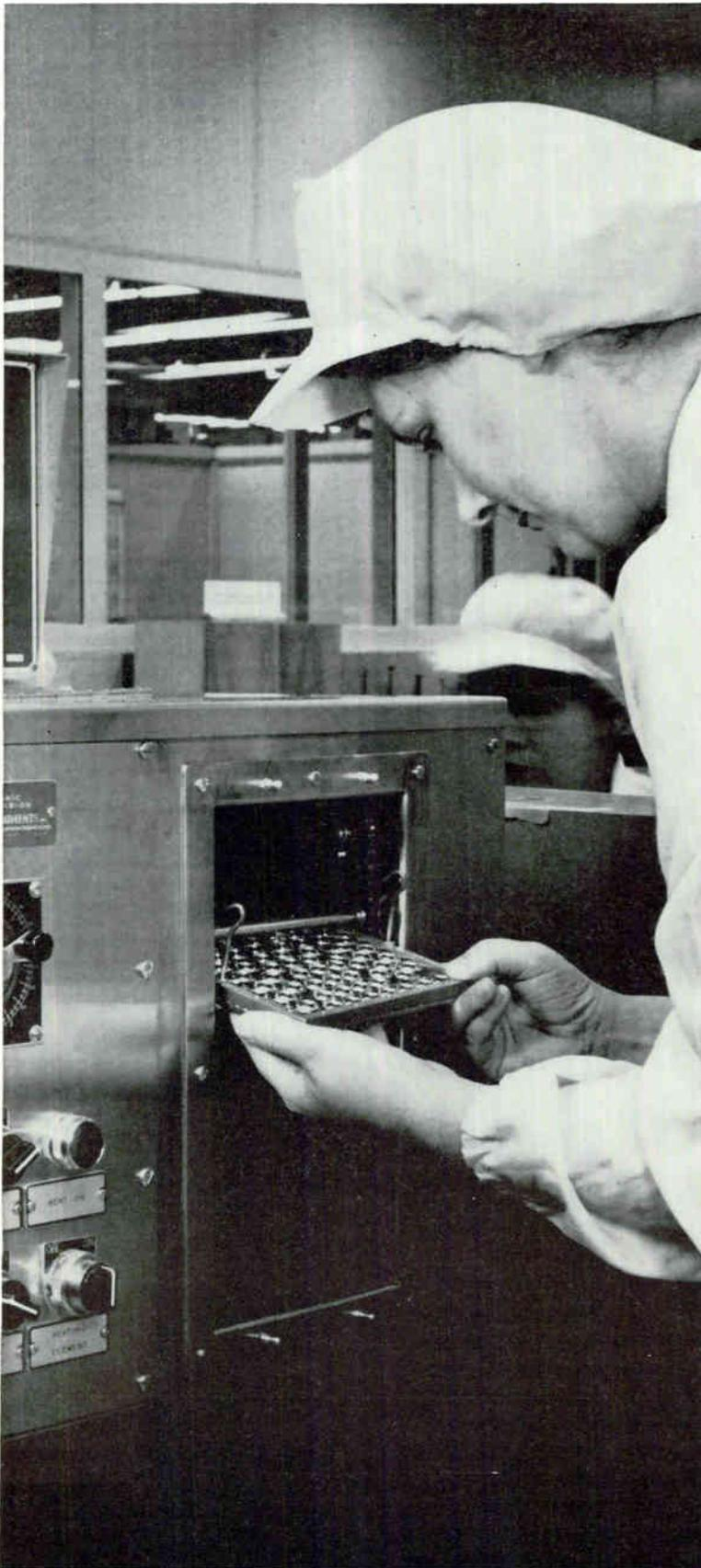
**PROBLEM:** Precision cleaning of assembled ball bearings for instruments used to be a time-consuming operation for the Barden Corporation, Danbury, Connecticut. Bearings up to 1" diameter went through a spray-cleaning machine at a relatively low production rate. Larger bearings were individually spray-cleaned.
