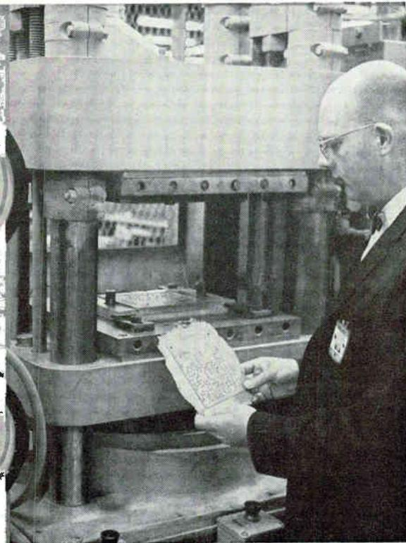
MOLDED BOARD is inspected by author Cichocki as it comes off molding press. Boards are made of glass-fiber-filled plastic
