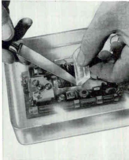
**Pot it.** Transparent or opaque, G-E silicones provide a resilient protection against moisture, ozone, thermal and mechanical shock. Flows freely around complicated parts, can be cut away to replace internal components.
