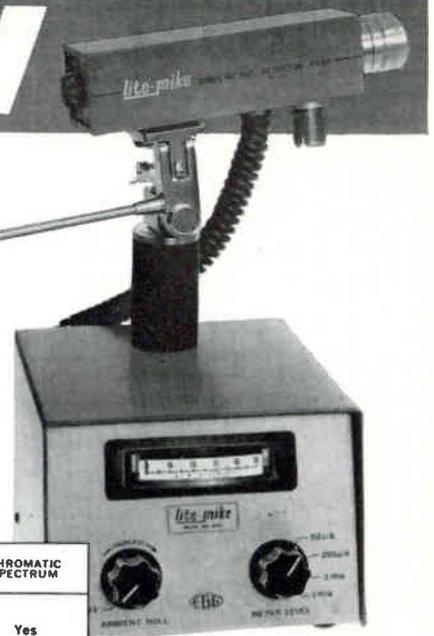
Compact (10" high) and lightweight, the EG&G LITE-MIKE has built-in controls for sensitivity and balancing of ambient light. Head is swivel-mounted for ease of alignment with source.
