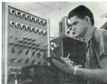
An IDS Technician checks out the PCM package using specially designed IDS test equipment. Each unit is individually checked for performance and workmanship and copies of test data are submitted with delivery.
