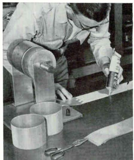
**Manufacture it.** RTV adhesive/sealants are fast working assembly tools, eliminate prefabricated parts or more costly, time consuming techniques. Here an RTV adhesive laminates flexible mica strips to form cylindrical ducts.
