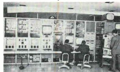
PENTAGON SYSTEM can distribute four different programs simultaneously to different viewing areas
