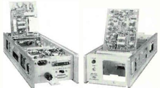
Major circuits of the DY-2460A are mounted on three plug-in etched circuit boards, which swing out for easy access. Sides, top and bottom are easily removed for servicing.
