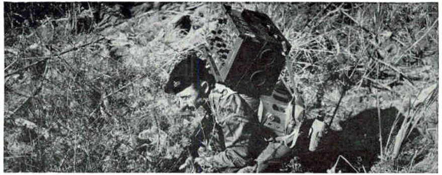
PARACHUTIST can drop behind enemy lines with 37-pound radio command pack to direct air and ground operations (Sylvania)
