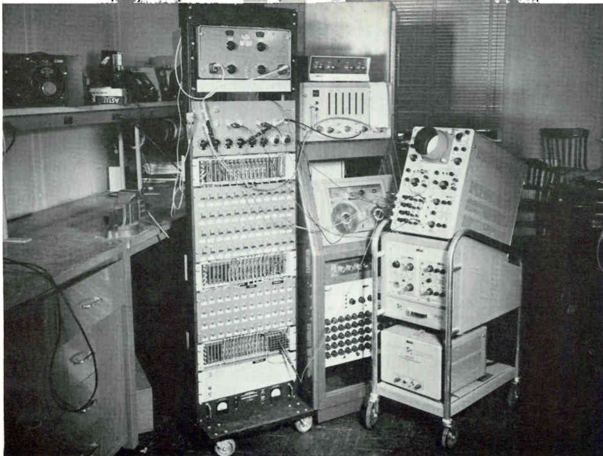
VOICE FUNDAMENTAL detector (left) is also used for cross correlation with fixed binary patterns. The bank of switches are used to enter fixed patterns into the memory
