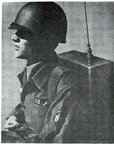
FOOT SOLDIER locates his position by same navigation system used by aircraft and ground vehicles. Low-frequency, hyperbolic system (AN/GRN-14) is built by Bendix-Pacific under license from Decca
