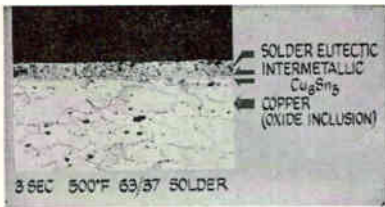
TINNED COPPER interface magnified 1,000 times. Intermetallic layer assures joint reliability
