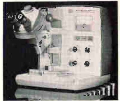
MICROWELDER lowers tip to work but pressure is dependent only on gram weights shown on right. Weights are placed on tip shaft
