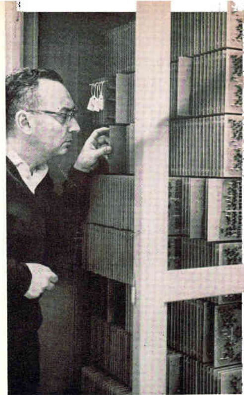
ARITHMETIC UNIT of Weizmann Institute's Golem computer, under construction in Rehovoth
