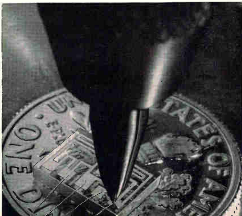
WELDER ELECTRONICS provides variable pulse trains by scr's to perform preheat and postheat of weldments. Voltage across electrodes is constantly monitored
