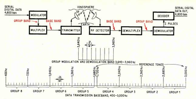
Multiplexing. Each group of eight data characters is first modulated in the groupband, 3,640 to 3,960 hz, and then multiplexed down to the voice, or baseband. The process is reversed at the receiver.
