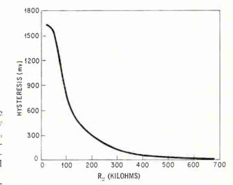
Hysteresis curve. Increasing the value of R<sub>a</sub>, minimizes or eliminates the circuit's hysteresis.
