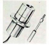
Linear position transducers series 230 are 60-hz units that provide infinite resolution. They are available in 20 different models with range of travel from  $\pm 0.010$  to  $\pm 4$  in. Units feature sensitivity to 100 mv/mil and linearity to 0.05%. A wide variety of standard mounting options simplifies installation of core and case. Robinson-Halpern Co., 5 Union Hill Rd., West Conshohocken, Pa. [364]
