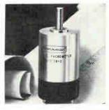
Temperature - compensated d-c tachometer 9011-2710-0 has an output gradient, with 100-kilohm load, of 7 v/1,000 rpm. Maximum deviation is no more than 0.01%/ °C change front  $-25^{\circ}$  to  $+75^{\circ}$ C. Ripple voltage is 3% max. Armature inertia is 6.5 gm-cm<sup>2</sup> max. Life expectancy is 10,000 hrs at 3,600 rpm at  $+25^{\circ}$ C. Beckman Instruments Inc., 2500 Harbor Blvd., Fullerton, Calif. [370]
