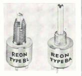
Half-inch-diameter variable resistors with conductive plastic element feature infinite resolution over a 50-ohm to 5-megohm range in sealed units with either standard (type BA) or locking (BL) bushings. Dust-, moisture-, and water-proof to 15 psi, they have an end resistance of less than 5 ohms each end. Reon Resistor Corp., 155 Saw Mill River Rd., Yonkers, N.Y. [345]
