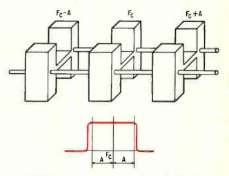
Broader bands. Frequency response can be made very broadband by mechanically coupling several resonators.
