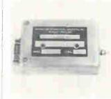
Logarithmic picoammeter model 12EN1126 is a 6-decade (120 db) current-to-voltage transducer capable of processing currents in the  $-1 \times 10^{-12}$  to  $-1 \times 10^{-6}$  amp range. Output is 0 at minimum input current and +5 v at maximum. Rise time is 9 msec maximum and noise is less than 50 mv peak to peak. Washington Technological Associates Inc., 979 Rollins Ave., Rockville, Md. **[375]**
