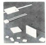
Fixed ceramic capacitors called High K Unicerams come in 17 sizes, the smallest being 0.07 x 0.035 x 0.04 in., and 3 voltage ratings (50, 100, and 200 wvdc). They meet or exceed requirements of M1L-11015C. Insulation resistance is  $10^5$  megohms- $\mu$ f at  $\pm 25^\circ$ C. Temperature coefficient is  $\pm 15\%$  max for  $-55^\circ$  to  $\pm 125^\circ$ C. JFD Electronics Co., 15th Ave. at 62nd St., Brooklyn, N.Y. [343]
