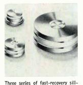
forme series of last-recovery sincon rectifiers are in flat-button form. The TR series is rated for 20 amps at 100°C case temperature. The RU series handle 40 amps and the RD units 200 amps. Both TR and RU have 500-nsec recovery times; the RD, 700-nsec recovery time. Piv ratings are from 50 to 1,000 v. Electronic Devices Inc., 21 Gray Oaks Ave., Yonkers, N.Y. 10710. [436]
