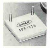
Model SPR-275 is a 21-w resistor designed to isolate line drive impulses and terminate lines within the demanding space requirements of a computer. It has a resistance range of 0.025 ohm to 1 kilohn, within 5% tolerance. Mounted to a heat sink maintained within the computer at 70°C, its maximum temperature on the other side 100°C at 21 w. Dale Electronics Inc., Columbus, Neb. [349]
