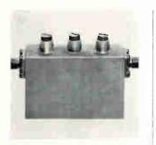
Tunable, coaxial bandpass filters series FBM span 960 Mhz through 6 Ghz in 2, 3, and 4-section combinations. They can be used as preselectors; to provide rejection for image frequencies in receiver front ends; and to eliminate harmonic or spurious signals from an oscillator multiplier chain. Prices start at \$150. Applied Microwave Dynamics Corp., 287 Sherman Ave., Newark, N.J. [401]
