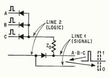
will be reflected from the open circuit, retaining its positive polarity. Because the reflected pulse and the incident pulse have the same polarity, the output is 1. To prevent ambiguity, the width of the pulse must be less than the transit time down the line and back.
