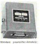
tor-quadrature rejector model 324 accepts 400-hz a-c input signals and converts them to phase-sensitive d-c signals for use in instrumentation systems. Maximum output is ±20 v d-c. Effective quadrature rejection ratio is 30:1 minimum. Input impedance is 10,000 ohms. Control Technology Co., 41-46 29th St., Long Island City, N.Y. **[386]**
