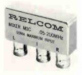
Double-balanced mixer M1C is for critical circuit functions of a-m with suppressed carrier, pcm, ppm, phase detection, and frequency converting in communications and test equipment. It has a noise figure of 5.5 db (ssb) at 50 Mhz, 45-db isolation between ports at 200 Mhz, and conversion loss of 5 db (ssb) at 50 Mhz. Relcom, 2329 Charleston Rd., Mountain View, Calif. [405]
