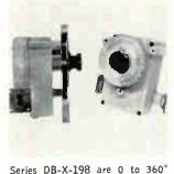
Series DB-X-198 are 0 to 360 direct-reading phase shifters for 7.05 to 90 Ghz. They offer accuracy to  $\pm 2.5^\circ$ , vswr of 1.20, and max. insertion loss of 1.25 db. All are panel mountable. Short insertion length (6 in. for X band) permits use in systems where compactness is important. DeMornay-Bonardi Division, Datapulse Inc., 1313 N. Lincoln Ave., Pasadena, Calif. **[407]**
