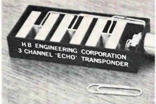
**Close quarters.** Their immunity to vibration enables several resonators to share a housing. The photo above shows a three-channel transponder for the echo system; at the left is a four-channel transponder for the passive remote telemetry system.
