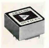
D-c differential operational amplifier model 1115 develops 5 ma output at  $\pm$ 10 v. Specifications include 15,000 open-loop d-c gain at full load, 20  $\mu$ v/°C max. voltage drift from  $-25^{\circ}$  to  $+85^{\circ}$ C, 200 na max. initial bias current drift, and 1.5 Mhz small-signal bandwidth. It measures  $\frac{1}{2} \times 1 \times 1$ in. Price is \$13 (\$9.75 in lots of 1,000). Analog Devices Inc., 221 5th St., Cambridge, Mass. [381]
