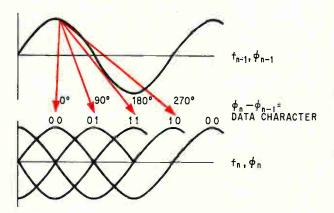
**Phase encoding.** Digital data is encoded by shifting successive tones by a multiple of 90°. For example, if  $f_{n-1}$  is one tone, the next higher tone  $f_n$  is shifted by 0° for 00, by 90° for 01, and so on.
