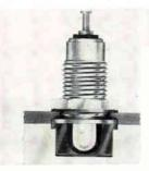
A lamp socket for mounting a T-1 size bayonet-base lamp in edge-lighted instrument panels has an over-all length of less than  $\frac{5}{16}$  in., plus mounting centers as close as  $\frac{3}{6}$  in. It positions the lamp for maximum lighting efficiency by providing 100% exposure of the lamp filament when installed in panels of  $\frac{5}{16}$  in. Western Indicator Co., 1710 N. Potrero, So. El Monte, Calif. [342]
