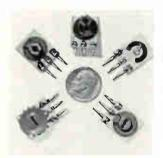
Trimmer resistor named Slim-Trim is useful in consumer, military and industrial equipment. Rated at ¼ w per section at 70°C, it has resistance values ranging from 100 ohms to 15 megohms. Maximum voltage is 350 v. The unit is built upon a base plate of alumina for heat dissipation. Centralab Electronics Div., Globe-Union Inc., 5757 N. Green Bay Ave., Milwaukee, Wis. [353]
