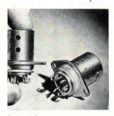
Series LS air-flow switches can withstand vibrations of 10 g to 500 hz and shock loadings up to 50 g at 11 msec. They are suited for use in military aircraft as preventive devices to protect aircooled mechanical and electronic equipment from overheating. The units are factory set to nominal air velocity from 200 to 1,000 fpm. G-V Controls Inc., Okner Parkway, Livingston, N.J. **[341]**
