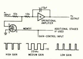
**Pulse control.** Signals for FET gain-changing circuit are provided by a pulse-width modulated source. High gain results from raising the on-off time ratio and low gain occurs when the ratio is reduced. Additional stages may be added to the gate of the FET.
