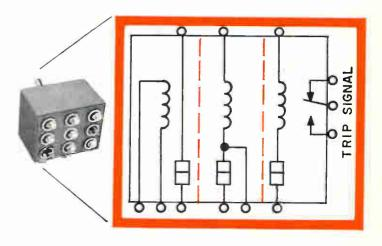
Style 50-APL is entirely magnetic trip (no heating elements), available 1, 2, 3, 4 and up to 10 poles, 10 ma to 50 amperes AC or DC, will open a 5000 ampere fault at 240 volts AC.
