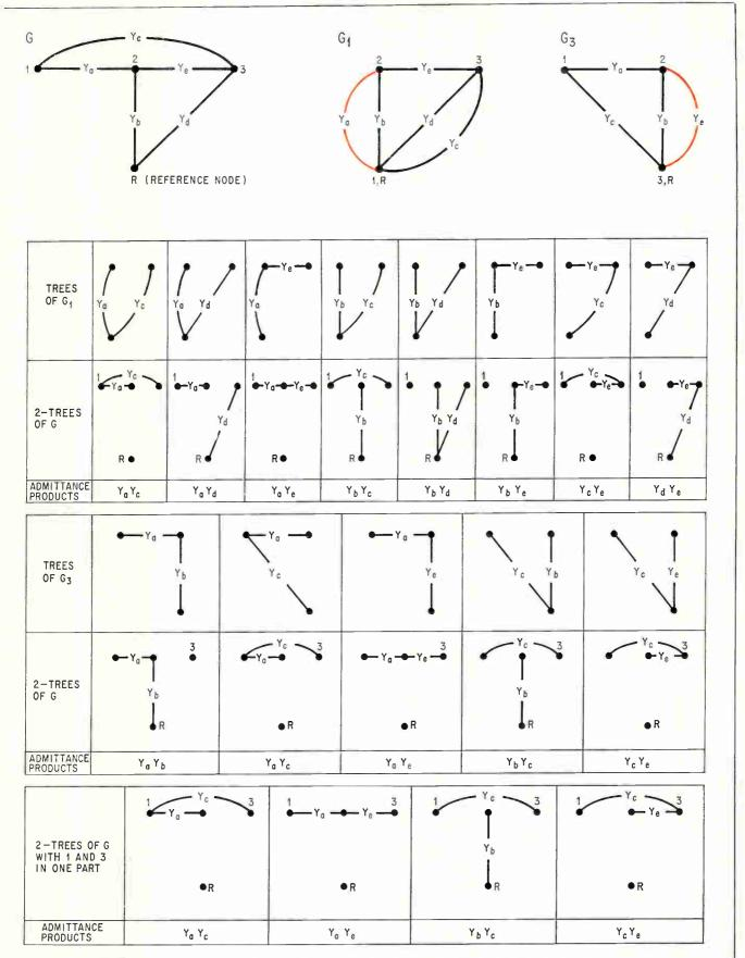
k-trees. Each branch of the network is replaced by a line segment that represents impedance of the branch. By shorting terminal 1 to the reference node the analyst can form all the 2-trees of  $\Delta_{11}$ . Similarly, shorting terminal 3 to R yields the 2-trees of  $\Delta_{33}$ . The 2-trees of  $\Delta_{13}$  are those common to both.
