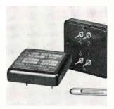
Miniature oscillators using IC's have frequencies as low as 1/10 hz in a case 11/2 in. square x 0.600 in. high, for p-c board mounting. Frequency accuracy is maintained from 0° to 65°C. Long-term accuracy is assured by a temperature compensated bimetallic tuning fork operating between 1,000 and 10,000 hz. Fork Standards Inc., 211 Main St., West Chicago, III. [344]
