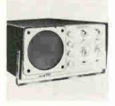
An X-Y monitor, Transi-Scope 701, uses solid state components and IC's. Specifications for the vertical and horizontal amplifiers include: deflection sensitivity of 10 kilohms, 1 kilohm, 100, 10 and 1 mv/major division with a vernier adjustment of X1 to X10 minimum; amplifier response of d-c to 1 Mhz (--3 db). Measurement Control Devices Inc., 2445 Emerald St., Philadelphia, Pa. [269]
