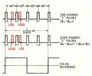
**Pulse decoding.** The phases of the output "Z" pulses correspond to the original data characters. The pulses, however, may be shifted from their undisturbed positions due to transmission delays. Shifts are in color.
