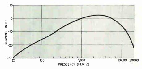
Impressive performance. Frequency response of new head is 10 kilohertz at -6db, with a playback speed of 3<sup>3</sup>/<sub>4</sub> inches per second. In addition, crosstalk rejection, which is even a more critical parameter in auto recorders than in home units, is greatly improved, to 80 db.
