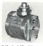
Unidirectional differential-pressure transducer PL385TC is capable of direct exposure to either gas or fluid corrosive pressure media on active or reference ports. Typical pressure ranges are from 0-5 to 0-50 psig. Differential overload is 5,000 psig. and max. allowable internal pressure is 6,000 psig. Price is \$500. Statham Instruments Inc., 12401 West Olympic Blvd., Los Angeles 90064. [362]
