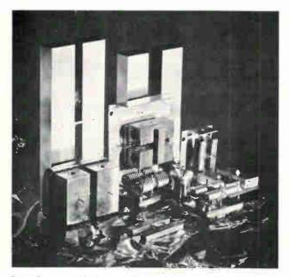
**On a theme.** Variations on the basic H-shaped design include big models that operate at very low frequencies, models fitted with tuning slugs, and a cylindrical version that can be used as a microphone.
