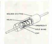
Metal film resistors in the MAF60 series are made by depositing a stable resistive film alloy on a ceramic substrate through a vacuum evaporation process. Units are rated at  $\frac{1}{4}$  w at 70°C and  $\frac{1}{6}$  w at 125°C. Change in resistance after 1,000 hours load life is less than  $\pm 0.5\%$ . Standard temperature coefficient is 100 ppm/ °C. Mallory Controls Co., 100 S Parker Ave., Indianapolis. [351]
