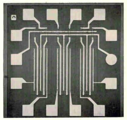
Getting its feet wet. Fairchild Semiconductor's move into the metaloxide semiconductor market begins with a six-channel multiplexer, the 3710. Soon the company plans to offer one new MOS product a month.
