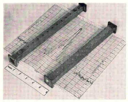
**Broad look**. Waveguides for Aeronutronic's new side-looking radar, developed for the Army, may be used by the space agency. Strip chart shows typical antenna spike pattern—decibles compared with radiated beam width.
