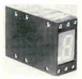
Decade counter model F1850E combines a bright segmented display with a 5-Mhz 1C counter. It requires only a single supply voltage of 5 v d-c. Input voltage swing is  $-1^{-1}$  v. Two outputs are provided to drive other counters. The unit is 7 a x 13/4 x 23/6 in, and weighs 2 oz, Price is \$90 in production quantities. United Computer Co., 930 W. 23d St., Tempe, Ariz. 85281. [388]
