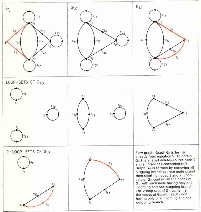
tionships. For example, equation 2 must be rewritten in the form of equation 3 to obtain a signalflow graph. The variables,  $x_1$ ,  $x_2$ ,  $x_n$  on the left-hand side of equation 3 may be interpreted as effects, and those on the right-hand side are causes.
