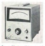
D-c multimeters MV-964A and MV-864A measure 100  $\mu$ v to 1 kv full scale, 0.1 ma through 1 amp full scale and 100 milliohms through 5,000 megohms. Both operate on 115/230 v, 50 hz through 450 hz and the 964A also operates on internal nickel cadmium batteries. Price: \$695 for the 964A, \$625 for the 864A. Millivac Instruments Inc., P.O. Box 997, Schenectady, N.Y. [365]
