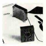
Transipad 10299-DAP adapts 12lead T0-5 IC's to a standard 0.100-in. grid pattern. It provides insulation and support, elevating the device only 0.150 in., including 0.025-in. feet under the Transipad. The feet permit air ventilation and open area for flushing away excess solder flux. DAP resists heat of 450°F. Milton Ross Co., 511 2nd St., Pike, Southampton, Pa. [352]
