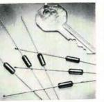
Hermetically sealed, glass-case silicon rectifiers series G have avalanche characteristics for protection from reverse voltage transients. Rated at 1 amp at 55°C, they have piv ratings from 200 to 1,000 v. Max. operating temperature is 175°C. Size is  $\frac{1}{16} \times \frac{1}{16} \times \frac{1}{$
