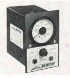
The ultraMonitor reads out any temperature point that can be sensed by a thermocouple. Used with standard thermocouples, the unit, with a  $5\frac{1}{2}$ -in. meter scale, is better than 2% accurate. It may be used with a thermocouple in parallel with other equipment because of its high input impedance that almost eliminates additional loading. Airborne Accessories Corp., Hillside, N.J. [363]
