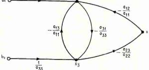
Superposition. Because more than one input is applied, the solution for  $x_2$  using signal-flow graphs requires superposition.
