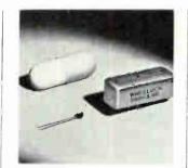
Reed relay series 442SS with built-in solid state driver occupies only 0.05 cu in. Typically, 40 2-pole relays with their driver stages can be mounted on a 4 $\frac{1}{2}$  x 5 $\frac{1}{2}$  in. p-c board with adequate spacing between "boards. Height is only 0.25 in. Contact is rated at a full 7 w. Units are available in 1-to 4-pole models. Wheelock signals Inc., 273 Branchport Ave., Long Branch, N.J. [1350]
