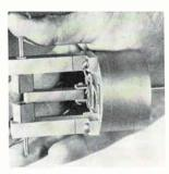
A d-c reciprocating motor consists of a copper-wound piston operating in an annular permanent air gap. The piston connects to a rotating shaft through a push rod and crank, and connects directly to an axial linear shaft. The motor is brushless, and commutated by an electronic circuit. Operating voltage is from 1.25 to 26 v. Mathews Electronics Corp., 312 S. Broad St., Mobile, Ala. [348]
