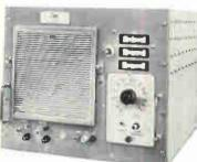
The NA Series of AC Power Supplies are exceptionally flexible sources of audio power. Each power supply consists of a Regulated Audio Power Amplifier with interchangeable fixed or variable Plug-In Oscillators for a wide range of precision AC power applications. The Amplifier has a full power range of 45-6,000 cycles. With the incorporation of a CML Plug-In Oscillator precise fixed or adjustable output frequencies are available anywhere within this range. For complete information, write today.
