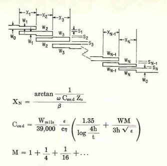
Multisection filter. In each section, coupling length  $X_{\rm N}$  depends on end capacitance  $C_{\rm end}$  for each conductor.
