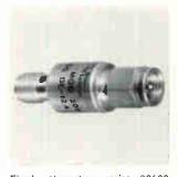
Fixed attenuators series 20600 operate from d-c to 12.4 Ghz. Standard models are available in values of 3, 6, 10, and 20 db with tolerances of  $\pm 5\%$  for attenuation values of 6 db or greater. All models are  $3/a \times 1^{3/4}$ in. Vswr is 1.20 max from d-c to 4 Ghz and 1.35 max from 4 to 12.4 Ghz. Price is \$80 each. Omni-Spectra Inc., Hallwood Ct., Farmington, Mich. [404]
