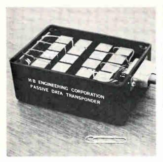
fined as the number of decade switches being read; a voice-grade line can handle 100 decades. The distribution of the decades in the communications circuit is immaterial—a single decade can be used at each of 100 meters (or any other telemetry transducer), or five can be used at each of 20 remote sites. Capacity of the interrogation system can be raised to 1,000 decades if the link's bandwidth is raised from 3 khz to 8 khz.
