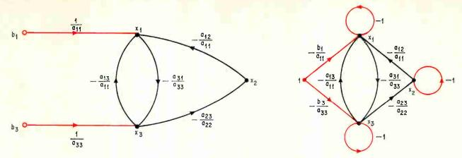
**Graph transformation.** Graph  $G_1$ , right, is formed from  $G_m$ , left, by first adding a self-loop with a gain of -1 to each branch devoid of a self-loop. Then the gain of the branch at source nodes 1 and 3 are multiplied by  $\cdot b_1$  and  $\cdot b_3$  respectively. These are then combined into one source node, labeled 1.
