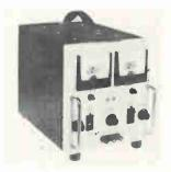
Portable, solid state power converter 4000A is designed for mobile use; the 4000AP is suited for ground service and lab use; the 4000AR, for rack or panel mounting. Input requirements are 120 v a-c, 47-450 hz. Output signals are fixed at 400 hz at 1 kva, or varied from 100-130 v a-c and 360-400 hz at outputs to 1 kva. Power Systems Inc., 4023 Del Ray Ave., Venice, Calif. [1376]
