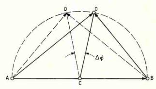
Vectors. Voltage that is proportional to the source-drain resistance of the FET is represented by vector DB. Output of network is a vector that is constant in amplitude and represented by CD.
