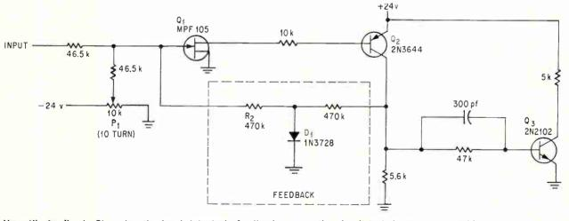
Versatile feedback. Changing the level detector's feedback causes the circuit to behave as an astable, mcnostable, bistable, or gated oscillator because Q<sub>1</sub>'s gate has a high input impedance, allowing signals to be summed at that point.
