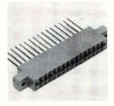
Card-edge receptacle series 6021 has 30 dual-readout or 15 singlereadout wire-wrap contacts spaced on 0.156-in. centers. It accommodates a 1/16-in. p-c card. The unit is available with simple-cantilever or double-cantilever bifurcated-nose contacts, both rated at 5 amps and made of phosphor bronze with a gold flash over a nickel underplate. Elco Corp., Willow Grove, Pa. 19090. L346J
