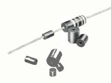
Ceramag<sup>®</sup> ferrite beads offer a simple, inexpensive, yet effective means of obtaining RF decoupling, shielding, and parasitic suppression without sacrificing low frequency power or signal level.
