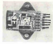
Looking down. Top view of regulator circuit showing hybrid IC configuration.
