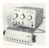
Solid state uhf sweep generator model 1501 features completely automatic frequency tuning and r-f attenuation. An electronic attenuator provides a 30-db dynamic range of r-f output level, and the tuner i-f or tv receiver 2nd detector demodulated curve is maintained at a constant amplitude over this range. Basic unit price is \$425. Sweep Systems Inc., P.O. Box 616, Indianapolis. [373]
