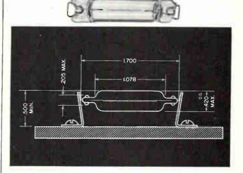
Automobile dome lamps have long employed the cartridge lamp shown at the top. It was a good lamp but it was bulky and had cemented-on end caps for contacts. Also the fuseclip type mount was comparatively expensive to make.
