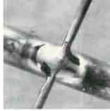
Cross weld between 0.005-in. diameter tungsten and 0.020-in. diameter nickel wires.
