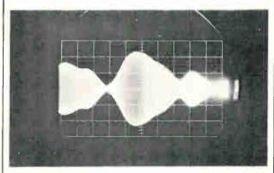
Fading envelope. Large and rapid amplitude changes are characteristic of continuous-wave signals.
