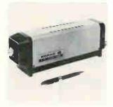
Yttrium aluminum garnet laser K-Y1 has a c-w output of 3 w. Emission is at 1.06 microns with a half-angle beam divergence of 2.5 milliradians at threshold. Power supply is housed in a  $10 \times 10 \times 20$  in. cabinet. The laser head is  $4 \times 4 \times 12$  in. Applications include trimming of resistors, real-time data display. Korad Corp., 2520 Colorado Ave., Santa Monica, Calif. [385]
