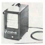
Environmental monitor model 166 uses a dry-writing method for a continuous, permanent record of temperature across  $-50^{\circ}$  to  $+100^{\circ}$ C range, with an accuracy of  $\pm 1.5^{\circ}$  C. The chart speed of 1 in/hr provides a 31-day record with standard 63-ft, style B, 75division paper. The unit measures  $5\frac{1}{2}$  x  $3\frac{5}{6}$  x 576 in. Rustrak Instrument Co., Municipal Airport, Manchester, N.H. [368]
