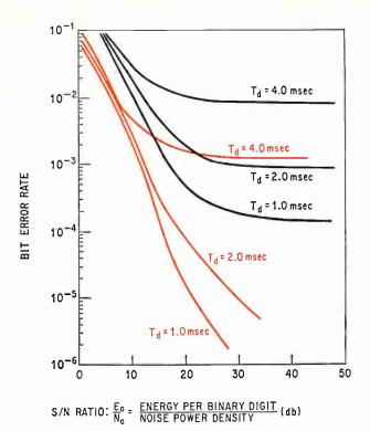
Simulated results. The error rate at 4,800 bits per second and at 2,400 bps with inband frequency diversity (in color) decreases with improved signal-to-noise ratio, but levels off and is limited by multipath delay spread,  $T_a$ . Ionosphere effects were simulated in laboratory.
