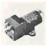
Miniature pressure transducer series P2-5000 combines a precision variable reluctance, twisted Bourdon tube pressure sensor with an integral carrier-demodulator. The series includes models for measurement of gauge, differential, and absolute pressure in ranges from 0-1 to 0-5,000 psi, with ±0.50% accuracy. Whittaker Corp., 12838 Saticoy St., N. Hollywood, Calif. 91605. [372]
