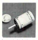
Incremental, photoelectric rotary encoder 8610 is housed in a synchro size 11 package. It is suited for use in computer and process control equipment, and aerospace guidance systems. The unit incorporates GaAs light sources for maximum reliability from  $-55^{\circ}$  to  $+100^{\circ}$ C and shock in excess of 50 g. Accuracy is  $\pm 1$ minute. W.&L.E. Gurley, Troy, N.Y. 12181. [382]
