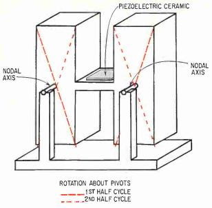
**Push-pull.** As the piezoelectric input transducer contracts and expands, the web flexes and the bars oscillate in opposing directions. The resonance signal can be picked off by a coil near a bar or by another piezoelectric transducer underneath the web.
