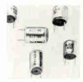
Miniature capacitors type V170 are constructed by wrapping the film dielectric with a synthetic film and thermally sealing the end. They may be subjected to 100% relative humidity for 72 hours at 75°C and suffer not more 1/3 loss in insulation after exposure and subsequent drying. Capacitances range from 0.01 to 0.1  $\mu$ f. Aerovox Corp., New Bedford, Mass. [356]
