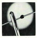
Microminiature zener diodes are electrically interchangeable with standard Jedec types. Measuring 0.075 in. in diameter and 0.125 in. long, the MTC series are encapsulated in high-temperature epoxy. Standard units cover the voltage range of 5 to 12 v. They have either silver leads or gold plated, weld ribbon type. Computer Diode Corp., Pollitt Dr. South, Fair Lawn, N.J. [440]
