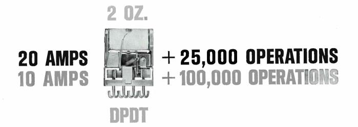
The rugged Hi-G "T" Series of 10 amp. crystal can relays meet all applicable requirements of Mil-R-5757. Testing has proved more than 25,000 operations typical at 20 amps. They match or out-spec. other 10 amp. DPDT crystal can relays and are priced competitively or lower. Case size:  $1.234'' \times 1.025'' \times .515''$ . All standard configurations and header styles are available for fast delivery.
