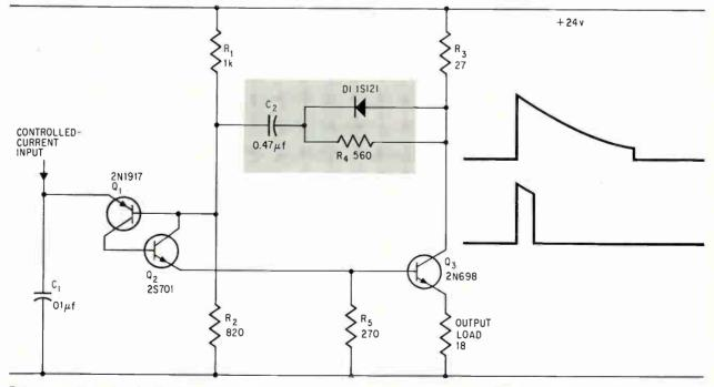
**Pulse generator.** Feedback network between pulse-circuit output and avalanche-switching input, formed by  $Q_1$  and  $Q_2$ , permits trailing edge of output pulse to be shaped. Exponential decay in the trailing edge of pulse output is unwanted. With a sharp decay the trailing edge triggers or controls other circuits.
