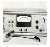
Electrostatic voltmeter model 144 Isoprobe uses a noncontacting 1½ x 1¼ x 2¼6-in. probe to permit drift-free measurement with 0.1% accuracy. Range of  $\pm$ 1 to  $\pm$ 2,000 v full scale at greater than 10<sup>18</sup> ohms input impedance allows for many potential applications in general materials research and evaluation. Monroe Electronics Inc., 5 Vernon St., Middleport, N.Y. [361]
