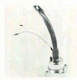
Thyristors in the CR7K series offer surge ratings of 7,000 amps and rms current of 770 amps from a pair in inverse parallel. These cells will replace ignitrons as the SCR is smaller and can be mounted in any position. Arc volt drop and triggering time are reduced by a factor of 20, and power requirement of the gate is 5 w peak. Calvert Electronics International Inc., 220 E. 23d St., N.Y. **[438]**
