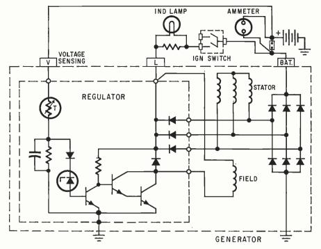
New look. As the voltage of the zener diode increases, the input transistor saturates. This turns off the Darlington pair and the generator field current. As generator output dips, the zener turns off and full current is applied to generator field coil.
