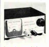
Zener reference, regulated power supply model PZ-131 delivers stable, continuously variable outputs from 0.5 to 25 v at currents to 200 ma. The compact  $(41/2 \times 2)/2 \times 4$  in.) unit provides load regulation better than 100 nv, line regulation of  $\pm 30$  mv, and a-c ripple and noise of less than 2 mv at full load. Price is \$34.95. Viking of Minneapolis Inc., P.0. Box 9507, Minneapolis. I **387**]
