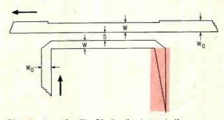
Directional coupler. The 50-ohm line tapers to the proper width for the corresponding coupled-mode characteristic impedance.
