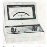
Power factor meter model 83 measures input frequencies ranging from 50 to 2,500 hz. It has an accuracy rating of ±1% of total span with sine-wave inputs of 120 v and currents ranging from 1 to 5 amps. The meter is self-energized from the voltage input and produces direct readings for leads or lags of up to 90°. Weston Instruments Inc., 614 Frelinghuysen Ave., Newark, N.J. [366]
