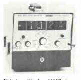
Digital multimeter 8000B is a portable instrument that uses Ni-Cd batteries. It offers 3 ranges of d-c volts, 3 of a-c volts and 5 of resistance. Features include full 4-digit readout, with 10% 5th-digit over-ranging. Accuracy is ±0.05% and resolution is 0.01%. Input impedance on all ranges is 10 megohms. California Instruments Corp., 3511 Midway Dr., San Diego, Calif. [374]
