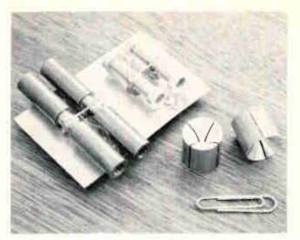
Tuning slugs. Applications versatility is indicated by the pair of resonators on the board at the left. Device with large tuning sleeves resonates at 300 hz, the lower end of the voice band. An identical device, but with small tuning collars, operates at 3,000 hz, the upper end of the band. Cylindrical objects are acoustic resonators; transducers haven't yet been placed on their webs.
