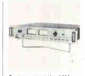
Frequency comparator 103A can make relative frequency comparisons, relative phase measurements, and short-term stability measurements without peripheral equipment. It makes short-term frequency comparisons to 1 part in 10<sup>11</sup>. Test and reference frequencies of 100 khz to 5 Mhz in 14 discrete increments are accepted. Montronics Inc., P.O. Box 7428, Seattle, Wash. [371]
