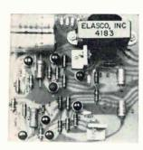
Dual output power supply model 2Q15-250PC operates from 105-125 v a-c, 60 to 400 hz, and furnishes ±15 v d-c with 250 ma capability from each side. Line and load regulation is held to 0.1% maximum with ripple and noise held to 2 mv rms max. Price (1-9) is \$47 each. Delivery takes less than 2 weeks. Elascoteastern Inc., 5 Northwood Rd., Bloomfield, Conn. 06002 [385]
