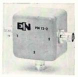
Power multicoupler model PM12-2 is a two-way hybrid coupler covering the range of 250 khz to 110 Mhz. Unit is capable of handling up to 12 w of average r-f power at  $\pm 65^{\circ}\mathrm{C}$  ambient temperature Maximum insertion loss is 0.4 db; amplitude balance, 0.1 db, phase balance,  $\pm 1^{\circ}$ ; vswr, 1.1:2 maximum. Electronic Navigation Industries Inc., 1337 Main St. East, Rochester, N.Y. [384]
