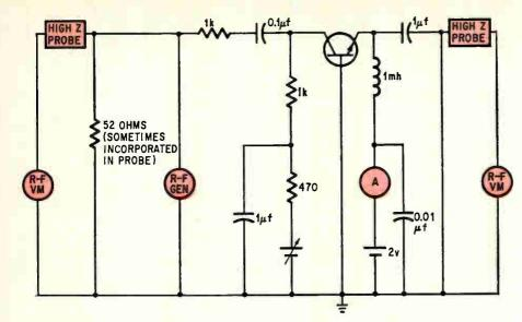
Measuring  $f_{htbI}$ . Inverse alpha cutoff,  $f_{htbI}$ , is obtained by providing a constant r-f signal at the collector and increasing its frequency until the output signal at the emitter drops by 3 db.
