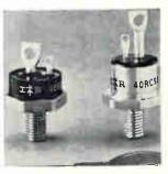
Silicon controlled rectifiers series 40RCS are new 40 amp devices available in two versions: epoxy package, up to and including 600 v rated units; and glass-to-metal sealed units rated from 700 v through 1200 v. Applications include d-c motor controls, power supplies, heater controls, and airborne and mobile converters. International Rectifier, 233 Kansas St., El Segundo, Calif. [439]
