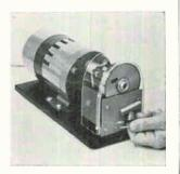
Motorized coaxial cable stripper model CX-2's operation consists of inserting the end of a co-ax cable into the rotating cable holder, and turning a handle which engages the 3 cutters to cut the insulation and shielding. Upon removal, end of cable is prepared with a 3-step strip for appropriate connector. Western Electronic Products Co., San Clemente, Calif. [427]
