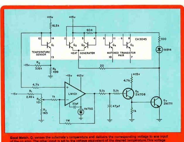
of the op amp. The other input is set to the voltage equivalent of the desired remperature. This voltage difference drives the current regulator, Q<sub>2</sub>Q<sub>2</sub> which neats the chip to hold its temperature constant.
