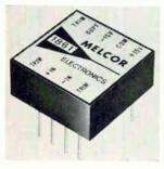
Amplifier model 1861 features a FET input stage combined with an IC. All shaping networks are Internal, with no extras required except a zeroing potentiometer, if desired. Other features include an output of  $\pm 10~v~\pm 5$  ma minimum, minimum d-c gain of 15,000, and unity gain bandwidth of 1 Mhz. Price (1-24) is \$10. Melcor Electronics Corp., Farmingdale, N.Y. [381]
