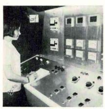
Plantation punch. Like an atom-smasher, Thomson-CSF's new machine accelerates particles for bombardment of a target, in this case semiconductor wafers. Simple controls allow in-plant use.
