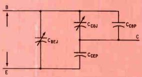
Base-emitter capacitance measured with collector-base not shorted.
