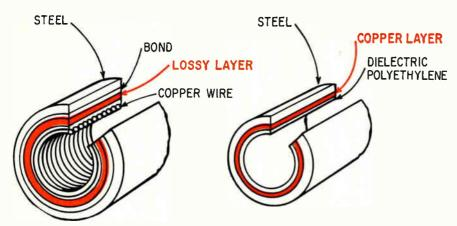
Double indemnity. Two types of waveguide sections can be used to kill unwanted modes. The helix-wound version at the left traps those modes in its circular configuration, prohibiting movement down the waveguide. The dielectric-lined section converts signals into heat, which is then dissipated in the walls of the pipe.
