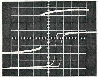
Enhanced. Top figure, hysteresis trace of bulk TT1-390 at a 400-oersted drive field shows a remanence ratio,  $M_{\rm r}/M_{\rm s}$ , of 0.67. The trace of the deposited film (bottom figure) made with same material has enhanced ratio of 0.82. Lower traces in each figure, expanded 500 times, show the deposited film with a squarer loop than the bulk material.
