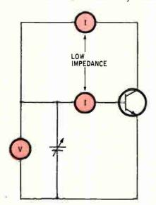
D-c measurements. Two low-impedance current meters are used to measure current gain under normal circuit operation. Meters short the base and collector, and assure accurate readings.
