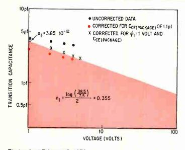
Evaluating a<sub>1</sub> and n<sub>1</sub>. Emitter-base parameters for the transition capacitance are obtained from a plot of transition capacitance versus base-emitter voltage.
