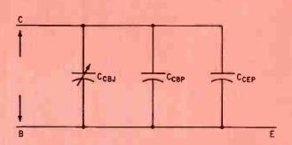
Collector-base capacitance measured with emitter-base shorted.
