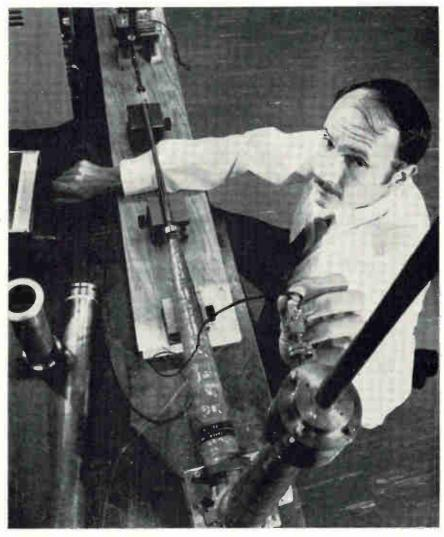
Guiding hand. Signals will travel from repeater to repeater down a two-inch waveguide in Bell's millimeter-wave system. To obtain the low-loss circular electric mode of transmission, a transducer length of pipe, which forms that mode, connects generator and line.
