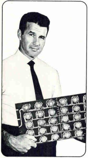
using rotary switches requires 330 soldered joints . . . over 8 hours of labor . . . occupies 293 square inches of panel space . . . costs \$88.00 installed. (That's \$0.29 per switching point.)
