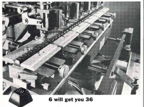
Now, new 6-spindle New Hermes engraves up to 36 machine keys with one set-up.
