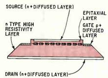
Pyramid. Thick intrinsic layer between gate, drain gives high power rating.
