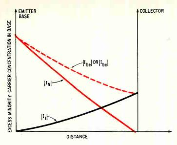
Concentration. Currents are proportional to the slope or gradient of the concentration lines for this npn transistor. Uniform base-doping is assumed and high injection effects are ignored. Current,  $I_N$  is proportional to slope of colored line at collector-base junction.  $I_I$  is proportional to slope of black line at emitter-base junction;  $I_{be}$  is proportional to slope of dashed line at emitter-base junction;  $I_{be}$  is proportional to slope of dashed at collector-base junction.
