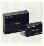
Low-pass active filters are designed for Butterworth response. Model 5720 is the 2-pole version at \$25 each. Cutoff frequency range is 10 hz to 20 khz. Model 5721 is the 4-pole version with a frequency range of 1 hz to 20 khz and a price of \$45. Both units have an output impedance of less than 20 ohms. Burr-Brown Research Corp., Int'l Airport Industrial Park, Tucson [386]
