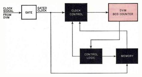
Three functions. Basic actions of digital reference-temperature simulator (dark boxes) coordinate with clock signals and functions (colored boxes) in digital voltmeter.
