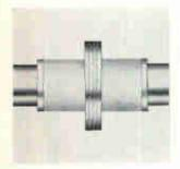
Back-to-back varactors DEP1712-1726 are for electronic tuning. They come with nominal capitance values from 1.2 pf through 12 pf, with Q's of over 1500 measured at 50 Mhz. In the back-to-back configuration, one bias voltage supply, either a-c or d-c, is applied to the common flange contact with other contacts on ground. MSi Electronics Inc., 57th St., Woodside, N.Y. [440]
