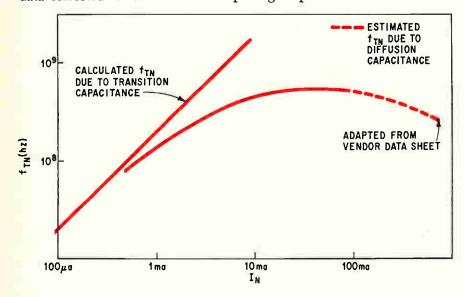
Finding  $f_{TN}$ . Transition capacitance resulting in a low value for measured  $f_{TN}$  at low currents.
