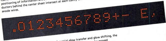
By utilizing the phenomena of preferential glow transfer and glow shifting, the initial glow caused by cathode ionization in the dot matrix may be moved through selected holes to a visible position on the top surface. A sequential flow of light is thus achieved without separate drivers for individual columns and rows.
