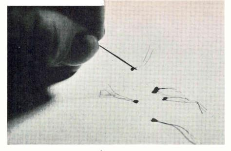
Inductors. Single and multiple microinductors, whose values range between 70 and 90 microhenrys, are encapsulated by nickel-zinc ferrite. They can be used as hybrid insertion pieces in circuits where space is at a premium.
