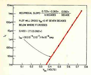
Current values. To find the emittersaturation current les, collector current le first is plotted against emitter base voltage V<sub>be</sub> on semilog paper. Final process is detailed on graph.
