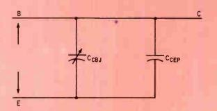
Base-emitter capacitance measured with collector-base shorted.
