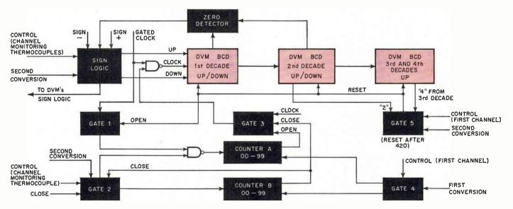
case correction requires counting down  $T_a$  bits from  $-(T_n - T_a)$ .
