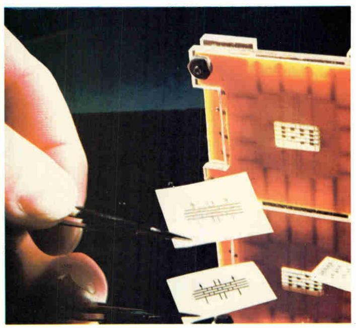
Long memory. The 16-bit read-only memory, mounted in a test board, has a flexible clad-fiberglass etched to form drive lines, one set on a side, which have areas of coincidence corresponding to the bit pattern. The assembled drives have a 30-nanosecond readout capability. Future devices could use low-cost ceramic substrates with increased bit densities.
