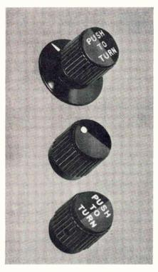
Pushed in, these Raytheon self-locking mechanisms can rotate control shafts in either direction to precise settings. Released, they automatically lock the shaft against vibration, shock, accidental turning. Their simplified, rugged packaging complies with MS91528C and MIL-K-3926B.
