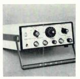
Minature waveform generator model 123 features voltage controlled frequency over a 1,000:1 ratio and a bandwidth from 0.1 hz to 3 Mhz. It produces sine, square and triangle wave forms, as well as a sync pulse. Output voltage for all waveforms is at least 20 v p-p into an open circuit or 10 v p-p into a 50-ohm load. Price is \$345. Exact Electronics Inc., Hillsboro, Ore. [364]
