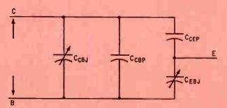
Collector-base capacitance measured with emitter-base not shorted.
