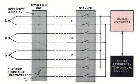
Bits replace summing. In new digital technique for thermocouple reference-junction correction (left), temperature of isothermal box, stored as bits in simulator is added to thermocouple's temperature, stored in digital voltmeter. Analog compensation methods (at the right) involves the summing of millivolts representing reference and thermocouple signals.
