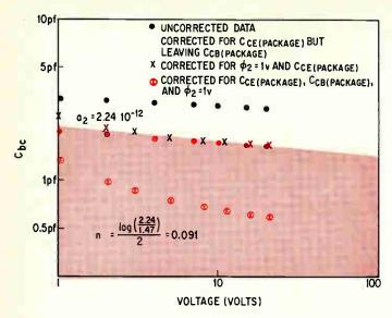
Finding  $f_{\rm TN}$ . Transition capacitance parameters for the capacitance are obtained from a plot of  $C_{\rm bc}$  versus collector-base voltage.
