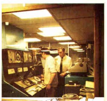
**Do-it-yourself kit.** In case QE2 must dock without the aid of tugboats, two fiberglass communications consoles and a gyro repeater help ship's officers to keep the dock in view while maintaining contact with the ship's personnel.
