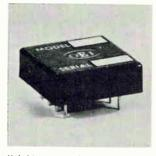
Hybrid operational amplifier model 9706 comes in an 8-lead jumbo dual in-line package measuring 0.32 in. high and 1 in. square. It features 60 db typical open loop voltage gain; ±360 v/μsec typical slewing rate; 1,300 Mhz typical gain bandwidth product; and 10,000 megohm input impedance. Price (1-2) is \$54 each. Optical Electronics Inc., P.O. Box 11140, Tucson 85706 E3881
