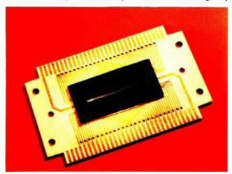
**Crowded picture.** Monolithic arrays are in demand for OCR: 100 phototransistors fit on Motorola chip bonded to a ceramic substrate.
