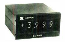
are display blanking, autopolarity, remote hold command, read rate control, overload and plus-minus indicators, and true differential inputs. Accuracy of 0.05% is maintained with digitizing rates of 0 to 60 readings per second. Price is \$189. Newport Laboratories Inc., East Young St., Santa Ana, Calif. [383]
