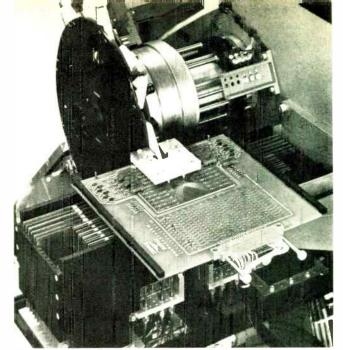
**5. Sorting it out.** A tough problem in production-line IC testing is to interface an automatic handler with a nanosecond system while preserving signal integrity. One solution was to use a carefully designed interface to the Daymarc 852 "stick-to-stick" sorter.
