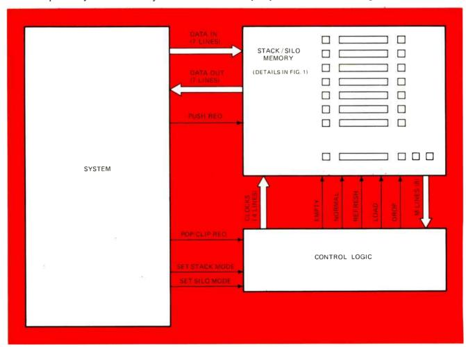
3. **Relation to system.** The stack/silo memory of Fig. 1 can be used in any small or large digital system. It is almost completely independent of the system, because it requires only data lines in both directions, a "push request" signal to initiate loading a new word, and a few signals to the control logic. The memory runs with its own clock, and therefore is asynchronous to the system in which it is installed.
