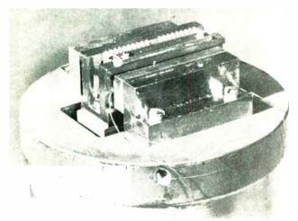
**News flash.** Ytterbium- and neodymium-doped YAG lasers have communications potential. TI's Yb-YAG laser is in cooling tank.
