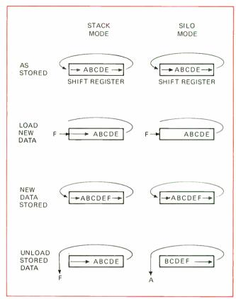
**5. Actual operation.** When dynamic shift registers are organized as stack or silo memories, new data always goes in front of old data circulating through the registers. Old data is "clipped" off the rear of the data in silo mooe, "popped" off the front in stack mode.
