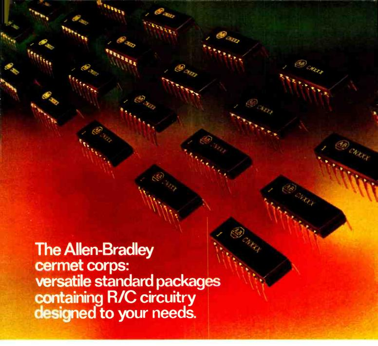
The need: compact R/C networks in DIP's for terminator applications in new generation computer designs. To meet the circuit board space crunch, Allen-Bradley combines resistors and capacitors in a package compatible with automatic insertion equipment. These cermet networks save space and attachment costs. Packaged in dual in-line molded packs that lock out the environment and
