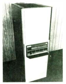
model 16 has a comprehensive set of 114 instructions, and the core memory is directly addressable and alterable to the eight-bit level. The instruction set includes fixed-point arithmetic, logical, byte handling, status control. Single unit price of the 16 is \$14,700. Interdata Inc., 2 Crescent Pl., Oceanport, N.J. 07757 [365]
