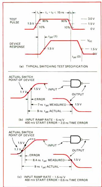
2. Be more exact. Conventional pulse test specifications may be ambiguous about pulse timing (a). Two pulses, each with a rise time of less than 15 nanoseconds, can result in a 1.4-ns variation in errors in propagation-delay tests (b and c). A specific, fast ramp rate reduces error and makes the test reproducible.
