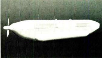
Garrett AiResearch enclosures are also cooling the pod mounted ALQ-76 and ALQ-99 electronic countermeasures systems. The enclosure in the ALQ-99 pod (shown above) for the EA-6B utilizes surface heat exchangers as the ultimate heat sink.
