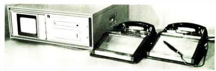
**Genuine.** Signature verification gear has stainless steel pad, stylus. Analog circuits pick up signature, transmit it to verification center's display tube. There, it is held for 30 minutes while a clerk checks it for accuracy. System comes in two configurations: one for hard-wired intercom, the other for phone link.
