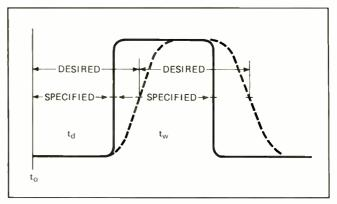
**4. Pulse-generator errors.** Specifications of pulse generators typically give the delay  $t_{\rm d}$  at minimum rise time, which may be 1 ns. When a longer rise time is desired, the delay is unknown. Error can be avoided by having the test system calibrate the pulse.
