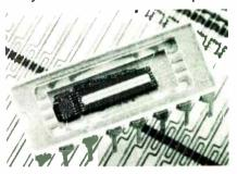
diodes of the monolithic imagesensing device are spaced on 1-mil centers, with on-chip scanning circuitry for serial output on a single video line. TTL compatibility is achieved through drive circuitry provided in the same 16-lead DIP. The silicon gate sensors are operated in the charge storage mode providing high sensitivity at up to 10-MHz scan rates. Price is \$250 in OEM quantities. Reticon Corp., 365 Middlefield Rd., Mountain View, Calif. 94040 [417]
