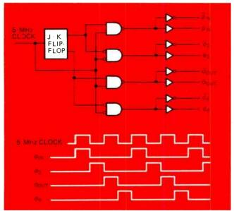
2. Clock pulse generator. A single 5-MHz oscillator plus one J-K flip-flop and four gates can generate all the timing pulses needed by the stack-silo memory of Fig. 1 and its associated control logic. Amplitiers are necessary to provide sufficient power.
