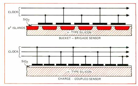
**Call the bucket brigade.** Salient difference between bucket-brigade and charge-coupled devices: bucket brigade requires two diffusions per bit processed; CCD requires none.
