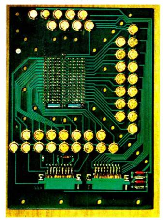
**Growing up.** Discrete detector arrays are becoming more complex. Motorola unit has hermetic photodetectors, decoding hybrids,
