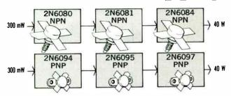
Marine radio power chain. 152 to 162 MHz, 12.5 V. Send for data sheets and AN282: "Systemizing RF Power Amplifier Design" and AN495: "A 25 W, 175 MHz Transmitter for 12.5 V Operation."
