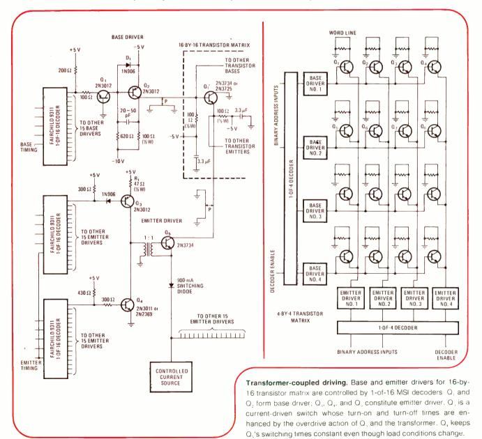
rent and pulse conditions. But since the voltage excursions of  $Q_5$ 's collector and emitter could vary over a wide range, a transformer-coupled drive is used to correct for changing load conditions.
