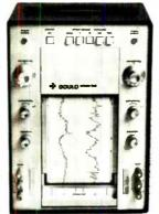
of 1 millivolt per chart division to 500 volts full scale. And a choice of 20 signal conditioners give you an even wider range. Four chart speeds are push-button controlled. And two event markers are standard.
