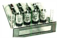
plays do not appear blurred. The modules operate from a single 5-v source, are available with three to six digits complete with TTL-compatible latches, driver-decoders, and decimal point at each position. Price is \$20 per digit. Tronix Inc., Box 349, Phillipsburg, N.J. [384]
