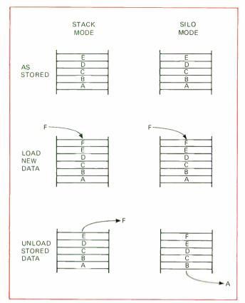
**4. Functional appearance.** To the system, the stack and silo versions look like these representations. New data always goes in at the top. Old data is unloaded from top in stack mode (first-in, last-out) and from bottom in silo mode (first-in, last-out).
