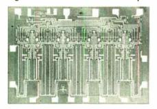
by Ragen Semiconductor contributes what the company calls "extremely low distortion" over a full 8-volt signal range. Distortion into a 10,000-ohm load (at 4 v rms and 1 kilohertz) is less than 0.05%—"So low we had difficulty measuring it," says Albert Medwin, Ragen Semiconductor president.
