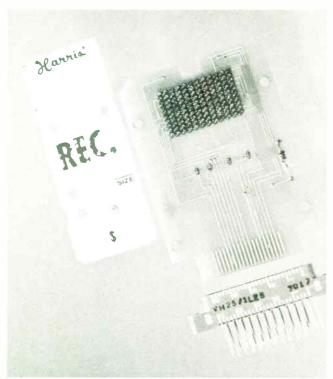
In small packages. Fairchild's circuit squeezes 120 transistors into a 50-by-100-by-80-mil package for reading of tags shown at left.
