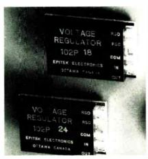
W. Specifications include regulation of 20 mv for load current of 0 to 1.5 A; 10 mv per volt input change, and temperature coefficient of 0.01%/ C. Epitek Electronics Ltd., 19 Grenfell Cres., Ottawa 12. Ontario, Canada [385]
