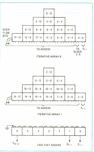
**5. Divided for speed.** Separating the iterative array into two or more parts and then adding the results produced by the parts decreases the propagation time even more—in this case to 185 ns.
