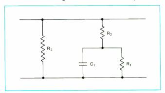
**1. General load.** RC network accurately represents most loaded transmission lines in high-speed digital systems. When  $R_2=\infty$ , it is resistive; when  $R_1=\infty$ ,  $R_2=0$  and  $R_3=\infty$ , it is capacitive.
