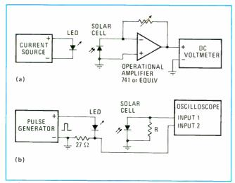
2. Simplicity. Uncomplicated setups simplify measurement of data required to derive curves of Fig. 1. At lower current levels, dc measurement with arrangement (A) should be used. When current level through LED exceeds 5 mA, pulsed setup of B) is required.
