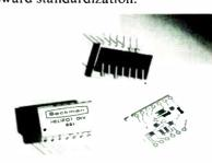
Now, the Microcircuit Operations at Beckman Instruments Inc. is taking what it calls a further step in that direction with its model 881 state-variable active filter. It's a hybrid thick film device instead of discrete components in a potted module, and it's more flexible than previous devices, says George Smith, director of research and development.
