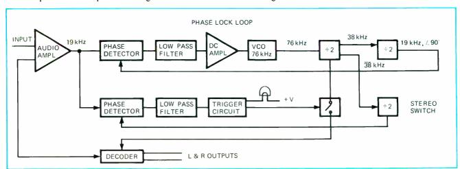
1. Stereo demodulator. Three functions—a phase-lock regeneration loop, a stereo switch, and a decoder section—are combined in a single integrated circuit to form a complete fm stereo demodulation system. A regenerated pilot tone, which is obtained from the phase-lock loop, is modulated with the composite input in the switch section to determine whether the input signal is in stereo or is monaural.
