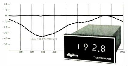
Digilin's linearizing readout breaks up your non-linear sensor information into ten straight-line segments that approximate the most capricious curve with all the accuracy you need for just about any transducer.
