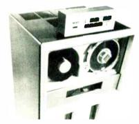
second at 200 in/s, and rewind speed is 2,400 feet of tape in 45 seconds. The model CDs 340 includes electrically operated reel/hubs, reel servo control by means of vacuum switch sensing, and in-column rewind under capstan control. Delivery time is 30 days.
