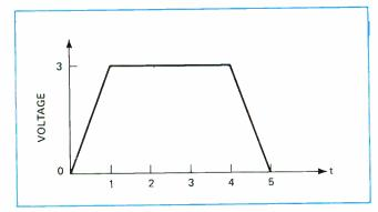
**3. Input voltage.** Line accepts input waveforms as piecewise linear functions with up to 20 breakpoints. For example, the voltage waveform shown is described by an initial value (0,0) and four breakpoints with coordinate locations of (1,3), (4,3), (5,0), and (10,0).
