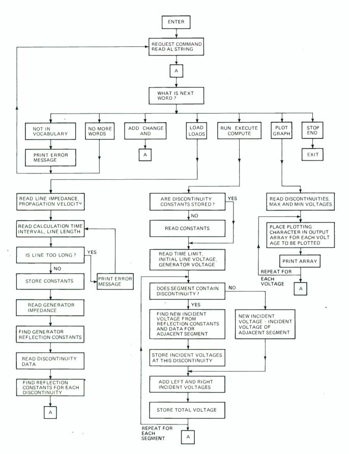
2. Flow chart. Once initial data is entered, Line computes incident voltage and reflection constants for each line segment, storing only incident and transmitted voltages from previous adjacent segment. There are three basic instructions: LOAD (describing physical line properties), RUN (establishing initial electrical conditions), and PLOT (graphing reflection voltage at several load points).
