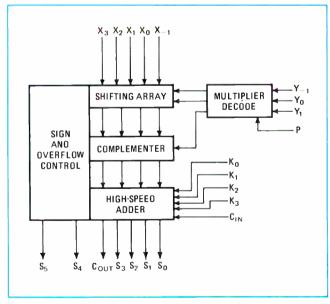
1. Multiplier. These five sections multiply a four-bit number, x, by a two-bit number, y, and add another four-bit number, k, to the product. Inputs x., and y., are among connections used when several devices multiply longer numbers. Pin P determines logic convention; it's grounded for positive logic, unconnected for negative logic.
