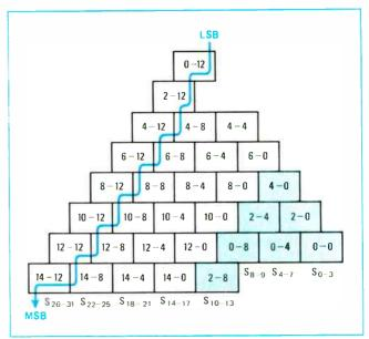
**4. Faster array.** Moving the tinted blocks down from their location in Fig. 3 without changing their horizontal position relative to each other decreases longest propagation path from 335 ns to 290.
