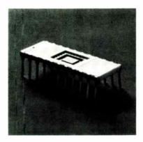
The AMS 6002 MOS RAM has already established more than 16 million hours of field performance in more than 40 installations. Six months after its introduction, the 6002 is still the fastest 1024-bit RAM available with 150 nanosecond access and 250 nanosecond cycle times. It is the only MOS RAM that utilizes field-proven P-channel processing and a ceramic package.
