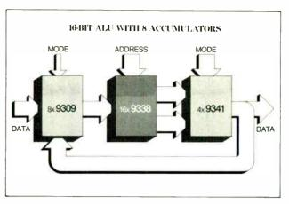
Used as a one-bit slice of eight registers/ accumulators, it combines with either the 9340 or 9341/74181 ALU device to become the powerful heart of a minicomputer central processing unit. It's equivalent to a 9301 decoder, a 9308 latch, two 9312 multiplexers and a dual flip-flop. Send for our Appl. Note 220.
