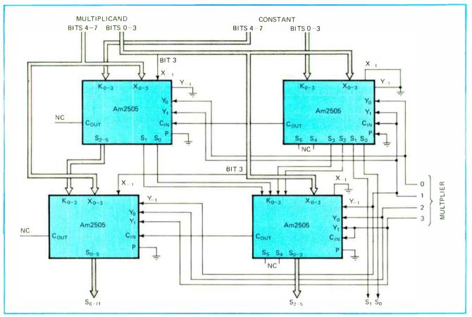
**2. Iterative connection.** Four multipliers can produce a 12-bit product from eight-bit and four-bit inputs. Successive rows are staggered; four K inputs to multiplier at lower right are connected to S outputs of multiplier immediately above and of multiplier at top left.
