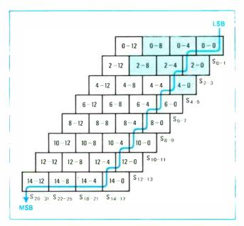
**3. Larger array.** For longer words, iterative connection can be extended indefinitely. Block labels identify bits connected to that block; for example, 6-12 refers to multiplier bits  $y_6$  and  $y_7$ , and multiplicand bits  $x_{12}$  through  $x_{13}$ . Solid color line shows path of longest delay through this array; tinted multipliers are the ones rearranged in Fig. 4 to reduce this propagation time.
