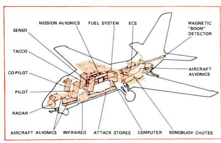
**Big avionics package.** That's the Navy's S-3A, which Lockheed sees as a way to save face after the L-1011 and C-5A problems. The antisub craft will begin flight testing next July.
