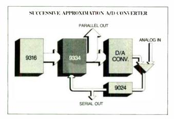
In an A/D Converter, the 9334, combined with a 9316 Binary Counter and standard linear devices, provides a successive approximation analog-to-digital conversion, Send for our Appl. Note 294.
