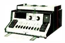
switches into a random-access memory, making it possible to set up and check an entire word before programing. Address capacity is 4,096 words, expandable to 65,536 words. Price for the basic model is \$1,500, and adapters start at \$360. The model 500 is modular in design, with plug-in circuit boards used throughout to facilitate service and minimize downtime.
