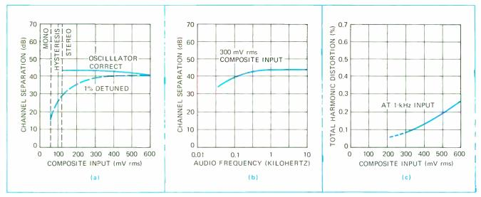
Choice characteristics. Because of the oscillator's excellent temperature stability, overall channel separation remains good even during detuning (a). When the oscillator is correctly tuned, channel separation is impressively high over the frequency range (b), and the circuit's total harmonic distortion characteristics stay at a very low level right through the range of the input signal (c).
