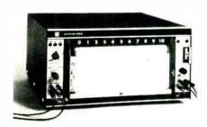
and fault location. Its step pulse rise time is 1.3 nanoseconds, amplitude 1 volt. The 1501 can be used out to 10,000 feet. Price is \$1,900 for the reflectometer alone, and \$2,950 with the 323 oscilloscope.
