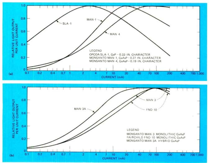
1. Helpful data. These curves, plotted from measurements made on several commercially available types of seven-segment displays, are the first step in determining the factor S, a comparative measure of the gain or loss obtained under multiplexed operation. Ratio of values at specified peak current to those at specified average current yields S. Similar curves can be derived for dot-matrix-type LED displays.
