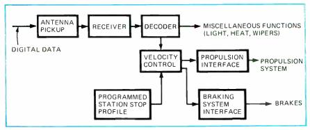
Vehicle control. Coded digital commands sent from the central computer on a 145-kHz carrier are received by the electronics on the vehicle, decoded and used to control speed
