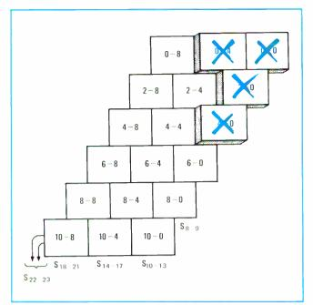
**6.** Truncation cuts cost. Dropping the least significant half of the full product without rounding gives a product with an error at most equal to the value of the least significant remaining digit, and permits omission of some of the multipliers.
