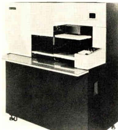
The machine uses a laser beam that passes through a lens onto the surface of the sheet. The reflected beams are received by a photomultiplier tube, and the resultant electrical pulses are then sent to a recognition-logic component. If characters are unrecognizable, the laser beam automatically rescans. If they are still unrecognizable, this is indicated on a CRT display so that correction can be made through a keyboard.
