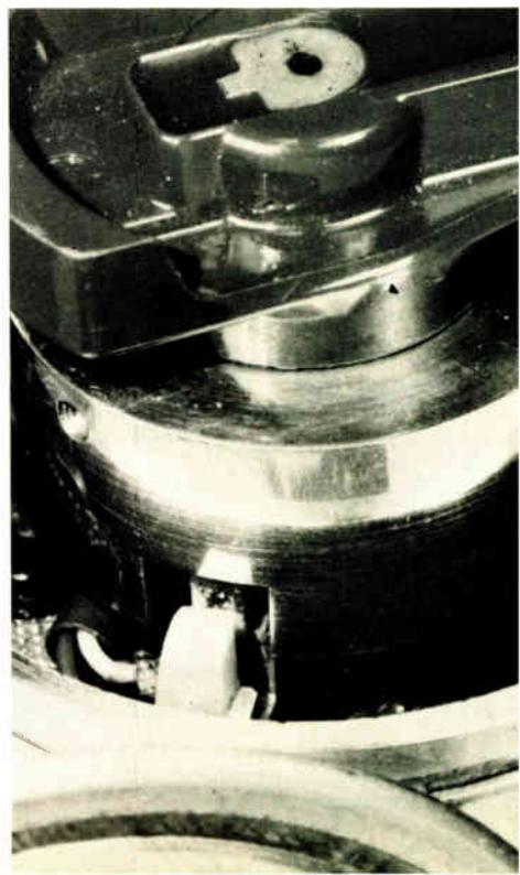
els some 3 millimeters to hit the phototransistor whenever a spark plug is to be fired.
