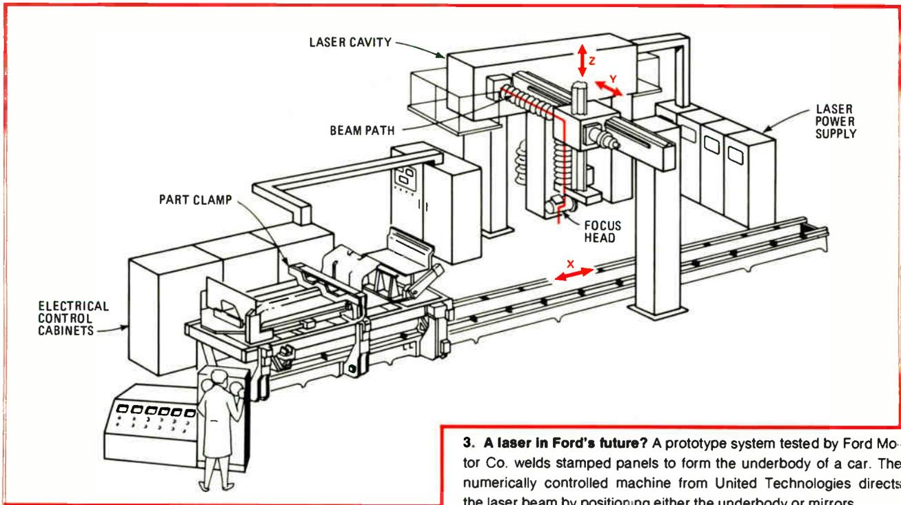
**3. A laser in Ford's future?** A prototype system tested by Ford Motor Co. welds stamped panels to form the underbody of a car. The numerically controlled machine from United Technologies directs the laser beam by positioning either the underbody or mirrors.
