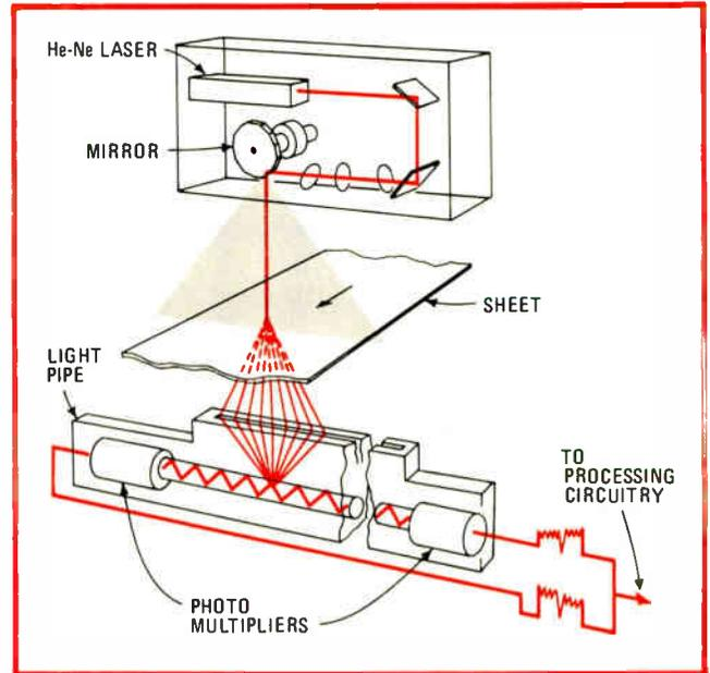
**2. Sheet inspection.** In Intec system, 12-faceted rotating mirror sweeps reflected laser beam across moving sheet. Two photomultiplier tubes pick up light, and their summed output contains transients whose amplitude and duration indicate flaw size and shape.
