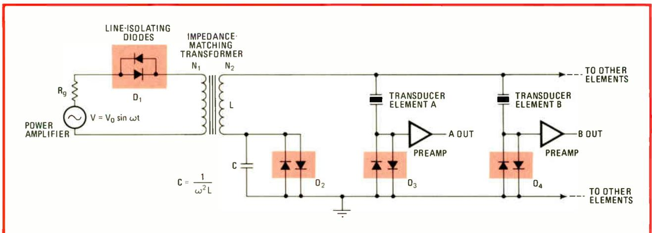
**1. Self-controlled.** Automatic solid-state transmit/receive switch uses pairs of diodes. High voltages during transmission drive diodes into conduction so that they appear as short circuits. Low voltages during reception leave diodes nonconducting so that they appear as open circuits. Capacitor  $C$  resonates  $L$  so that common sides of all transducer elements are grounded during receive mode.
