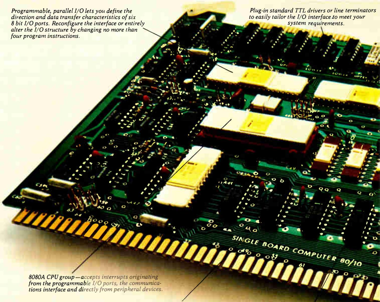
*8080A CPU group—accepts interrupts originating from the programmable I/O ports, the communications interface and directly from peripheral devices.*
