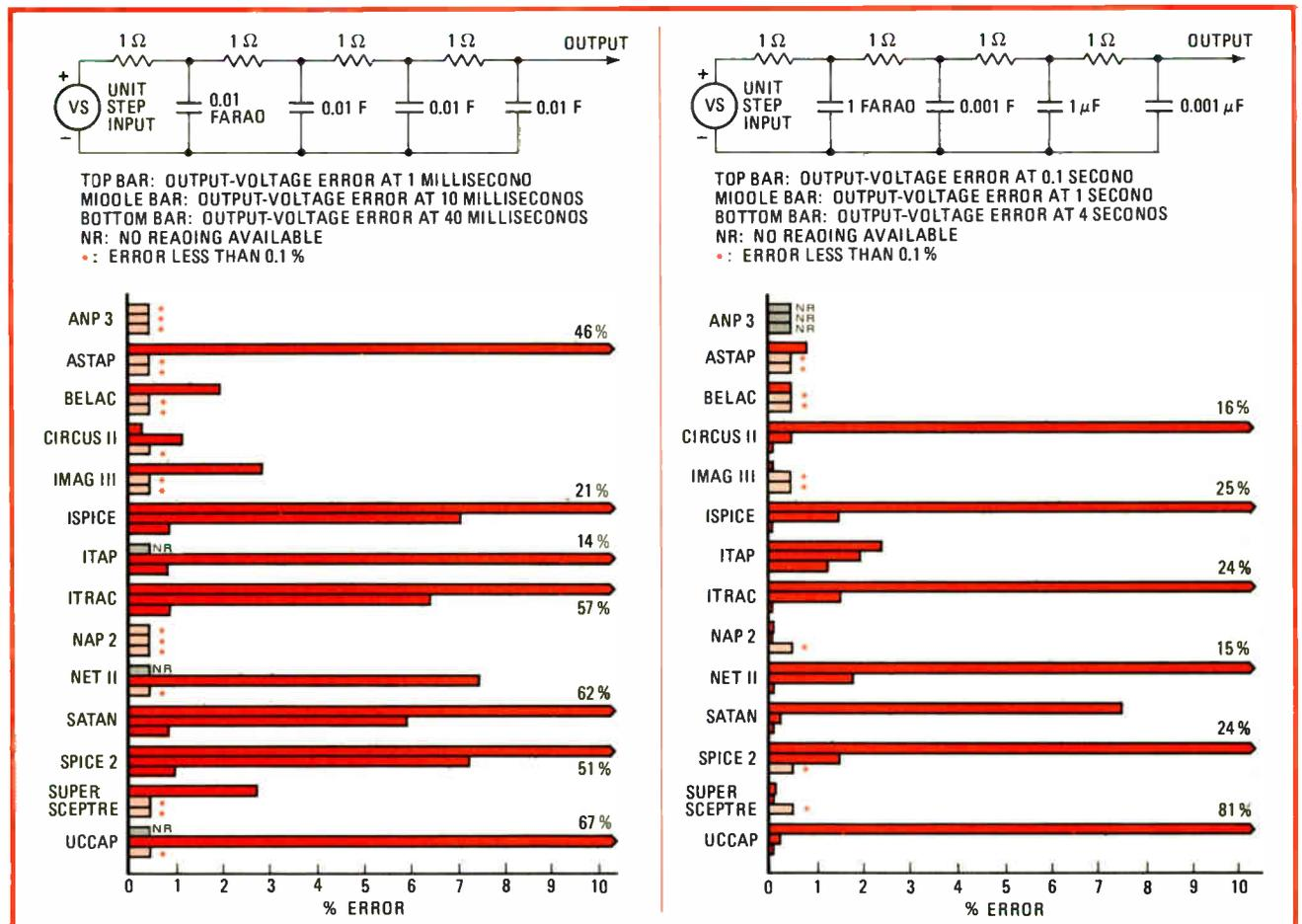
**2. Accuracy.** For the two four-stage RC ladder networks shown, the variation of the value computed by 14 CAD programs from values calculated by the investigators is given as a percentage error. The three times chosen represent points in the transient, settling, and steady-state phases of the circuits' operations. For programs accurate to a fixed quantity, small early errors can appear as a large percentage.
