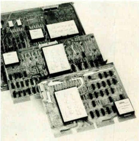
The Economy Series is rounded out by four control-only systems that include from one to four d-a converters but drop the input multiplexer, analog-to-digital converter, and sample-and-hold amplifier of the data-acquisition system. Pricing
