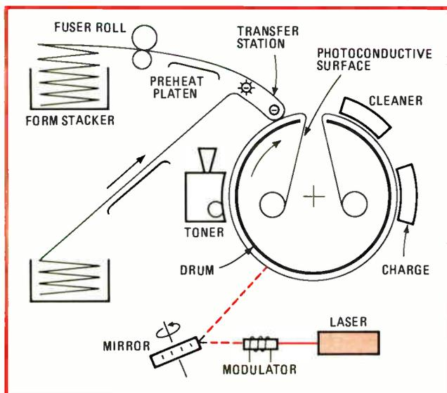
**6. Printing without impact.** Modulator interrupts laser beam in IBM printer, exposing the photoconductive surface of a rotating drum in a dot pattern. Multiple horizontal scans form line of characters, which are made visible by toner and then transferred to paper.
