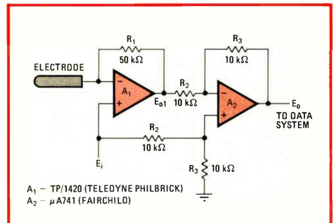
**Plasma probe.** Rocketsonde studies of density and temperature of electrons in the ionosphere may be achieved by measuring the current drawn to an electrode that projects out and is well insulated from the rocket body. The circuit shown here applies potential to the electrode through an op amp, thus avoiding voltage-supply-insulation problems and leakage errors in current measurement. Circuit measures currents from  $10^{-3}$  amperes down to  $5 \times 10^{-11}$  A.
