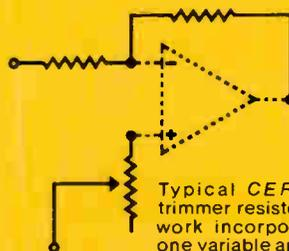
Typical CERBON trimmer resistor network incorporating one variable and two fixed resistors on dual substrate configuration.
