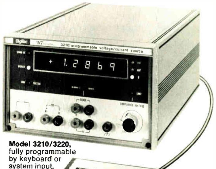
Model 3210/3220, fully programmable by keyboard or system input.
