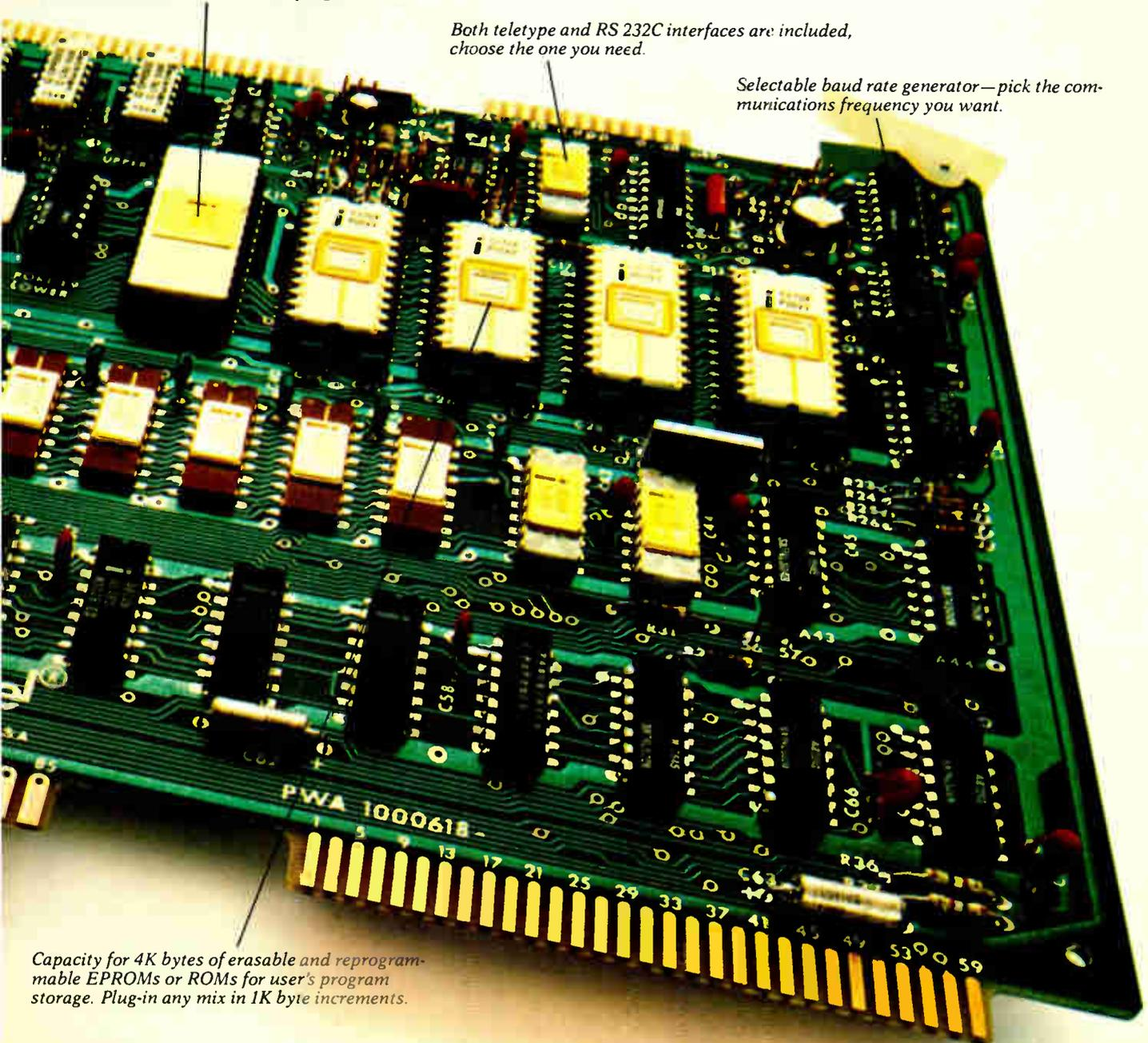
*Capacity for 4K bytes of erasable and reprogrammable EPROMs or ROMs for user's program storage. Plug-in any mix in 1K byte increments.*
