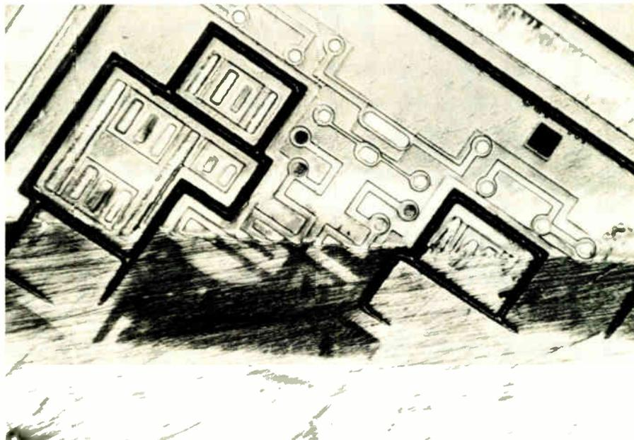
An example of the anodized silicon isolation process as used in the new generation of I<sup>2</sup>L devices.
