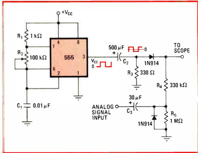
**2. Dots all, folks.** A 555 integrated-circuit timer generates pulses that drive the scope trace off scale with fast rise times and fall times, to produce a dotted or dashed display of a waveform. The timer frequency, set by  $R_2$ , determines the appearance of the trace.
