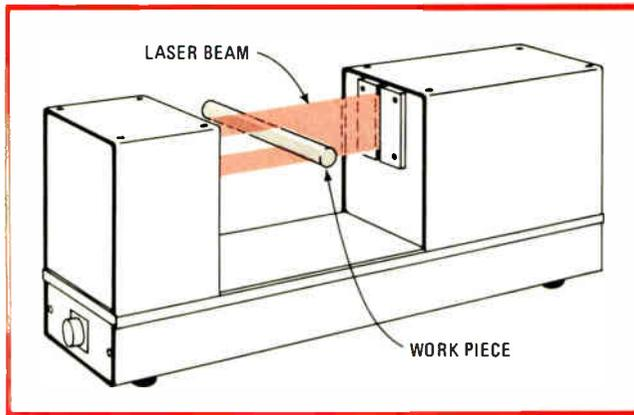
**1. Measuring size.** Beam of Techmet's Lasermike, deflected by rotating mirror, sweeps out vertical plane of light that's blocked by part moving down assembly line. Part size determines the length of time the beam is blocked. Resolution is typically  $\pm 0.005$  inch.
