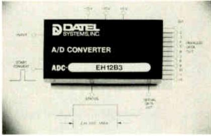
converter has an input impedance of 1.5 kilohms, an input-voltage range of either 0 to 10 volts or -5 to +5 v, and TTL-compatible serial and parallel outputs. A temperature coefficient of differential nonlinearity of less than 3 ppm/°C ensures monotonicity over the unit's operating temperature range of 0°C to 70°C. Priced at \$299 each in small quantities, the ADC-EH12B3 is available from stock to four weeks.
