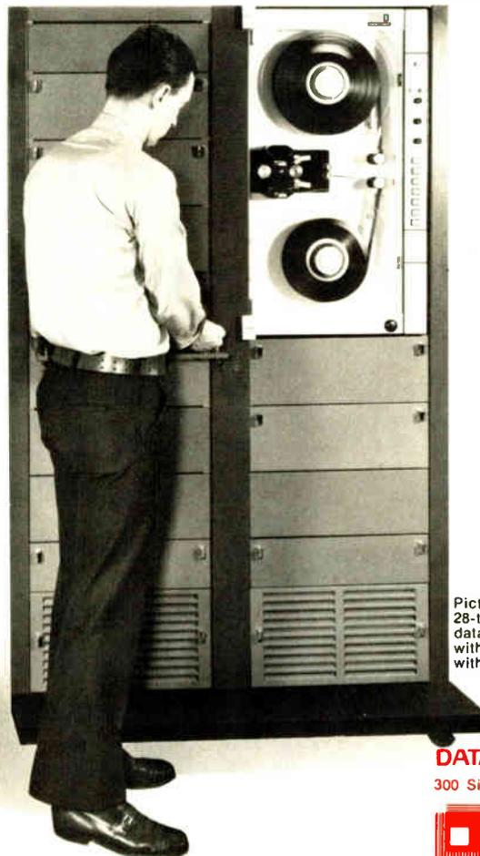
Pictured is a single transport, 28-track system capable of accepting data up to 92 megabits per second with errors as low as 1 in  $10^6$  without EDAC.
