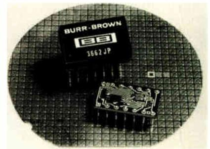
3662 KP has a maximum nonlinearity of 0.05%, a maximum drift of 2.5  $\mu$ V/°C at a gain of 1,000, and sells for \$23 in small quantities. Both units have typical common-mode input impedances of  $2 \times 10^{10}$  ohms shunted by 3 picofarads. All required resistors, except the gain-setting resistor, are included in the 14-pin dual in-line package, which measures 0.80 by 0.50 by 0.25 in. In hundreds, the JP version sells for \$9.75 and the KP for \$14.95.
