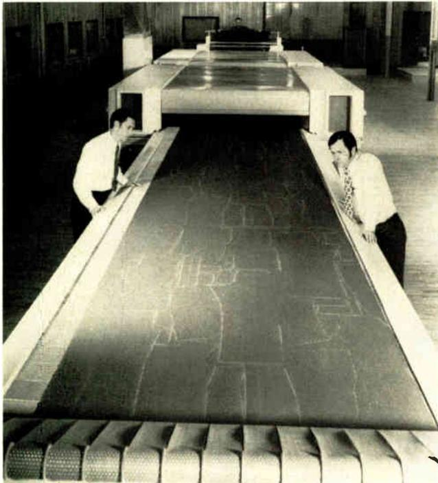
4. **Cutting to suit.** Laser cutter (left) developed by Hughes Aircraft cuts the fabric for men's suits, one layer at a time, at the rate of 80,000 inches an hour. A similar system (top) is now being used by McDonnell Douglas to cut boron epoxy material for the F-15.
