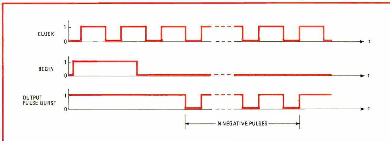
**1. Controlled pulse burst.** Applications such as circuit debugging require generation of a predetermined number of pulses. Basic timing is provided by a free-running clock, and the pulse burst is initiated by a begin signal that lasts for at least one clock period. Note that the negative output pulse sequence follows the first rising clock pulse after the begin command goes low.
