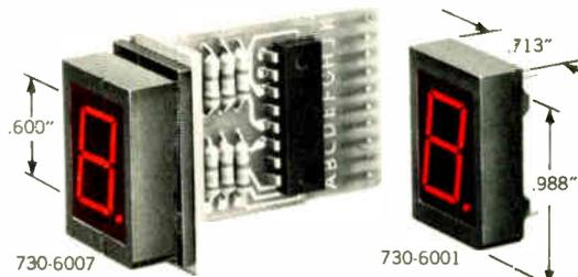
**730 SERIES** A new 0.600" LED character in super bright red, seven-segmented readout . . . low power . . . draws 10mA/segment or less . . . operates with standard IC power supply levels. Very high contrast ratio . . . visible from 40'. Available with or without on-board decoder/driver, plus or minus bar, and with bezel mounting. In 1000-ot quantities each LED
