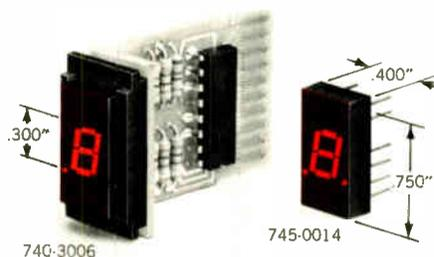
**745 SERIES** A new 0.300" LED character in a very bright red, seven-segmented readout . . . low power requirements. Standard 14-pin DIP . . . available with left and right decimal with  $\pm 1$ , and with and without on-board decoder/driver. Compatible with most TTL and DTL circuits. In 1000-lot quantities each
