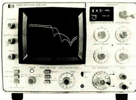
forming. Now with the tracking oscillator driving your filter, you can trim component values to optimize filter performance. Note how the tracking oscillator lets you observe the influence of each adjustment on filter performance — how it reduces the frustration you experienced before with interactive adjustments.
