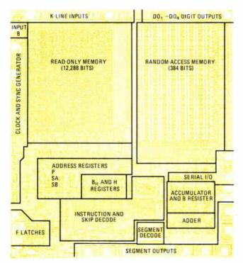
**1. Calculator-derived processor.** Part of a new family of dedicated microcontrollers is the MM5799 programable calculator chip. Designed for quick-turnaround applications, it contains all system timing, arithmetic and logic, control-ROM, and RAM functions.
