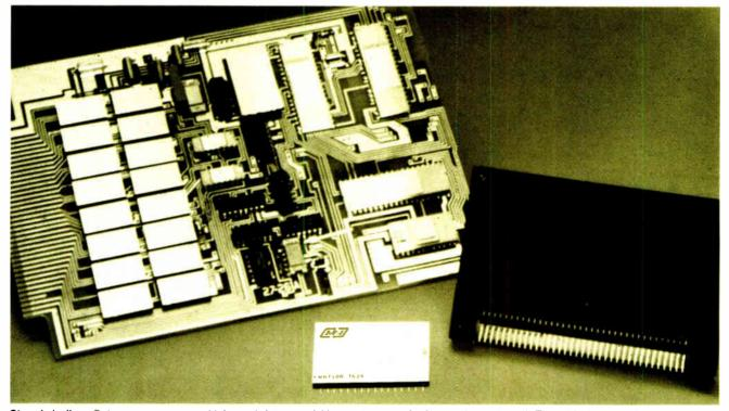
Size dwindles. Only a year ago, a multichannel data-acquisition system required an entire pc board. Then 16-channel 12-bit systems became available as hand-sized modules. And now a complete eight-channel 8-bit system has been squeezed into an IC-compatible DIP.
