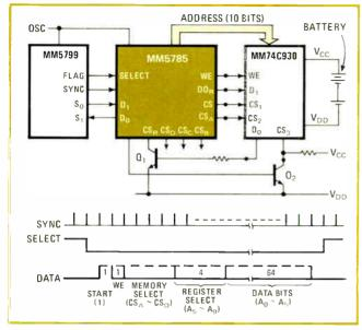
4. **Expansion.** Although designed to be self-contained, the controllers can be expanded by being linked to standard 1.024-bit RAMs through the MM5785 RAM interface elements. Schematic and timing diagram show how this works for the MM5799 controller.
