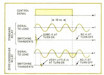
7. Solid-state comparison. With or without zero-crossover, solidstate relays generate only a fraction of the rfi produced by electromechanical units. Although zero-crossover versions create less rfi at turn-on than standard models, both types essentially eliminate rfi at turn-off. This is because each employs a thyristor output, and a thyristor is inherently a zero-crossover device for turnoff.
