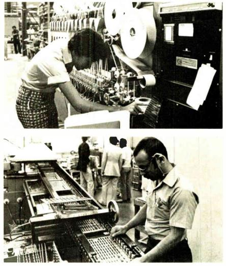
On their way. Top photo shows computer diodes being unrolled from shipping reels, while in bottom photo memory board is leaded onto belt of a wave-soldering machine
