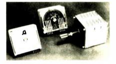
tions. Special features include modular stacking for multilayer operation and snap-together construction. A specially processed printedcircuit disk provides full programing to any truth table and allows the use of any code.
