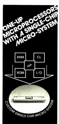
Microprocessor, Memory, I/O and Clock on the same chip optimized to your needs including special instruction set.
