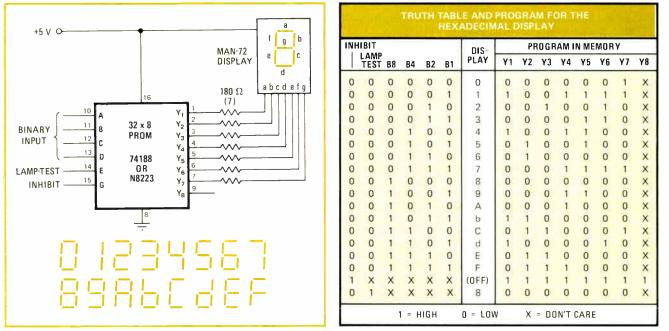
**Remember the hex symbol.** Binary inputs to the PROM produce a seven-segment representation of hexadecimal-code symbols. The PROM costs about \$3, and can be programed quickly at practically no cost if an automatic programing machine is available.
