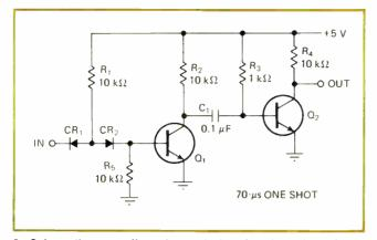
**3.** Schematic conventions. In a typical engineering schematic, the component symbols are labeled and arranged to show how they interact. Each symbol and notation has a function in helping understand how the actual hardware works.
