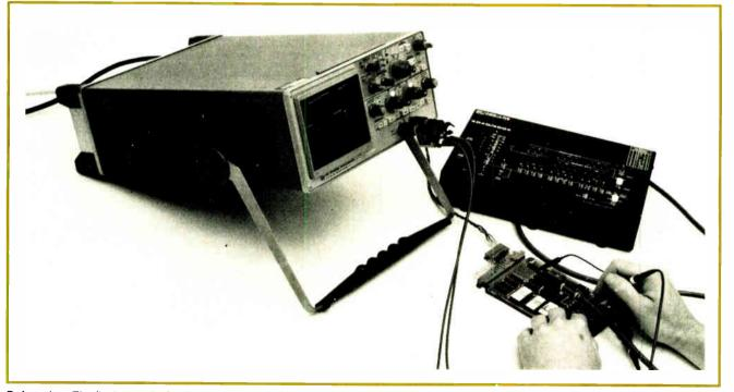
**Debugging.** The final stage in the design of a microprocessor system is to see if the program works as it was designed to. Here, an oscilloscope and a system analyzer are being used to debug a system whose program is in a PROM, equivalent to a circuit breadboard.
