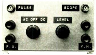
2. All packed up and ready to go. Complete electronic load circuit, including the 9-volt battery that powers it, is housed in a standard 3-by-2-by-5<sup>1</sup>/<sub>4</sub>-inch aluminum box. Connectors can be seen.
