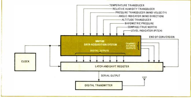
6. Digital transmission. Data is frequently sent in digital rather than analog, form to take advantage of faster speeds and simpler systems designs. Here, on board a weather balloon, the MN7100 translates atmospheric and position information to a digital transmitter.
