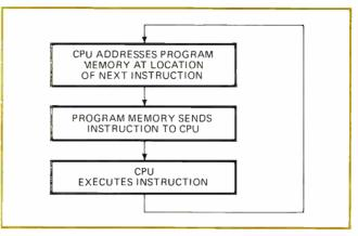
4. Instruction cycle. To execute one instruction, a microprocessor typically goes through three fundamental steps—addressing memory, extracting the instruction from memory, and performing the operation. A typical cycle takes about 11 microseconds.
