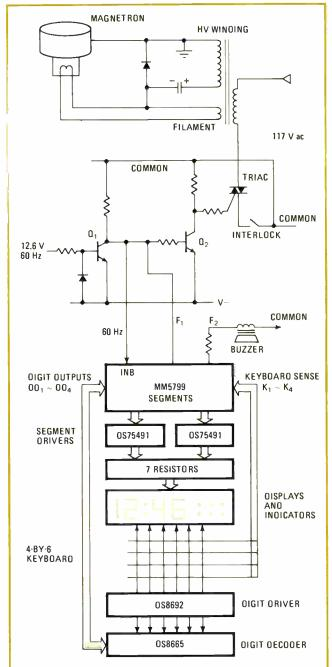
**5. What's cooking?** This microwave-oven controller shows the efficiency of design with a dedicated microcontroller. Relatively few components are needed to achieve, virtually automatically, all the timing and control functions involved in household cooking.
