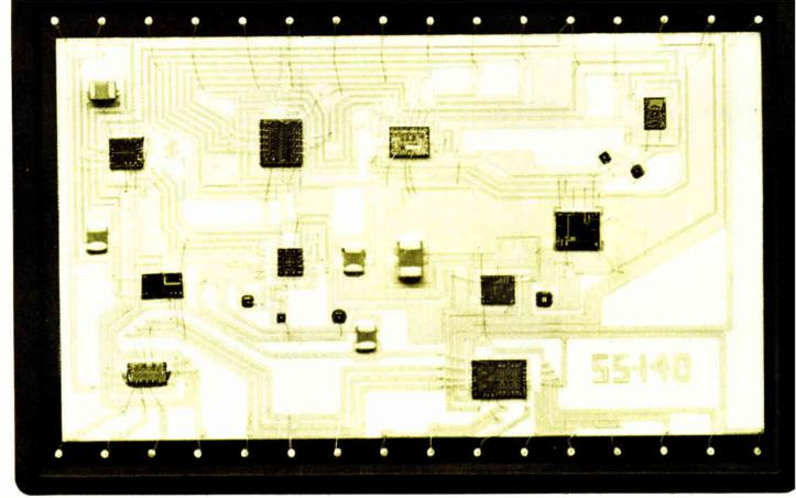
1. Uncovered. Inside the 32-pin DIP of the MN7100 data-acquisition system is a 21-chip, thin-film hybrid circuit that can multiplex, sample and digitize eight analog inputs. The device even includes integral clock, control logic, and voltage-reference source.
