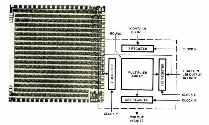
The first monolithic-bipolar, 16 x 16-bit multiplier (MPY-16) is now available from TRW. It's fully TTLcompatible, too. A single MPY-16 package can replace as many as 50 MSI/TTL packages. eliminating 2 x 4 multipliers.
