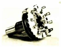
**Obsolete?** Each wiring terminal in conventional rotary switch must be handled individually, adding to the unit's cost.
