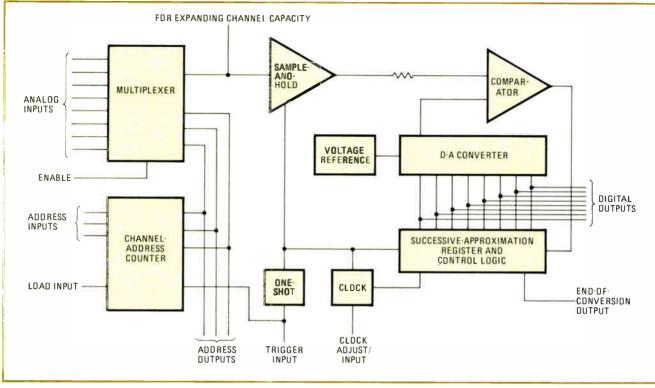
2. The works. Circuit operation of the MN7100 is fairly conventional. The desired input channel, selected via the address counter, is fed to the sample-and-hold amplifier by the multiplexer. When the sample-and-hold changes from track to hold mode, the signal is digitized by the a-d converter, which is composed of the d-a converter, the comparator, the voltage reference, and the logic register.
