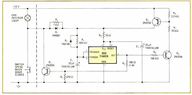
**Holds the light.** When car door closes, output current pulse from 555 timer turns on transistor  $Q_1$  to keep interior light on for about 10 seconds. This type of one-shot arrangement, driving the line that is sensed, can be added at any point in the circuit. It is useful in alarm systems, process controls, automatic machinery, safety circuits, and convenience circuits such as this one.
