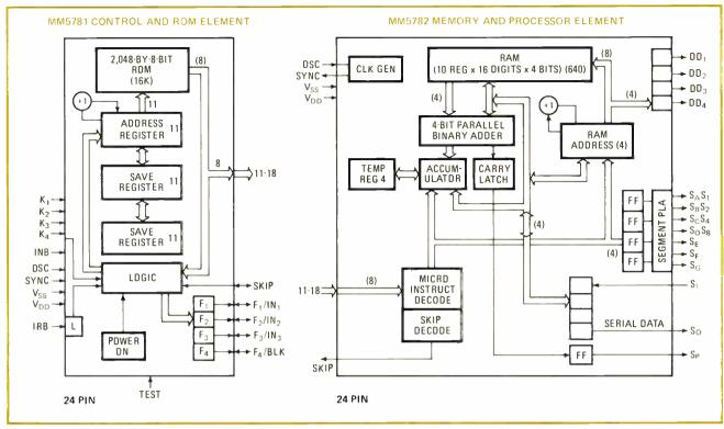
**3.** Added power. Two-chip microcontroller carries more internal ROM and RAM capacity than one-chip versions, making more powerful control systems possible. Program storage and control fit on the MM5781 program chip, with processing and RAM storage on the MM5782.
