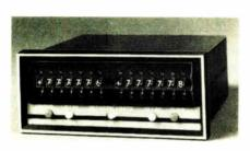
ture is the set of comparison-logic outputs that are available at the rear connector—using gatable, latchable, open-collector transistor-transistor logic. This forms a data bus that enables the 8400 series comparators to interface with a central process computer. For additional versatility, the comparison-logic outputs can be multiplexed onto buses with 4, 8, 16, or 24 wires.
