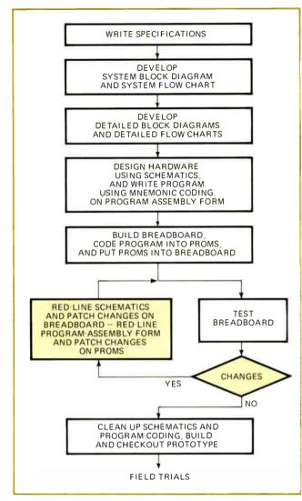
7. **Program design.** The procedure for writing a microprocessor program is similar to that of designing hardware. For every step in hardware design, there is an equivalent step in program organization, so hardware and software elements appear together.
