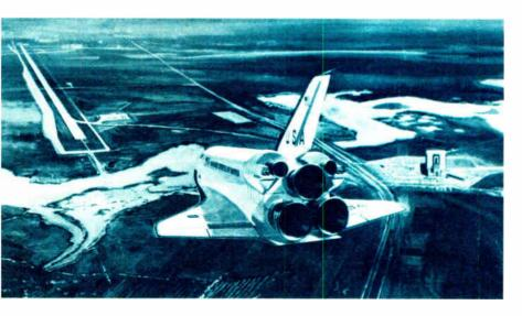
control functions is unprecedented. Rubenstein says. "It has to fly a craft that goes up like a rocket booster, orbits in space for up to 30 days as a space lab at 18.000 miles an hour, returns to earth as a re-entry vehicle, and lands like an airplane." Landing the orbiter without power at 250 miles per hour with only one chance to hit a 150-footwide, 15,000-foot-long runway has never been tried before, the Rockwell engineer notes.
