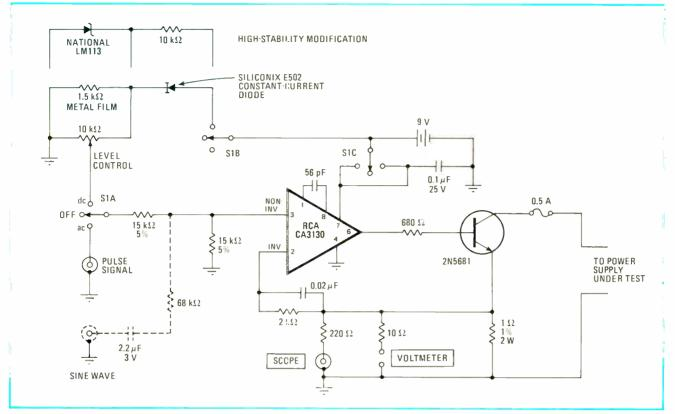
**1. Electronic load.** Characteristics of a power supply are tested with this circuit, which controls current delivered by the supply. Regulation, ripple, transient response, and temperature effects can be measured at currents up to 1. A peak or 0.25 A dc and voltages of 1.5 to 100 V.
