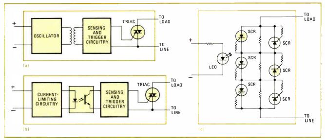
5. Standard solid state. Because they don't include optional zero-crossover circuitry, standard solid-state relays are generally about 30% ess expensive than their zero-switching counterparts. Here, three versions are shown: transformer-isolated (a) and optically isolated with either a phototransistor (b) or a chain of photo-SCRs (c). The latter configuration is used to obtain very high blocking voltage
