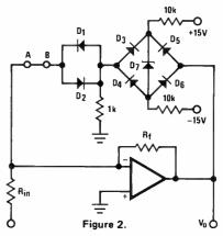
Figure 2, however, improves limiting, and in fact performs quite well. Here, the diodes do not add much capacitance across the feedback resistor. And all diode leakages are absorbed by the 1-k $\Omega$  resistor. D7 will be, typically, a 9.1-V Zener for an 11.8-V limit. At V<sub>0</sub> = 10 V, leakage will be less than a nanoamp; but at ±11.8 V the limiting circuitry will conduct more than 2 mA. As the same Zener conducts for both polarities of the input, output symmetry is very good.
