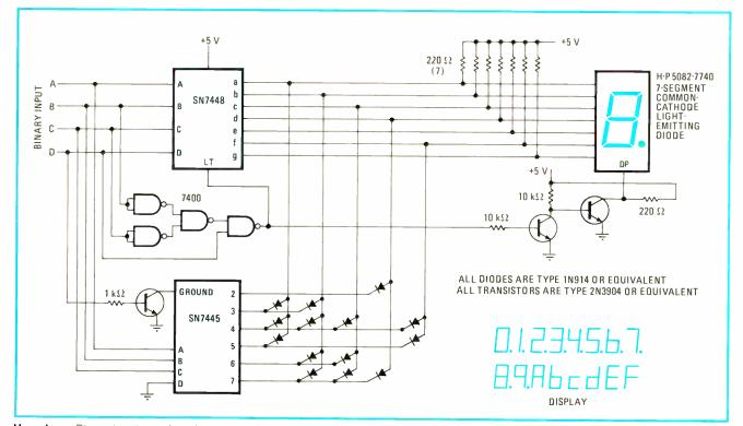
**Hex signs.** Binary inputs produce hexadecimal code on a standard seven-segment display with this circuit. To emphasize distinctions between numerals and letters, a decimal point is activated for numbers 0 through 9, as shown. Cost of parts (not including LED display) is less than \$5. For more than one digit, the inputs can be multiplexed. Pull-up resistors may not be required for small displays.
