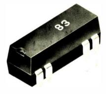
grid to fit all standard DIP sockets. Because it has three poles, compared with a maximum of two for previous units, the series 83 reduces required printed-circuit board space and per-pole cost. Contact rating is 10 watts with a maximum switching voltage of 100 volts dc and a maximum switching current of 0.5 ampere. Three standard coils are available: 150 ohms for 5-volt applications, 450  $\Omega$  for 12-v, and 750  $\Omega$ for 24-v dc.
