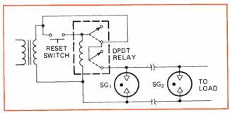
1. Load protection circuit is first reset, energizing relay and connecting load to supply; relay is held energized via its own contact. If transient occurs,  $SG_1$  fires, and its voltage drops below voltage needed to hold relay, opening contacts and disconnecting load. Second spark gap is used if load is connected through long length of line, susceptible to transient pick-up.
