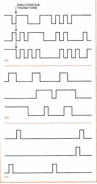
1. **Pseudorandom patterns.** Three types of pseudorandom sources are (a) one that allows transitions on more than one line at a time, the so-called Trendar generator; (b) the pseudo-Gray generator, in which only one line transits at a time; and (c) the 1-of-N generator, in which a pulse appears on only one line at a time. Waveforms are shown for three of 32 available lines in each case.
