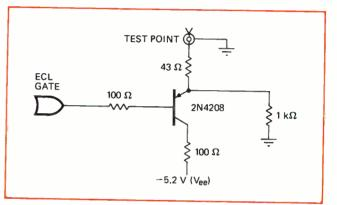
**7. Wideband sync.** This single-transistor amplifier makes a good circuit for driving counters and external sync inputs on sampling and other wideband oscilloscopes. Matched to emitter-coupled logic, the circuit produces 400 mV of signal into a 50-ohm load.
