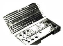
on the board, and the circuit was operated at a power of 170 watts while maintaining a case temperature rise of all semiconductors within acceptable tolerances. The same circuit on a G-10 epoxy board would be able to operate at a power level no higher than 12 watts. International Electronic Research Corp., 135
