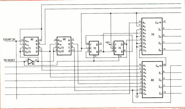
5. Adder activity. Another section of memory-control system has two four-bit binary adders, 6D and 7D. Inputs COUNT 4X and TD RESET must toggle J-K flip-flops with enough activity to provide adequate adder inputs before reset. Pseudorandom and Gray clock signals do this.
