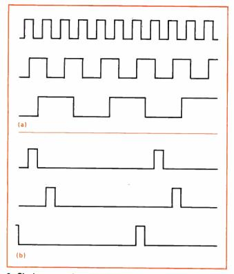
**2. Clock sources.** Gray clock generator (a) allows one bit stream to transit at a time (three of 24 bit streams shown). The eight-phase clock generator, useful for MOS circuits, is shown in b.
