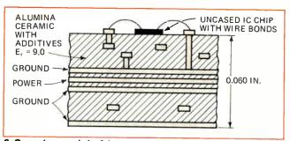
**3. Ceramic speed.** An 8-layer ceramic substrate allows logic speeds up to 1 gigabit per second. Uncased monolithic chips allow required miniaturization and complete the low thermal-resistance path from heat sink, through ceramic, to device junctions.
