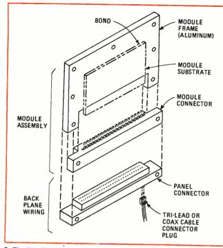
5. Flexible interface. Module connector assembly allows complete plug-in capability for the high-speed modules. The panel connector, mounted to the chassis, interfaces with three-conductor cable plugs for matched-impedance tri-lead or coaxial cables.
