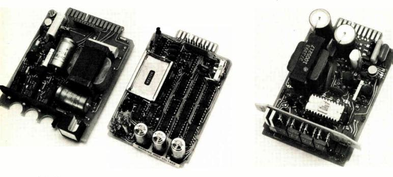
4. Looking for reliability. Fewer components mean better reliability. This manufacturer has substituted a single IC for the 14 IC packages required in his older model, has reduced the package design to one circuit board instead of two, and cut the number of connections.
