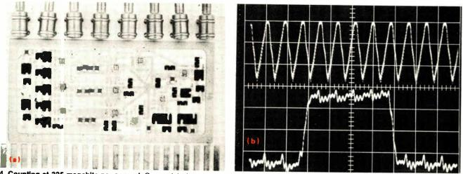
4. Counting at 325 megabits per second. On an eight-layer ceramic substrate, a fully decoded decade counter (a) has been operated at 325 megabits per second, limited solely by the 10 logic chips. The clock and a divide-by-10 output (b) show binary wave-shapes at 250 megabits per second. Horizontal scale is 5 ns per division; vertical scale is 200 mV per division with logic levels at about -0.8 and -1.7 volts.
