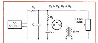
2. Two-terminal spark gap repetitively triggers flash tube when  $C_2$  charges to the gaps breakdown voltage. Capacitor  $C_1$  then releases its charge through the flash tube.
