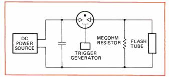
3. Three-terminal triggered spark gap fires flash tube when pulsed. Megohm resistor provides path for trigger pulse and also for initial rush of current through spark gap.
