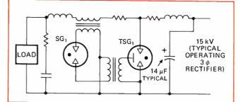
**4. Crowbar protection** against overcurrent surges is provided by  $STG_1$ , set to trigger from the secondary of the series transformer,  $T_1$  and  $TSG_1$ , which absorbs overcurrent when triggered.
