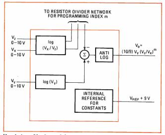
**Handy logarithmic module** has output that is function of three inputs:  $V_0 = V_y (V_z / V_x)^m$ . Two resistors set value of exponent m.
