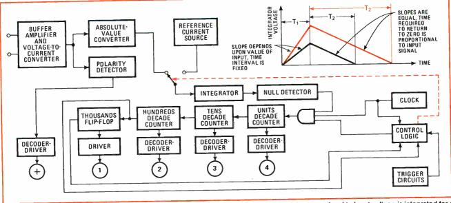
1. Heart of the meter. Typical, simplified DPM is built around a dual-slope converter. Current proportional to input voltage is integrated for a fixed length of time, T<sub>1</sub>. Integrator is then discharged at fixed rate, set by reference current source. Time needed to reach zero, T<sub>2</sub>, is measured by decade counters. Larger signal (shown in color) needs more time to reach zero than smaller one does.
