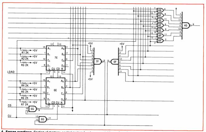
4. Forces overflows. Section of memory-control system has two presettable up-down four-bit binary counters. Preset data words applied to pins 15, 1, 10, and 9 are represented by pseudorandom signals; LOAD input is driven by Gray lock square wave.
