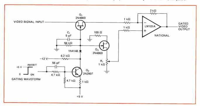
acteristics for both  $Q_1$  and  $Q_3$ . This eliminates the need for a matched pair of FETs. By simply adjusting resistor  $R_1$ , nearly all of the transients can be cancelled.
