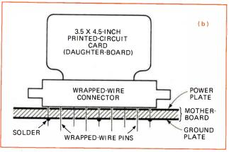
1. 100-megabit-per-second module. A conventional two-sided printed-circuit card (a) provides good signal fidelity up to 100 megabits per second. Wrapped-wire connector (b) eases mechanical transition into motherboard and speeds system assembly.
