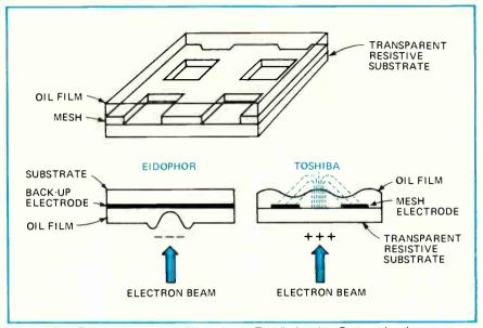
**Picture this.** Top drawing shows light valve in Toshiba's tube. Bottom drawings compare Toshiba and Eidophor light valves. In the Toshiba model, the oil doesn't degrade.
