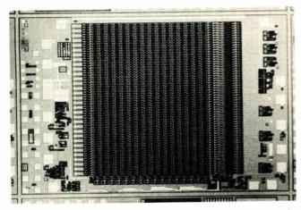
**5. Beating the system.** A 4,096-by-8-bit memory system using the V-ATE 1,024-bit RAM (RR5502) requires very few additional packages, unlike MOS systems, and offers access times of 25 to 35 ns from board select to data out. The memory is easily expandable, without extra buffers, because of the low address input currents.
