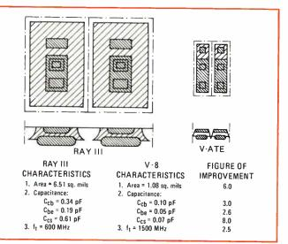
2. Old and new. A topological, cross-sectional, and parameter comparison of the conventional bipolar technique with V-ATE shows that large areas of wasted space have been eliminated and performance has been improved with the new process.
