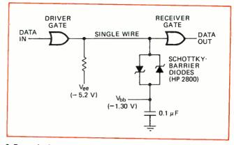
**6. Dynamic duo.** A pair of Schottky diodes at the logic gate receiver reduces the effects of overshoot caused by a termination mismatch. The technique, first developed by O.A. Horna at Comsat in 1969, is often used as a dynamic nonlinear termination for long wires.
