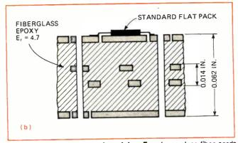
**2. 200-megabit-per-second modules.** Four-layer glass fiber cards (a) serve as the building blocks for circuits operating to 200 megabits per second. Interconnect layers (b) function very much like stripline. Lines in these layers are usually mutually perpendicular, resulting in crosstalk more than 20 dB below signal levels.
