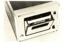
different lengths and are located by address without rewinding. The ability to find a file by number also lets the user recall data from that file, modify it, then restore it to the same file without rewriting on a second cassette. Search speed is 130 feet per minute in either direction. Price is \$1,750.
