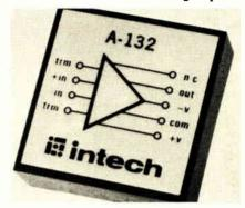
logic, cables, or other capacitive loads to 1,000 picofarads. Openloop gain is typically 100 decibels, and bandwidth is 20 megahertz minimum. Input bias current is less than 50 pA, and input drift is 50  $\mu$  V/°C. Price is \$57, and delivery is from stock.
