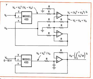
**Outboarding one or more op amps** permits module to find vector length (top) or solve for root-mean-square sygnal values (bottom).
