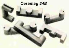
Tektronix, Inc. selected 24B for their "U" and "E" cores. This proven material has seen years of service in flybacks for television. Ideal for power applications, it can be operated at higher frequencies than laminated steel. It is cool running, due to low losses under power conditions and controlled power permeability. Tooling is available for a wide range of "U", "E" and "I" configurations.
