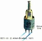
Operational range  $-65^{\circ}$  to  $+150^{\circ}$ C. Rotational life 25,000 cycles with less than a 10% resistance change. Resistance range 50 ohms to 1 meg. For panel or PC board mounting. Leads fit standard 0.1 inch spacing. Immersion-proof, can be encapsulated. Plain or locking
