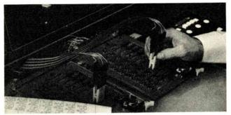
6. Compare and test. Troubleshooting by comparison tester, once fault is discovered on board under test, is performed with pair of dual in-line package test clips. Fault is traced back from output.
