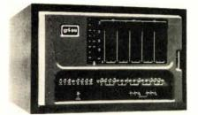
each in quantity. The unit is in a class of general-purpose computers known as direct-function processors, and is aimed at applications requiring wholly dedicated systems. The internal architecture and machine language use a universal bus system.
