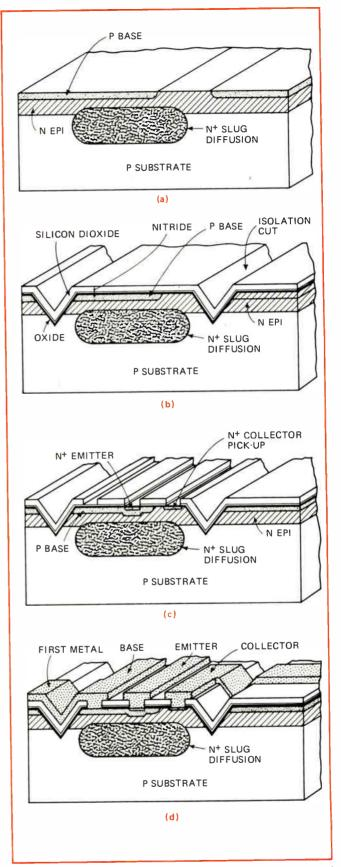
3. V-ATE processes. In the earlier steps (a), the epitaxial layer and base diffusion have been completed in readiness for the vee-etch. In (b), the process has been taken through the vee-etch and the oxide-nitride-oxide sandwich, while (c) shows the emitter diffusion. Then in (d), the first layer of metalization is deposited.
