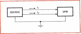
**3. Blas current.** For the differential-input configuration shown, the bias current is either  $I_1$  or  $I_2$ , whichever is greater. The offset current  $(I_1 - I_2)$  is most important when the source resistances are equal.
