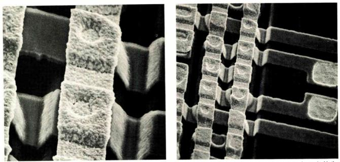
1. Groovy. Clearly visible in the scanning electron microphotograph of a memory subfunction (a) are the isolation grooves formed with the V-ATE process. Shown in (b) are strings of cells with double metalization and cross-overs. In the case of the titanium-platinum-gold metallurgy, note the absence of hillocks and bumps that are usually present with conventional aluminum systems.
