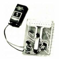
Game guts. TI board in Parker's sub chase game holds microprocessor, resistors, discrete LEDs and, under lenses at top, segmented LEDs. Wires go to keyboard.
