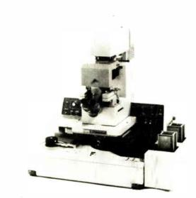
**9. Reduction projection.** Canon's FPA-141 step and repeats a 4:1 mask image onto a resist-covered silicon wafer. The unit can print 0.89- $\mu$ m lines in positive resists and 1- $\mu$ m lines in negative resists.
