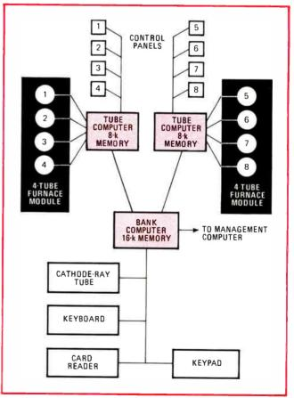
**15. Direct control.** Thermco's direct digital control system for an 8-tube diffusion furnace uses three LSI 2/20 minicomputers—one bank computer and two tube computers. Each tube computer controls four diffusion tubes and eliminates all analog controllers. The bank computer supervises the other two computers.
