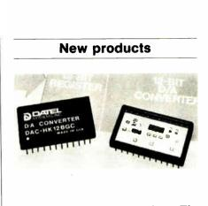
amplifier, and the input register. The quad current switches, combined with a laser-trimmed nichrome resistor network, give the converter its differential linearity temperature coefficient of 2 ppm/°C.
