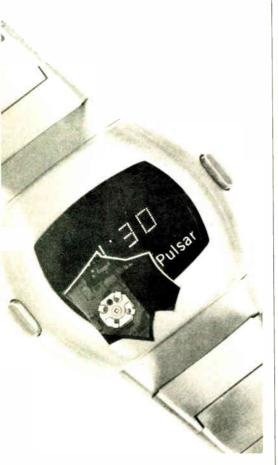
Tucked in the corner of this Pulsar Watch is a miniature pacitor which is used to trim the crystal. ais Thin-Trim capacitor is one of our 410 series, has an adjustment range of 7 5.45 pf., and is .200" x .200" x .050" thick. the Thin-Trim concept provides a variable levice to replace fixed tuning techniques ind cut-and-try methods of adjustment. Thin-Trim capacitors are available in a variety of lead configurations making them very easy to mount.
