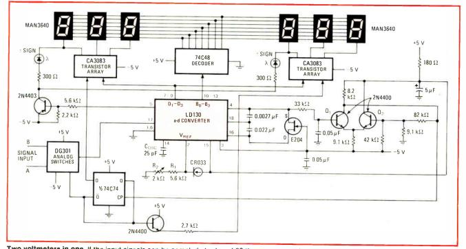
Two voltmeters in one. If the input signals can be sampled at rates of 60 times per second or greater, they can be measured, then observed simultaneously at acceptable flicker rates. Key to circuit operation is use of fast-sampling analog-to-digital converter.
