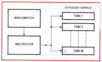
**14. Minicomputer control.** One of the first approaches to automating multiple diffusion tubes was to let a minicomputer with a multiplexer act as the master controller. However, failure of either of these components disables all the diffusion tubes.
