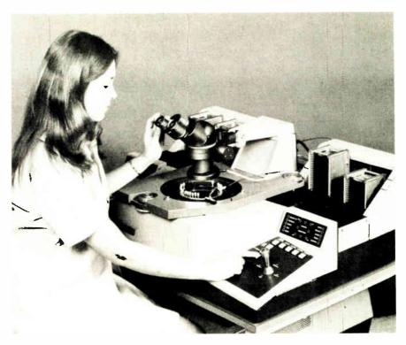
**17. Microprocessor control.** The Electroglas Model 1038 reflects the improvements that IC firms wanted in probers. It is microprocessor-controlled and has a cassette-tocassette mechanical interface and Z-axis compensation for wafer warpage.
