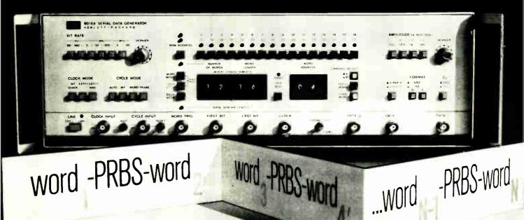
In MIXED MODE, HP's 8018A alternately generates PRBS and word information, simulating preamble-data message-postamble patterns.
