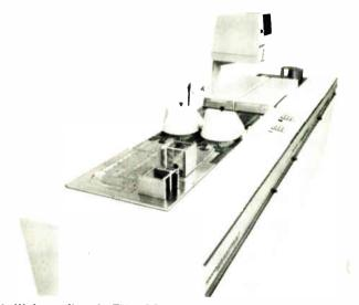
**4. Water railroad.** This GCA Watertrac in-line system takes cassettes of waters through a microprocessor-controlled sequence of scrubbing, baking, spinning, and developing. It needs only a single person to load and unload the input and output water carriers.
