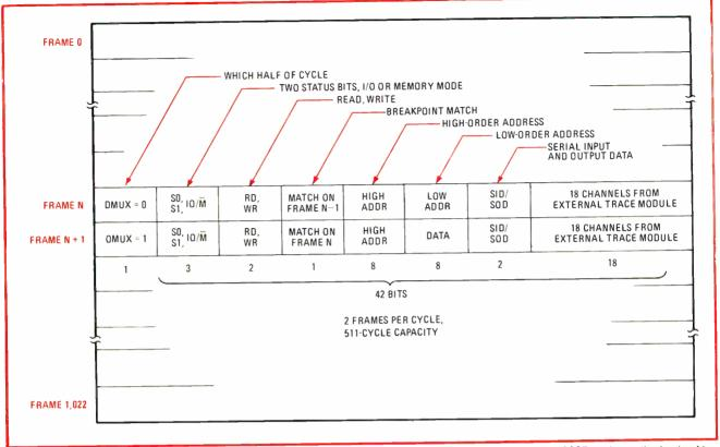
4. Trace memory. For logic analysis, the ICE-85 trace memory holds 1,023 frames of 42 bits each. Since the 8085 works on the basis of two trames per cycle, with low-order addresses and data multiplexed in alternate frames, the memory can store up to 511 machine cycles.
