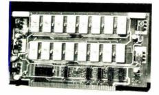
the 8,192-bit memories, the unused sections can be disabled so that a read/write memory can be accommodated within their address space. The board also has provision for a wait state so that it can run in a Z-80 system. Supplied with a full set of integrated-circuit sockets, but without the PROMS, the kit has a small-quantity price of \$85. Delivery is from stock.
