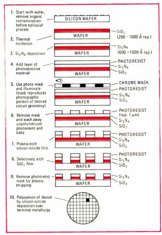
**11. Plasma processes.** A typical process for a silicon wafer shows that plasma processes may be applied for wafer cleaning, oxide etching, resist stripping, and silicon-nitride deposition (passivation).
