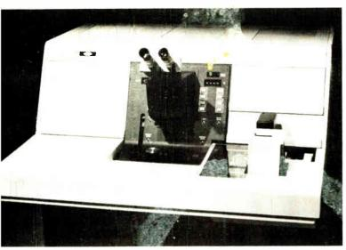
8. Projection aligner. Perkin-Elmer's Micralign model 140 directprojection mask aligner can expose 90% of a 4-inch wafer and is equipped with automatic wafer loading. Older versions of this unit are used for much of the current projection lithography.
