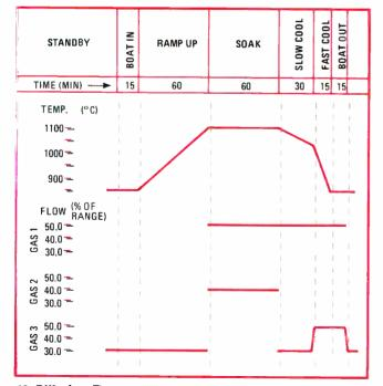
**13. Diffusion.** Time, temperature, and gas flow are controlled in the diffusion process. Note that temperature vs time functions use ramps rather than step functions to maintain process control.
