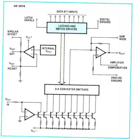
goes high, the input data present at the moment of transition is latched and retained until the enable input again goes low.
