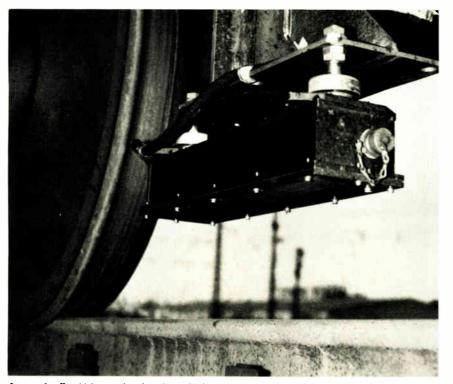
Accurate fix. Using radar-doppler principles, sensor unit above measures railway train's speed with  $\pm$  1% accuracy and distance from starting point with  $\pm$  0.1% accuracy.
