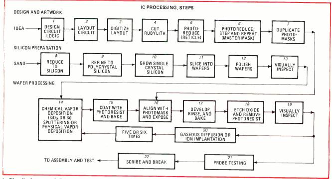
1. Circuits from sand. Fabricating a wafer of ICs involves many techniques: circuit design, photoreduction, photolithography, wet and dry chemistry, materials handling, metal deposition, and gaseous diffusion. Last steps in the process are inspection and electrical probing.
