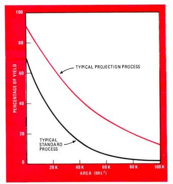
**7. Big chips.** As chip area increases, probe yield goes down. For a usable yield on LSI wafers, many IC firms are switching from contact lithography to projection alignment and printing.
