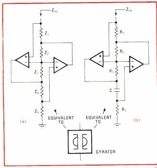
**2. Reatistically.** Preferred gyrator realization (a) requires two amplifiers and five impedances. In practical RC implementation (b), impedance  $Z_4$  is a capacitor, and the other impedances are resistors. The gyrator may also be represented by the special symbol shown here.
