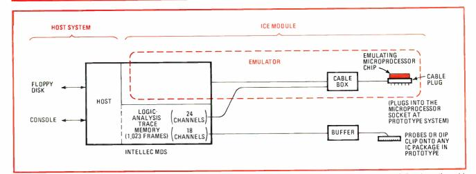
2. The ICE-85 module. The in-circuit emulator for the 8085 microprocessor has the emulating microprocessor mounted directly on the cable plug, which is inserted in the prototype. This eliminates signal delays in the cable. A DIP clip holds 18 leads for extra debugging capability.
