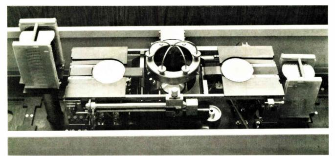
**3. Untouched by human hands.** Pneumatically driven teflon supports transport wafers in Macronetic's in-line wafer-processing equipment. Wafers move from the left cassette to the transport, through a scrubber, to the right transport, and back to a cassette.
