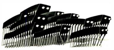
2K x 8. We also have a 3508, organized 1K x 8. Our 3516E features a 5-volt power supply. All inputs and outputs are TTL-compatible. It also features microprocessorcompatible access times, 3-state outputs and completely static operation.
