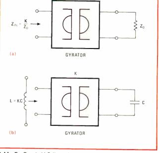
**1. Ideally.** Coupled LC filters simulated with gyrators have characteristics approaching the ideal. In effect, the gyrator is a lossless twoport circuit (a) that inverts a load impedance. With a capacitive load impedance, the circuit (b) simulates a high-quality inductor.
