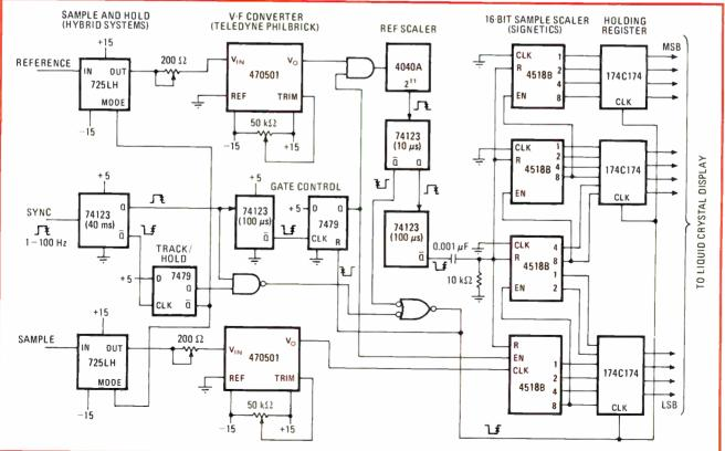
2. Digital normalization. Circuit detects relationship of analog sample amplitude to reference voltage by digital means. Several one-shots are used to obtain proper timing and gating. Circuit uses C-MOS devices where possible to reduce power consumption.
