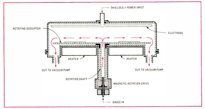
12. Parallel plate. A new type of reactor using parallel-plate construction, rather than the older barrel method, is appearing for both etching and deposition. Applied Materials uses the parallel-plate reactor, shown in cross section, in its Plasma 1 silicon-nitride deposition unit.
