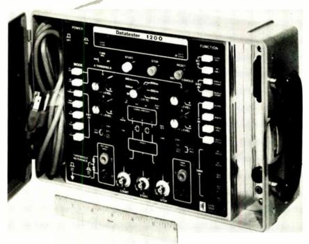
**Heiper.** Somewhat bulkier than an attache case, the portable Datatester 1200 multifunction circuit-tester does the job of several separate instruments, including a digital multimeter and a frequency counter and timer. It also counts digital-logic transitions.
