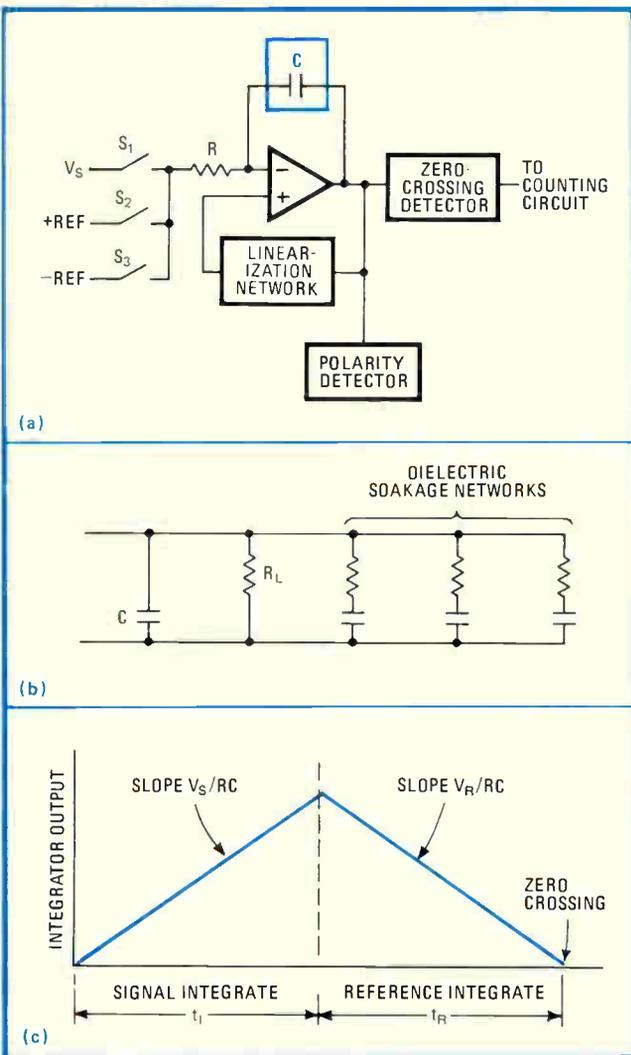
**2. Dual slope.** A modified dual-slope circuit is the heart of integrating a-d conversion. A simplified circuit is shown in (a). Departure from linearity can be introduced by the capacitor C's leakage resistance and less-than-perfect dielectric (b). A compensating network can make the integrator output approach an ideal linear ramp (c).
