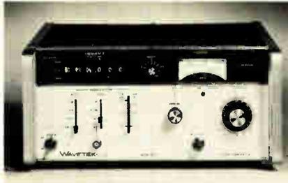
accuracy of 0.001% and a stability of 0.2 ppm per hour over its entire frequency range. The unit is frequency-programmable and, with the model 3911 general-purpose interface bus converter, is IEEE-488-1975-compatible. It can be operated in a-m and fm modes using either external modulation or internal 400- or 1,000-Hz frequencies.
