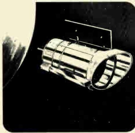
**IRAS - Infra-Red Astronomical Satellite** - due to be launched into a 900 kilometre polar orbit in 1981, is the first scientific satellite designed to make a detailed inventory of infra-red sources in space. The on-board computer, which will process about 500 million bits of measured data per day, will be supplied by us along with other electronic systems.
