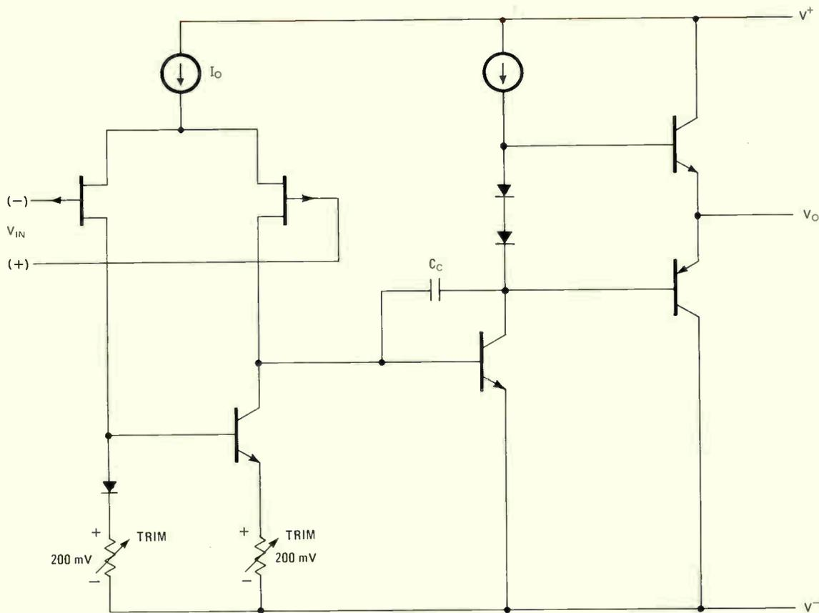
**4. Low cost.** Bi-FET op amps that are less complex and expensive than the LF356 are made by using laser trimming to adjust offset voltage right on the chip, instead of optimizing the design for low offset as with the LF356. A zener and a resistor set the input bias current.
