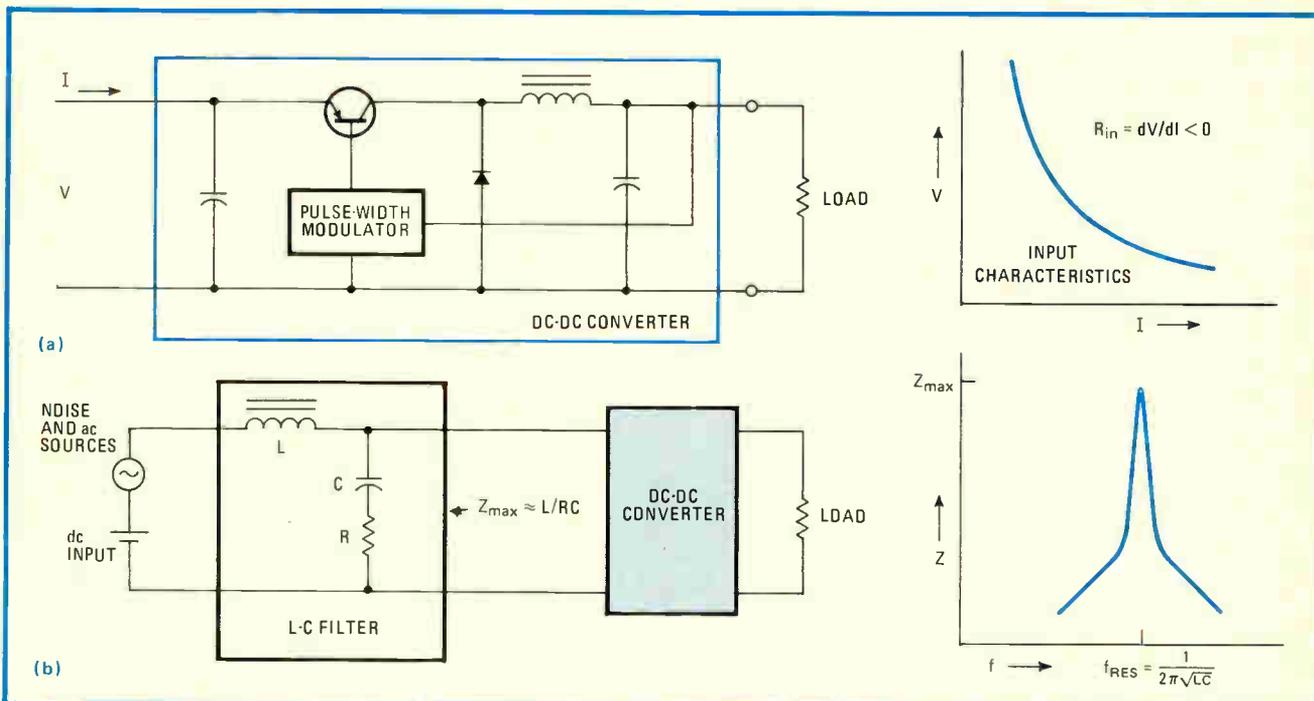
**Filter interaction.** Switching dc-dc converter (a) exhibits negative input impedance, causes converter/noise-filter combination (b) to oscillate at  $f_{res}$  if  $Z_{max} > R_{in}$ . For proper filtering, and to eliminate the possibility of oscillations, filter's L-to-C ratio must be reduced.
