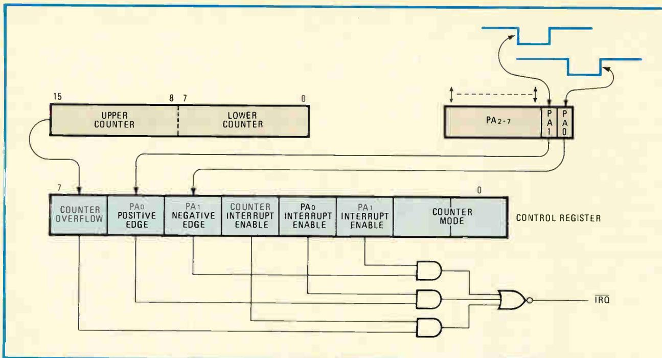
**5. Interrupts.** The  $\overline{\text{IRQ}}$  interrupt request originates from three sources that are each software-maskable: the rising edge at pin  $\text{PA}_0$ , the falling edge at  $\text{PA}_1$ , and counter overflow. The other interrupt,  $\overline{\text{NMI}}$ , is non-maskable and is used for critical events such as power failure.
