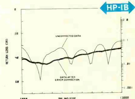
The dramatic effects of error correction are shown in this plot generated by HP's semi-automatic network analyzer system. It offers major advantages in speed, accuracy and convenience, yet costs only 50% more than a manual network analyzer.
