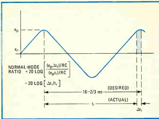
**3. Normal-mode rejection.** If the integration period is not identical to the power-line period, the system's rejection of power-line noise is adversely affected. An internal oscillator controls the integration period to  $\pm 0.1\%$ , essentially limiting normal-mode rejection to 48 dB with the expected 60-cycle line variations.
