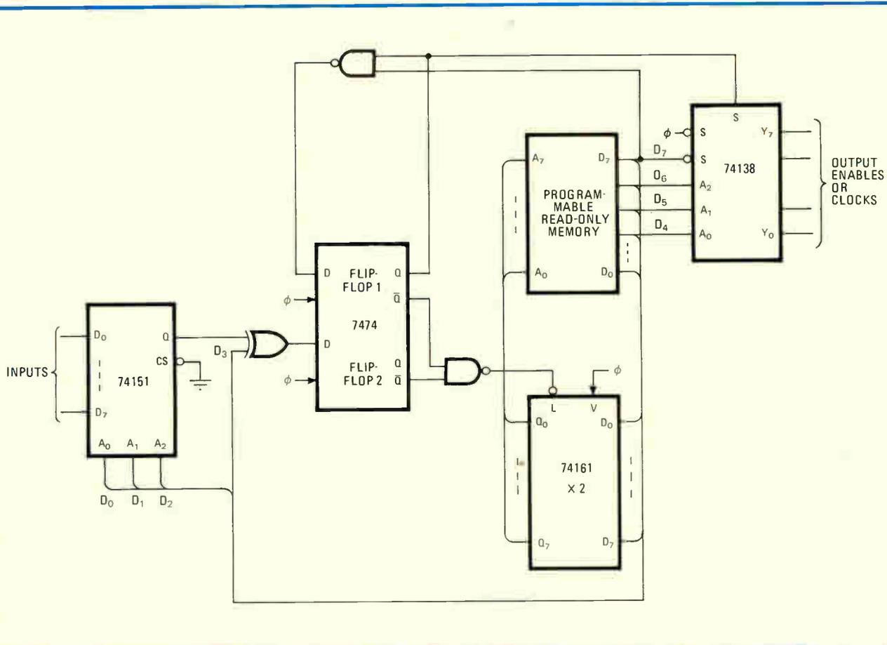
**6. Sending data.** The algorithmic state machine, a 256-word-by-8-bit variable-format design, has a microcycle time of 250 nanoseconds. It executes two types of microinstructions: store output and conditional jump, taking one and two microcycles, respectively.
