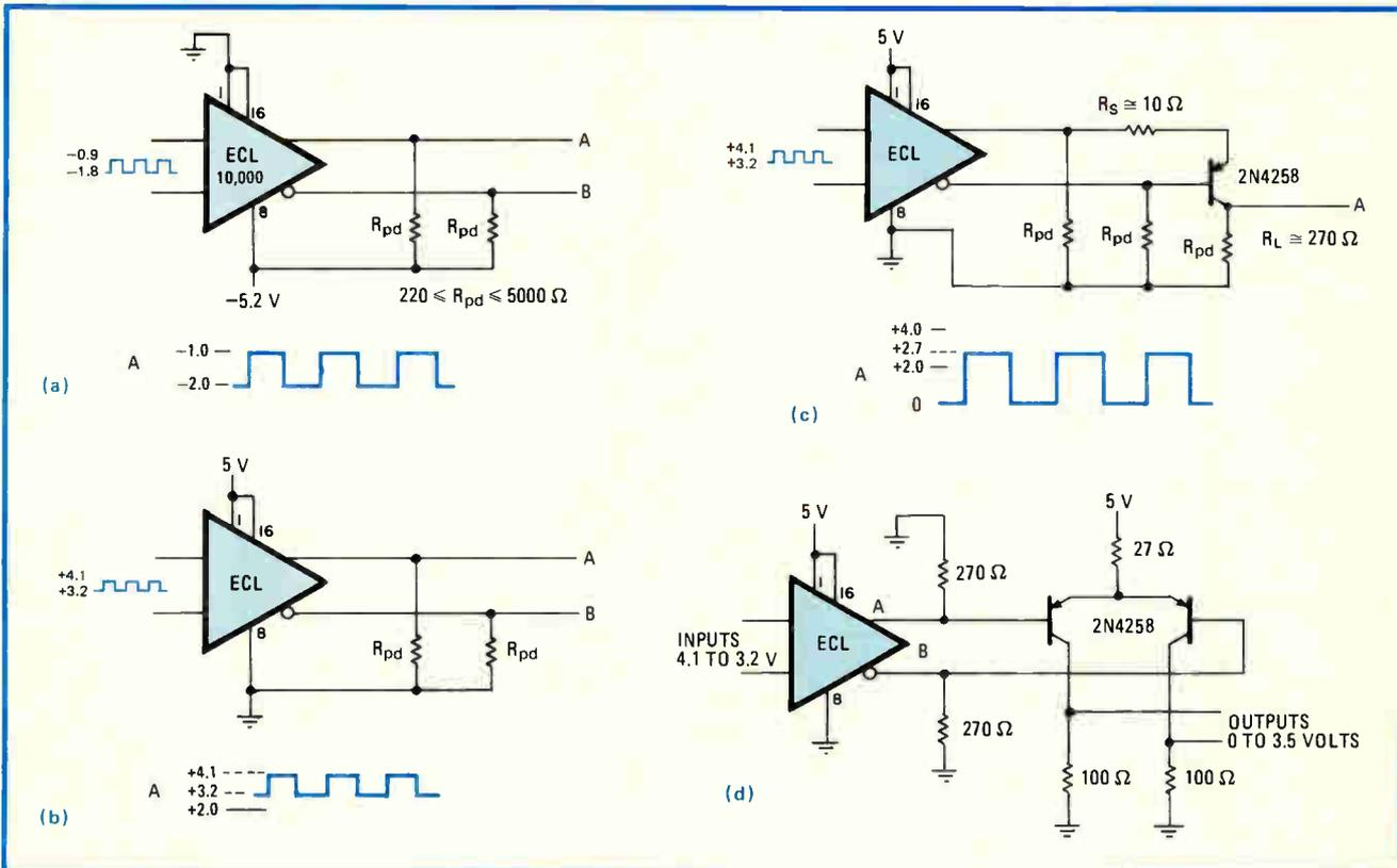
**Evolution of an interface.** Standard emitter-coupled logic is powered by at least one negative voltage, cannot drive or be driven by TTL (a). Re-biased ECL device generates positive output voltage, but not within proper TTL switching threshold range (b). Adding a transistor enables 0-2.7-V swing, suitable for TTL (c). Five-volt ECL gate and two transistors drive 100-ohm TTL loads at 0-3.5 V (d).
