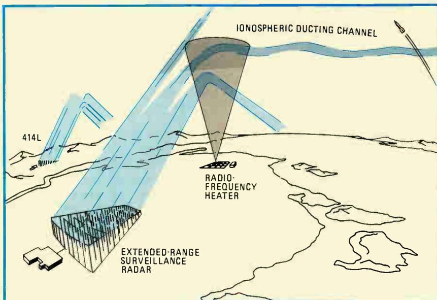
**Long-distance radar.** The tunneling or ducting effect in the ionosphere could provide a means of using long-range radar signals injected into the duct via rf "heaters."
