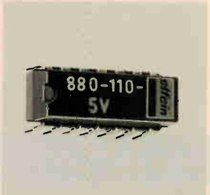
Featuring bounce-free mercury contacts, dual in-line reed relay Q43 handles 300 mA and 28 V at a 10-W switching power. Transfer resistance is 100 m $\Omega$ ; maximum deviation, 10 m $\Omega$ . Life is between  $5 \times 10^6$  and  $5 \times 10^7$  operations. Elfein GmbH, 6 Frankfurt, Wienerstr. 120, West Germany [458]
