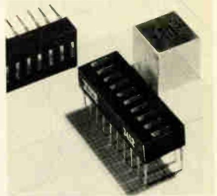
A 10-bar light-emitting-diode line array permits assembly of linear displays of any desired 10-multiple length. It is intended for applications where it is desirable to have a display output in linear analog form. ITT Components Group Europe, Edinburgh Way, Harlow, Essex, England [463]
