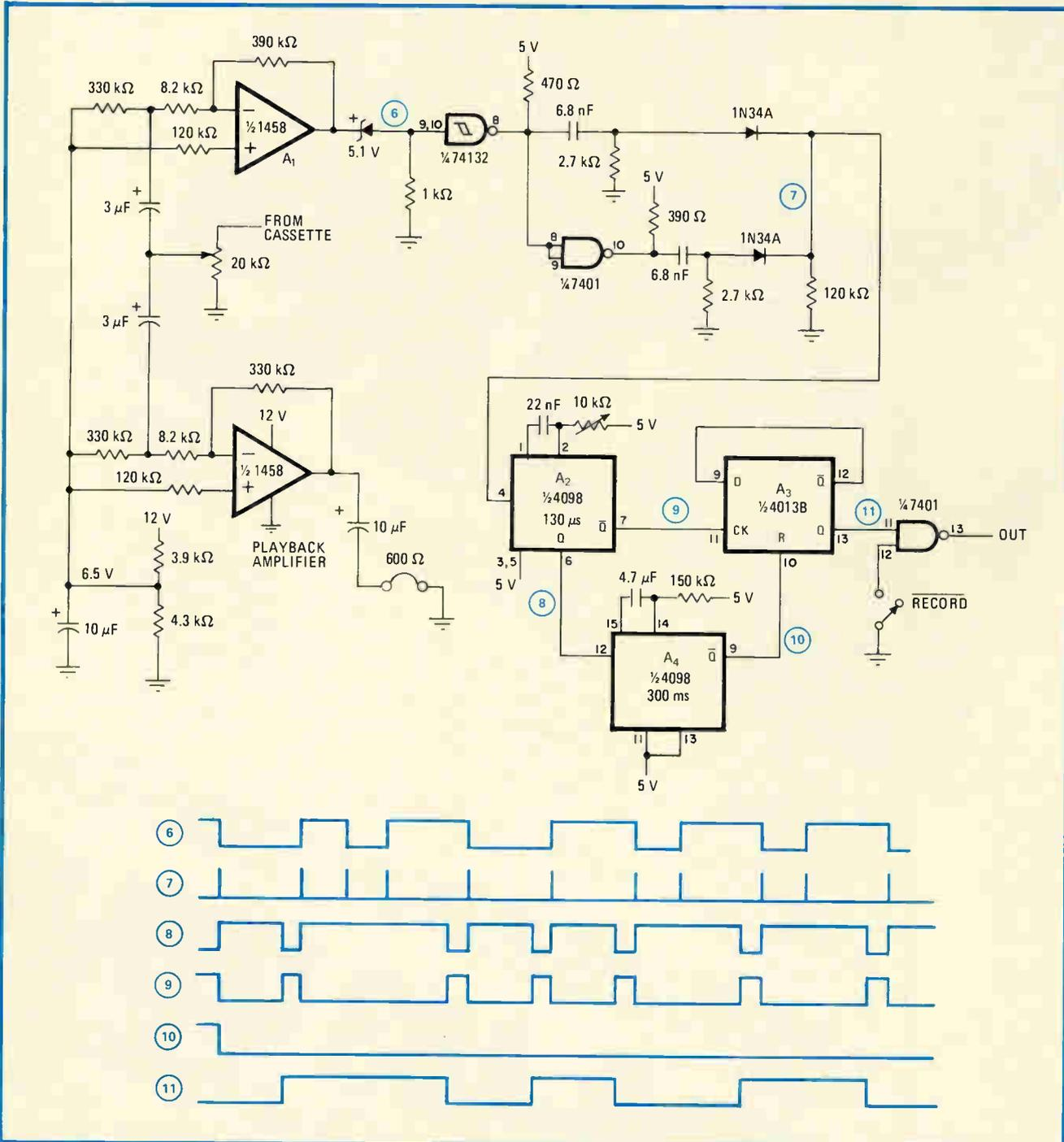
**2. Retrieved.** Data is recovered after passing through receiver interface using process essentially inverse to one used at transmitter. One-shot  $A_2$  is used to convert input signal to two complementary 130- $\mu$ s waveshapes. One waveform drives a second one-shot,  $A_4$ , which in turn resets  $A_3$ , while the other waveform drives its clock input. Timing diagram details operation. Output is a delayed version of the original signal.
