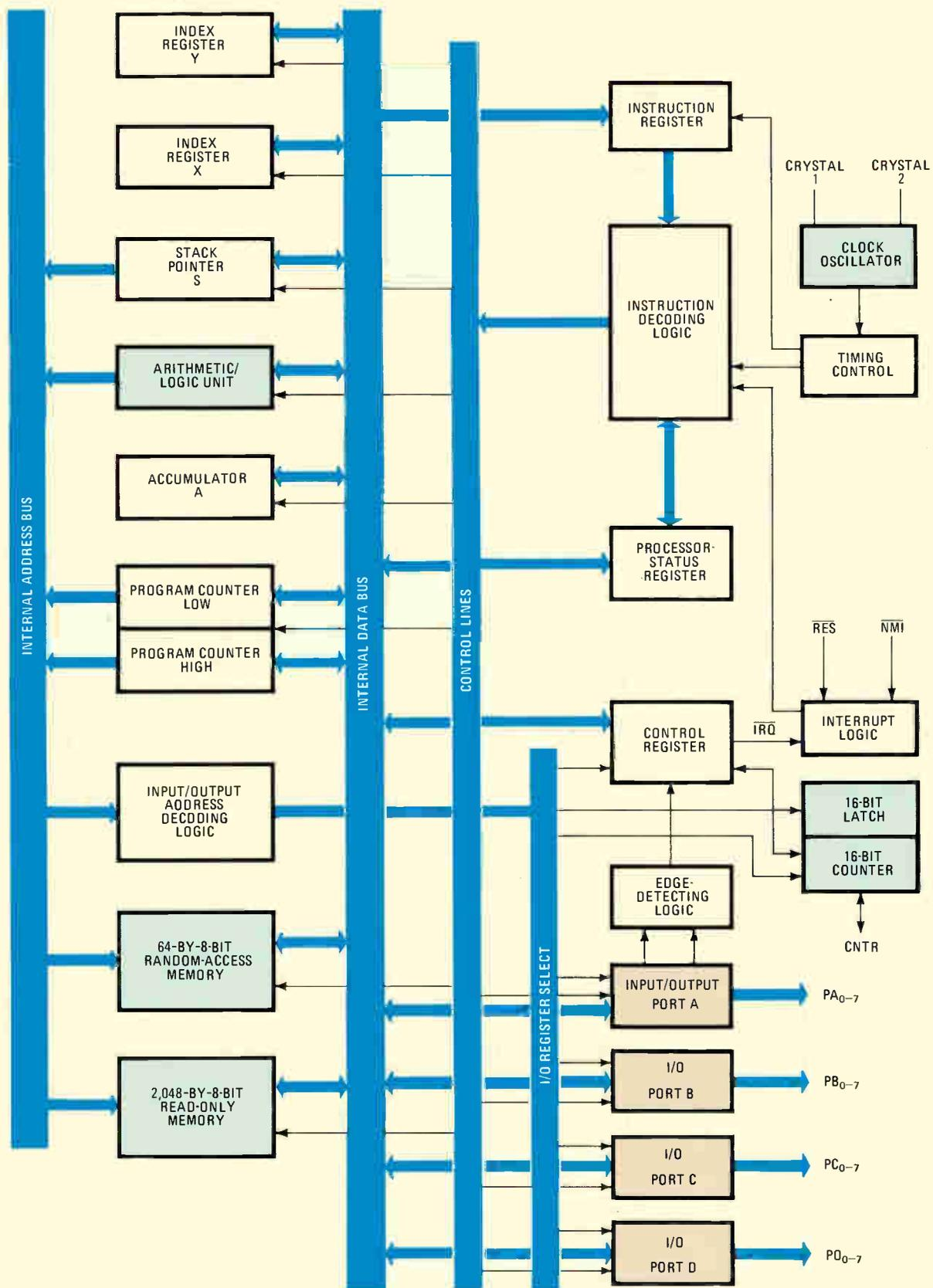
1. **One-chip 6500.** The 6500/1 contains all the makings of a computer—clock and associated timing circuits, arithmetic/logic unit and storage registers, four 8-bit input/output ports, and memory. There are 64 bytes of random-access and 2,048 bytes of read-only memory.
