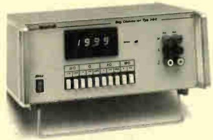
The type 300 digital ohmmeter can measure from  $10\mu\Omega$  to  $20\text{ M}\Omega$  in 13 decades. Use of a four-wire technique reduces the maximum error to 0.1%. All leads are shielded to reduce risk of false measurements. Diotechnik, 8041 Weng, Am Kirchfeld 2, West Germany [456]
