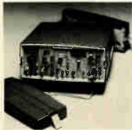
It also takes the guesswork out of checking oscillator and phase-locked loop frequencies. And, in just one second, it measures low frequency tones in the 10 Hz to 25 kHz range with a resolution of 0.01 Hz.
