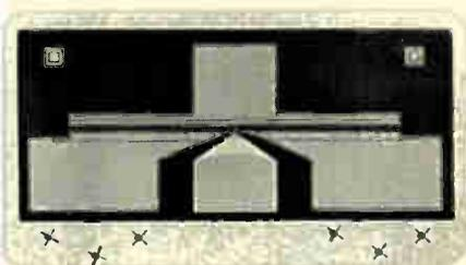
This new rugged GaAs FET, with a 1.7 dB *guaranteed* noise figure, is intended for first stages of amplifier design.
