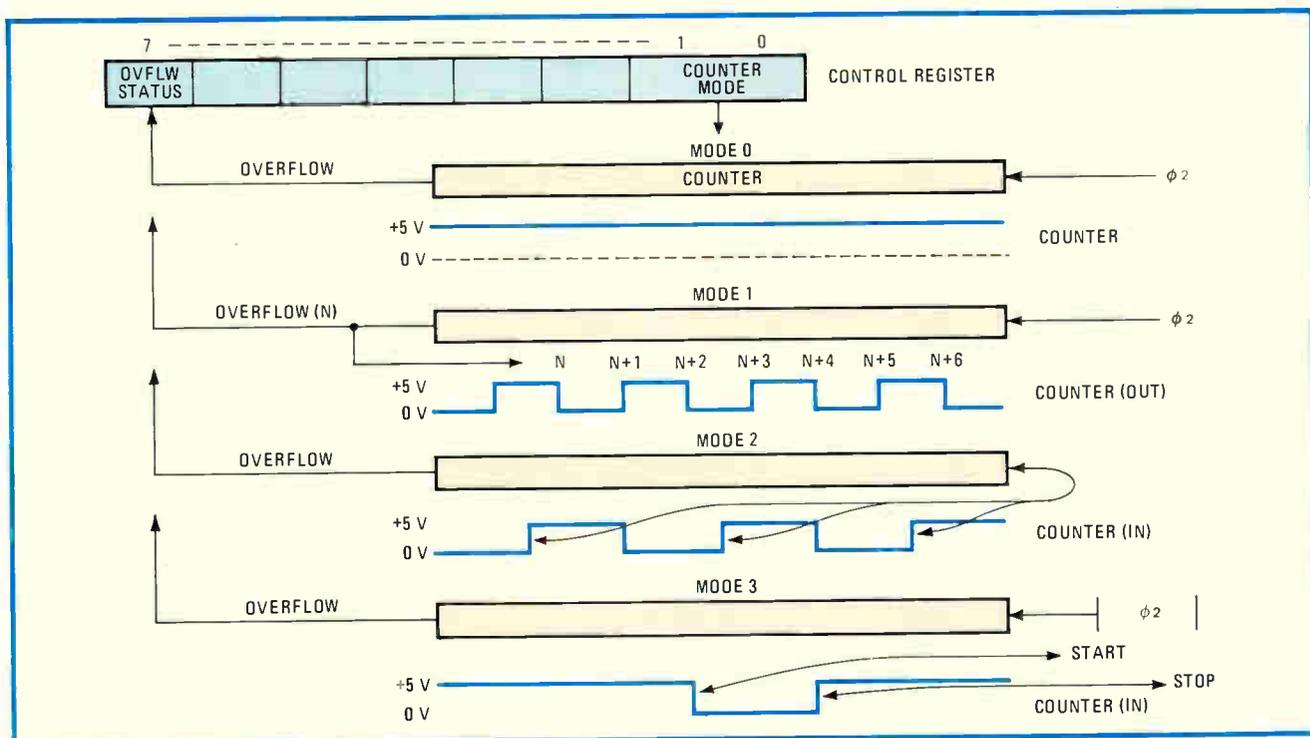
**4. The counter.** The four-mode counter is programmed by 2 bits in the control register. Modes 0 and 1 are both free-running, the latter toggling the CNTR pin on overflow. Mode 2 counts down with each rising edge on CNTR, and in mode 3 CNTR gates the countdown.
