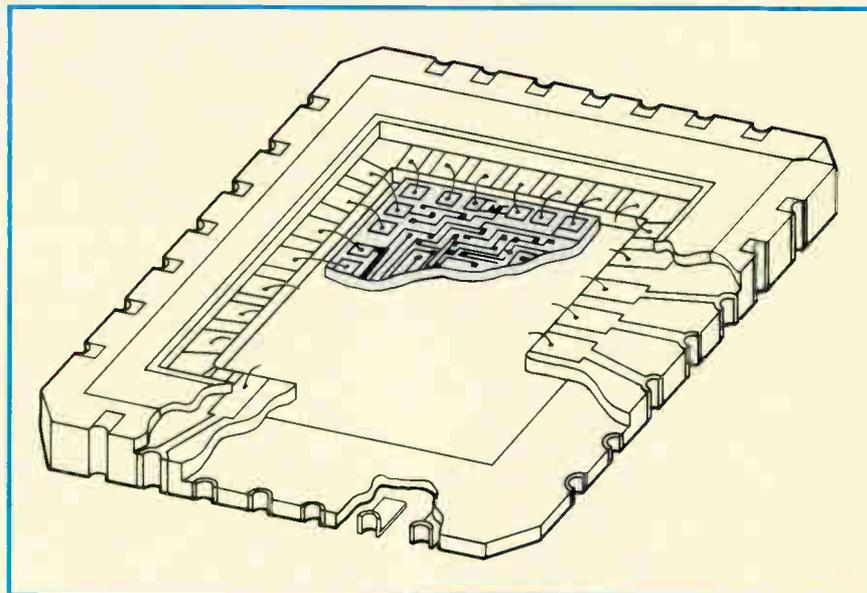
**Future package?** GE says ceramic chip carrier, seen in exploded view, works with ceramic substrates.
