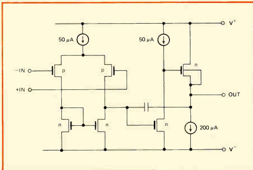
**On a chip.** In experimental LSI operational amplifier built with complementary-MOS technology, dc gain is 90 dB, slew rate is 2.5 V/ $\mu$ s, and common-mode rejection is 65 dB.
