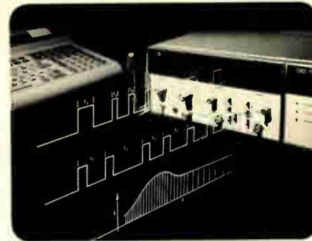
HP's 5391A Data Acquisition System is capable of over 50,000 measurements per second in frequency, period, time interval, ratio, or totalize mode.
