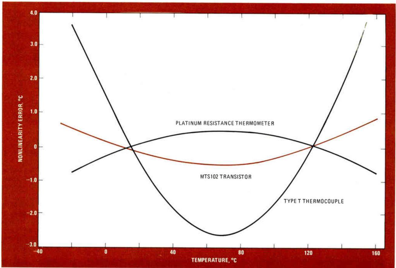
2. **In context.** Although they are inherently nonlinear, transistors perform quite admirably when compared to other devices. Between  $-40^{\circ}$  and  $+150^{\circ}\text{C}$ , the MTS102 rivals more expensive platinum resistance thermometers and easily outshines type T thermocouples.
