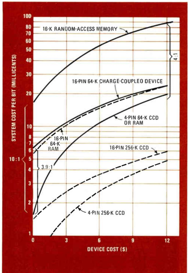
**7. Compare costs.** The system-level cost per bit drops dramatically when a 4-pin memory package replaces standard 16-pin devices. The effect is especially important as the device cost falls—the figure could be as low as a few millicents per bit for a 4-pin 256-K device.
