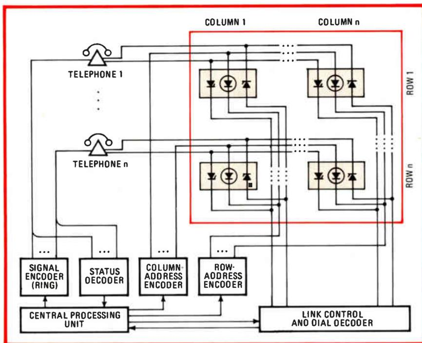
**Light switch.** Solid-state crosspoints (tinted) contain two SCRs and an LED controlled by a CPU. When the LED switches the SCRs to conduct, phone links are established.
