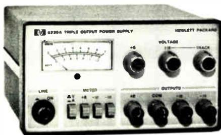
Convenient power for circuit breadboards is yours with this new three-in-one lab bench power supply.
