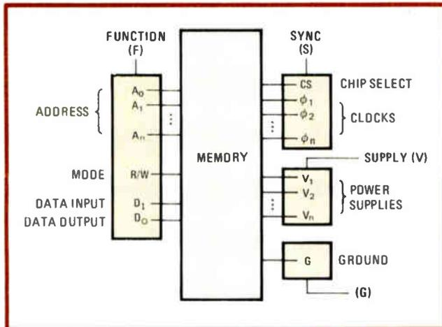
**1. Try four pins.** A dynamic memory could be built with only four pins if intelligence were added to it. Besides supply (V) and ground (G) pins, a sync pin (S) would receive clock and chip-select information, and a function pin (F) would pass addresses and data serially.
