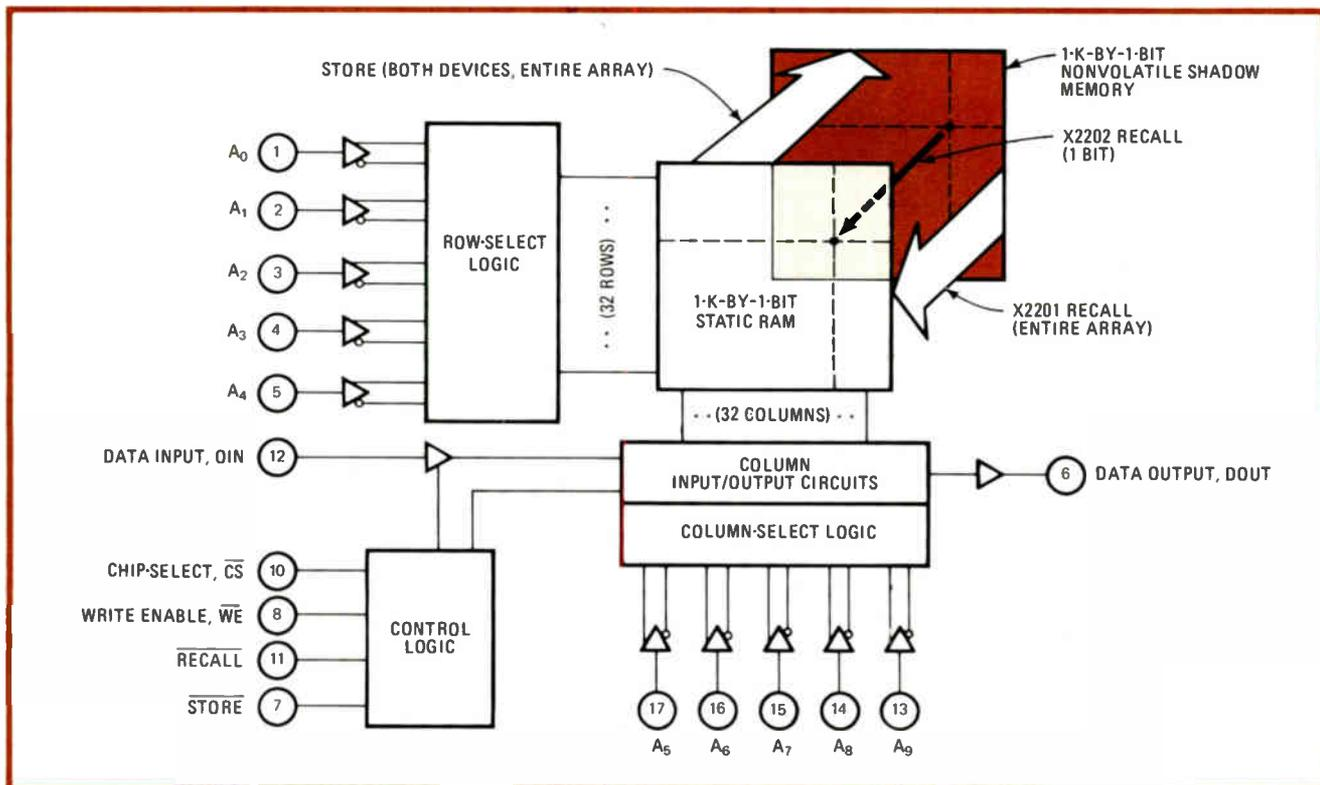
**6. The shadow knows.** The store and recall functions are depicted by arrows to and from parallel planes. Both devices come in 18-pin packages, but the actions initiated by the recall pin are different for the two devices. Pin 9 is ground and pin 18 is for power.
