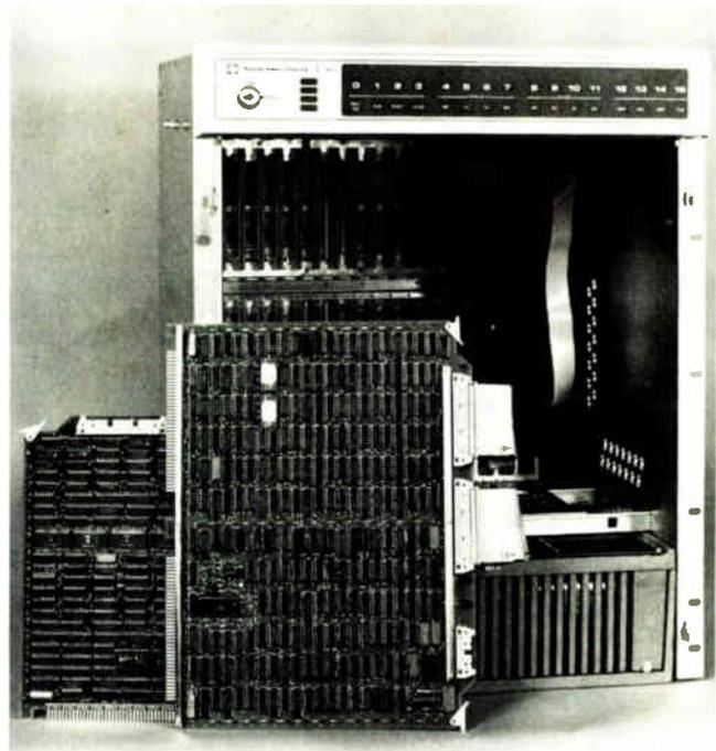
**1. Growing power.** The new 990/12 minicomputer, whose two-board central processing unit is shown here, not only runs existing software but is electrically and mechanically compatible with other computers. The 17-slot chassis has a bigger power supply, however.
