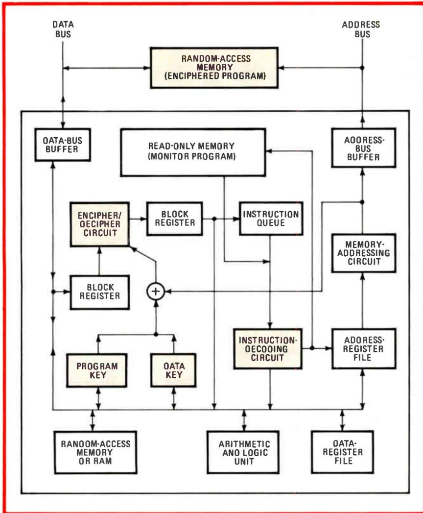
**Mum.** Instructions cannot be read out of the cryptomicroprocessor. Each enciphered instruction is deciphered as it is fetched into the instruction queue for execution.
