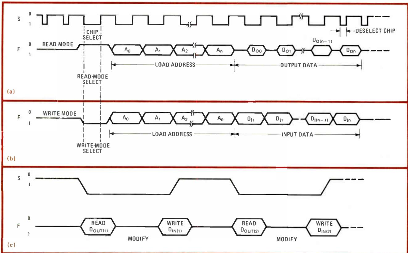
4. **Timing.** Refresh applies a narrow pulse to S while F is in the high-impedance state. To read (a), a wide pulse is applied to S, and F is high. To write, F is driven low (b). In both cases, addresses and data flow serially through F. The scheme accommodates read-modify-write (c).
