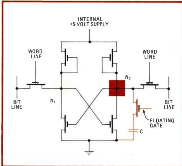
**4. Flip-flop plus.** The capacitor has no effect when the devices are used as RAMs. If the floating gate is charged,  $N_2$ 's rise is slowed by the capacitor and the flip-flop latches with  $N_1$  high. If the floating gate is off, the cell latches with the opposite polarity.
