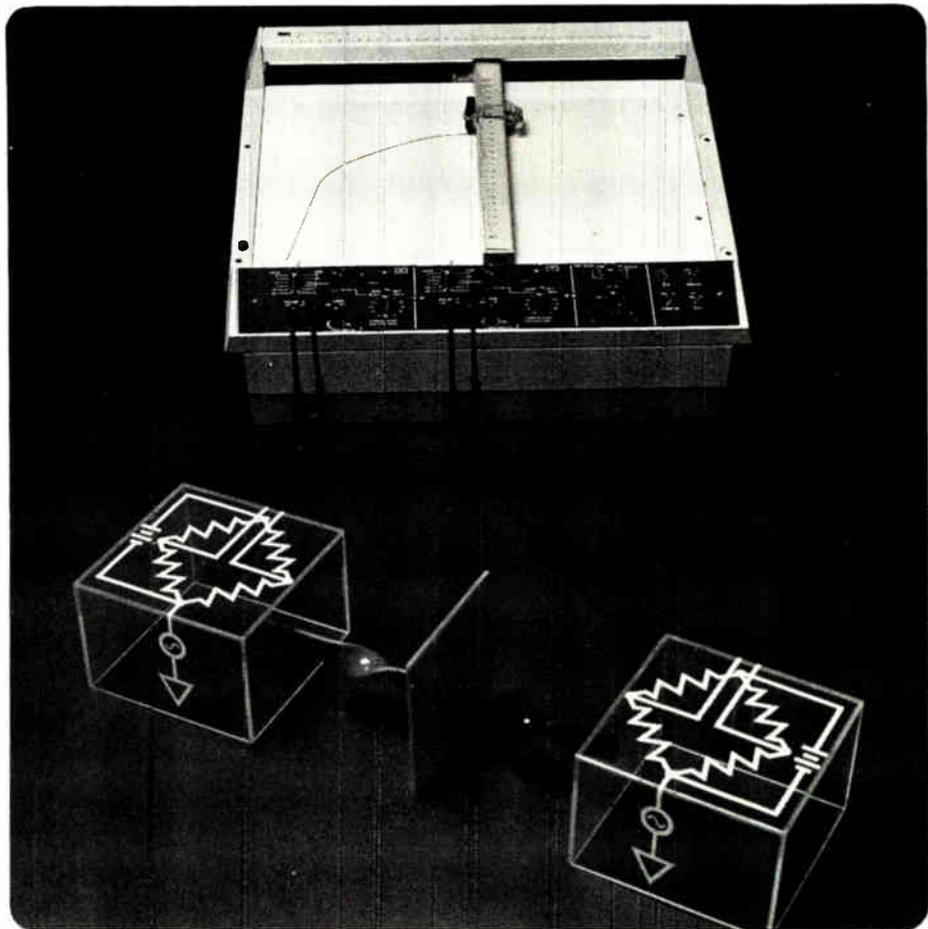
A major convenience feature, "automatic guard", is incorporated into HP's 7047A's High Sensitivity Recorder to provide you with complete freedom in connecting input terminals. Automatic guard removes the necessity for connecting the guard to maintain good common mode rejection.
