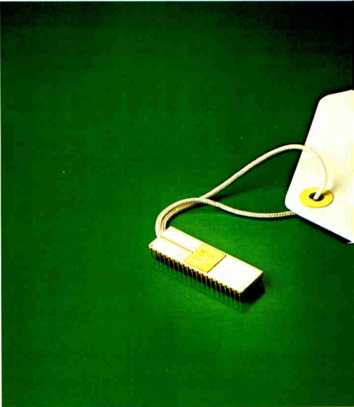
Designed and manufactured in Ireland by Analog Devices – one of 55 overseas electronic companies now operating here. A quad scope integrating 13 bit analog to digital converter for use in converting analog voltage into digital language.
