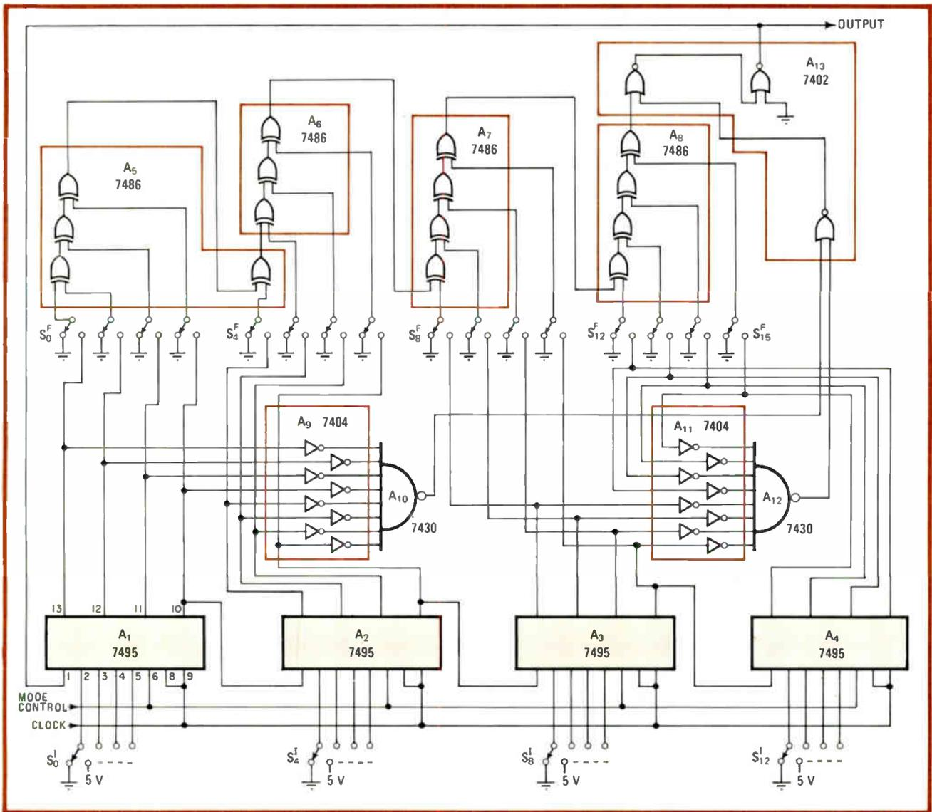
**Selection.** Switches  $S_i^F$  and  $A_5$ - $A_8$  derive suitable feedback signal so that shift register  $A_1$ - $A_4$  can generate a pseudorandom binary sequence of selectable length.  $A_9$ - $A_{13}$  detect register's all-zero state and prevent register lock-up by generating logic 1 bit to  $A_1$ - $A_4$  input during power-initialization period. Switches  $S_i^I$  initialize registers at any point in a sequence that may extend to  $2^{16} - 1$  bits.
