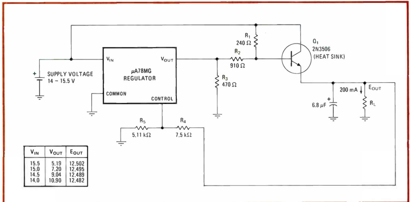
**Closer.** Outboard power transistor stage, and resistor pad  $R_1$ – $R_3$  set  $E_{out}$  to within a few volts of  $V_{in}$ , so that  $(E_{out} - V_{in})$  is below  $\mu A78$ 's dropout value.  $Q_1$  also provides increased current capacity. Table summarizes dynamic range attained for example using technique discussed in text.
