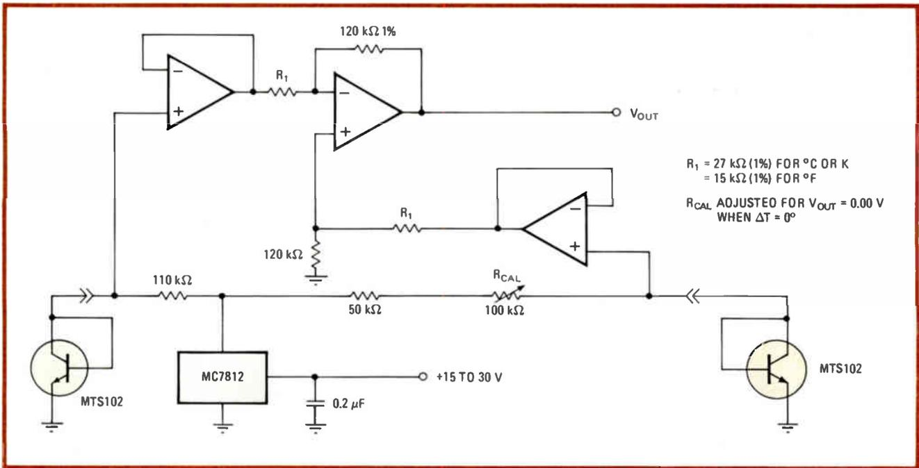
**4. Simple difference.** Differential temperature readings, frequently needed in process controlling, can be inexpensively obtained using the configuration shown. The same circuit could also be used to set an alarm when temperature stability is critical.
