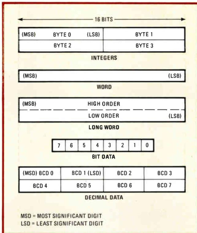
**2. Data types.** Data types associated with the 68000 include integers, words, 32-bit long words, individual bits, and decimal numbers. Integers may be represented as bytes, words, or long words; binary-coded-decimal data is packed two digits to a byte.
