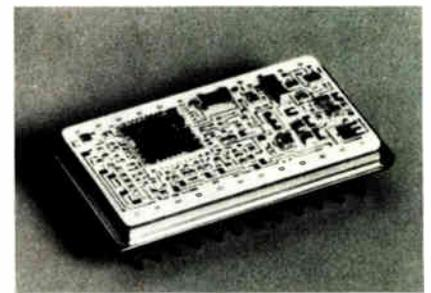
The hybrid device requires  $\pm 15$ -V power supplies. It is housed in a hermetically sealed metal case that measures 1.4 by 0.8 by 0.2 in. The price of the DAC-8528 starts at
