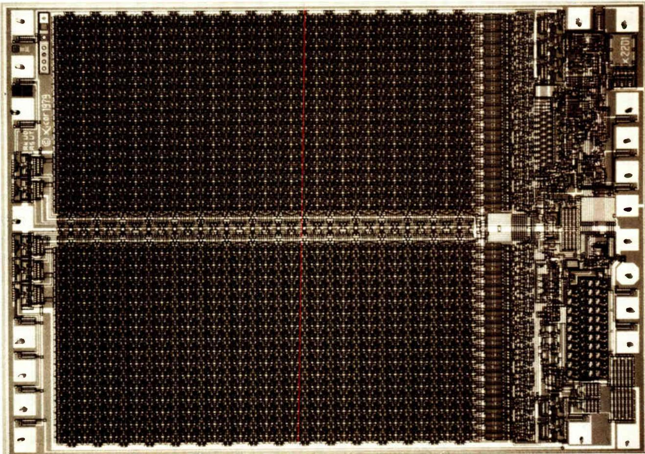
**1. Two in one.** In Xicor's memories, a nonvolatile matrix backs up a static RAM on a bit-by-bit basis. The photograph is of the X2201, wherein all nonvolatile data is restored to the RAM at once. In the X2202, also 118 by 164 mils in area, bits are brought back individually.
