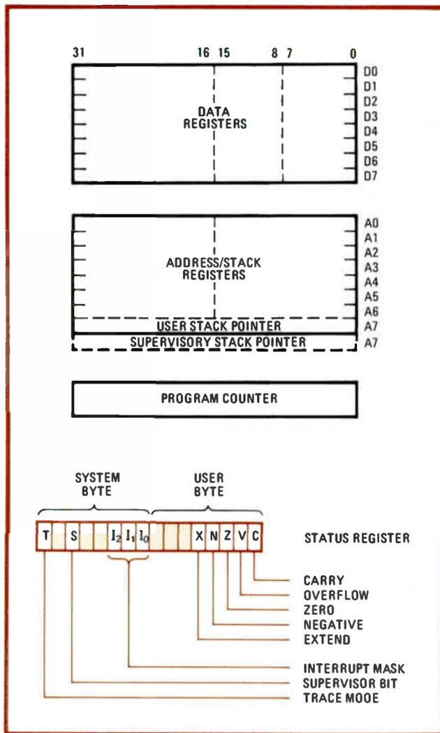
**3. Register file.** The 68000 has eight registers for data, seven for addresses, two stack pointers, a program counter, and a 2-byte status register. The device has user and supervisory states, with a stack pointer and status byte provided for each state of privilege.
