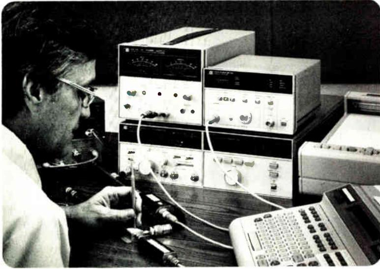
Noise figure is one of the most important specifications for amplifiers, signal conversion devices, and many system components. HP's new 346B Noise Source combined with a power meter measuring technique now offers substantial improvements in noise figure measurement. With solid state technology driving noise figure characteristics to new lows, measurement uncertainty is decreased.
