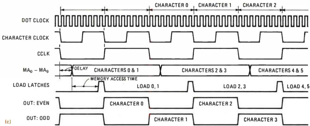
**Hardware.** Logic for increasing character rate handled by CRT controllers uses readily available gates. Circuitry for memory control (a) and data transceivers (b) adapts system for two-character fetch and display. Timing diagram (c) details system operation.
