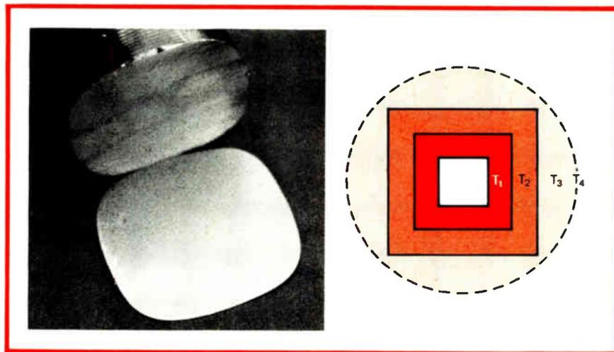
**Going square.** Motorola is getting close to square silicon ingots (left). To achieve perfect square growth, the thermal temperature zones in the melt must be square (right).
