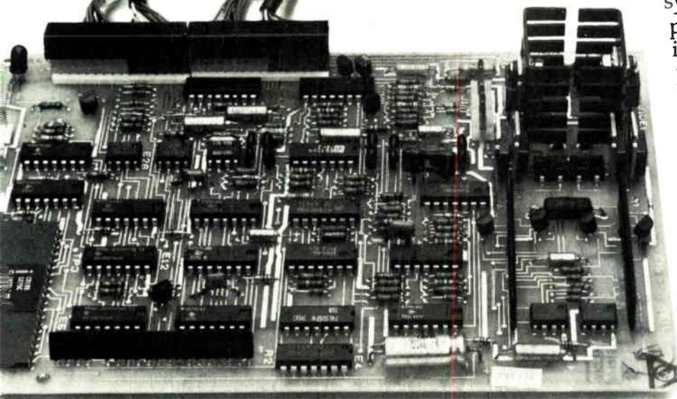
Digital's 512Kb TU58 cartridge tape subsystem. At \$562 in 100's, it's priced like a tape device. But with random-access block addressing, and EIA serial interfacing, it's like no other tape drive on the market.
