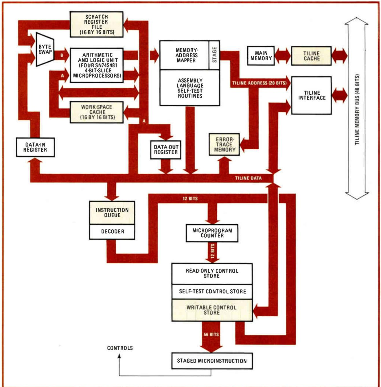
**2. Memory expansions.** Adding more memory to the 990's architecture speeds the 990/12's performance. Among the new units are the work-space cache, Tiline cache, scratch-register file, and writable control store. The error-trace memory aids diagnosis.
