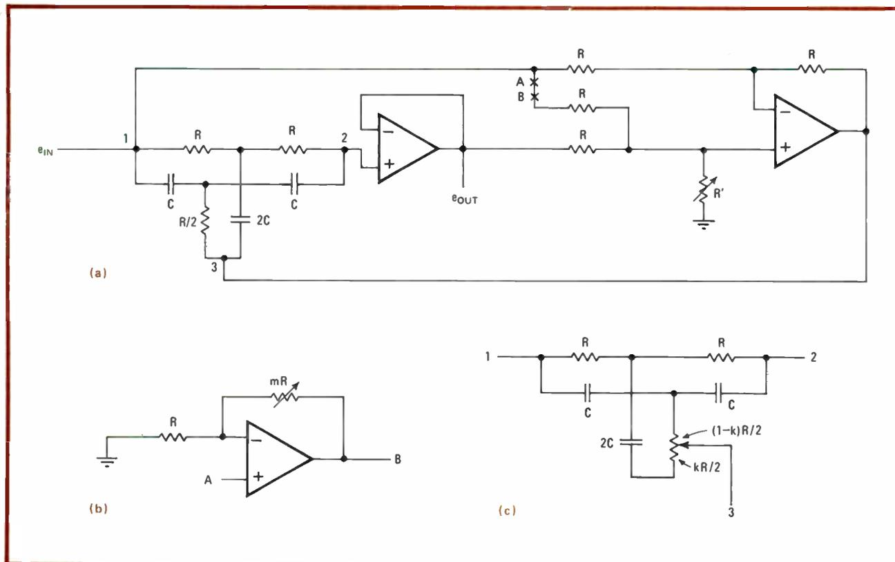
**Selection.** Parallel-T RC network simplifies design of tunable two-stage equalizer network. Delay is set with only a single control element,  $R'$  (a). Amplitude equalization or adjustment in network's center frequency is attained by adding op amp (b) and tunable RC (c), respectively.
