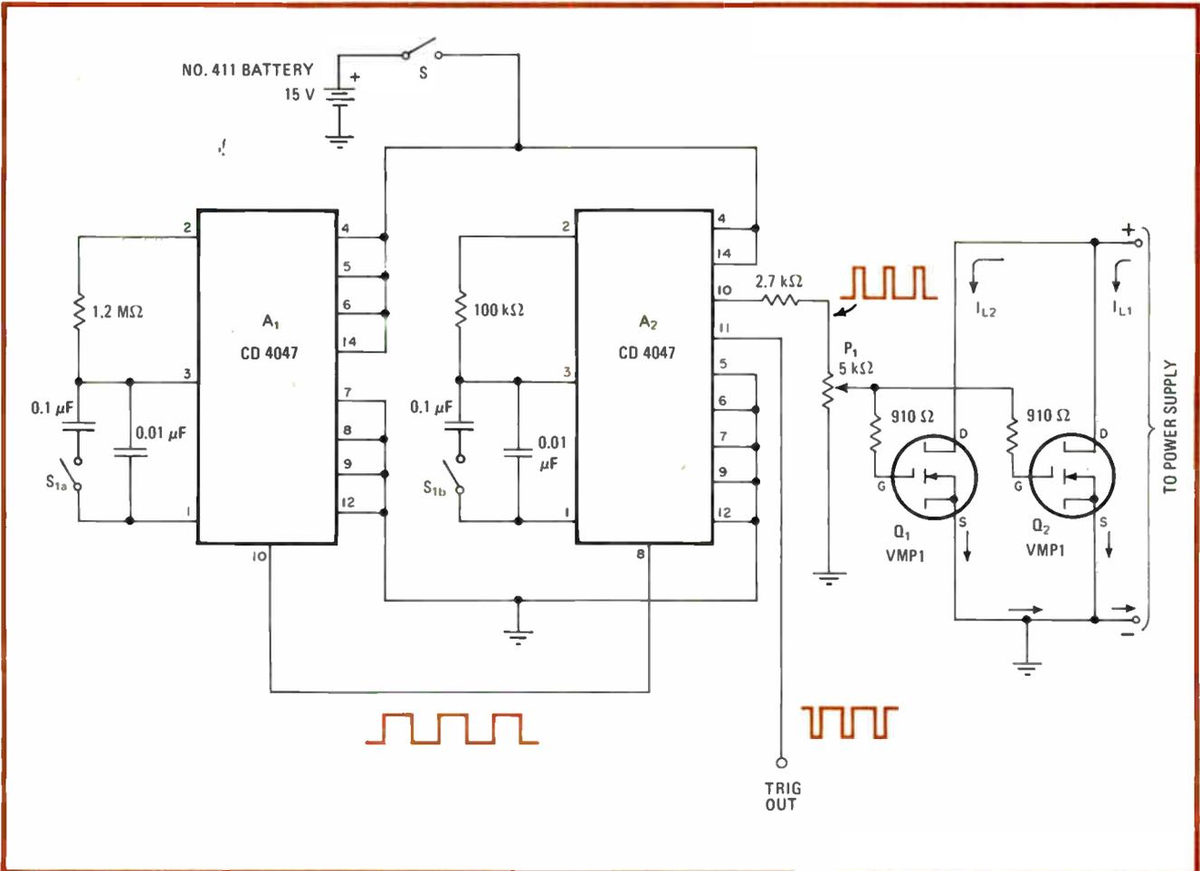
**Load dynamics.** Low-cost tester, with aid of scope, finds transient response of power supply by ordering periodic increase in supply current to simulate load changes.  $A_1$  and  $A_2$  set frequency and width of switching waveform.  $Q_1$ – $Q_2$  sink current proportional to setting of  $P_1$ .
