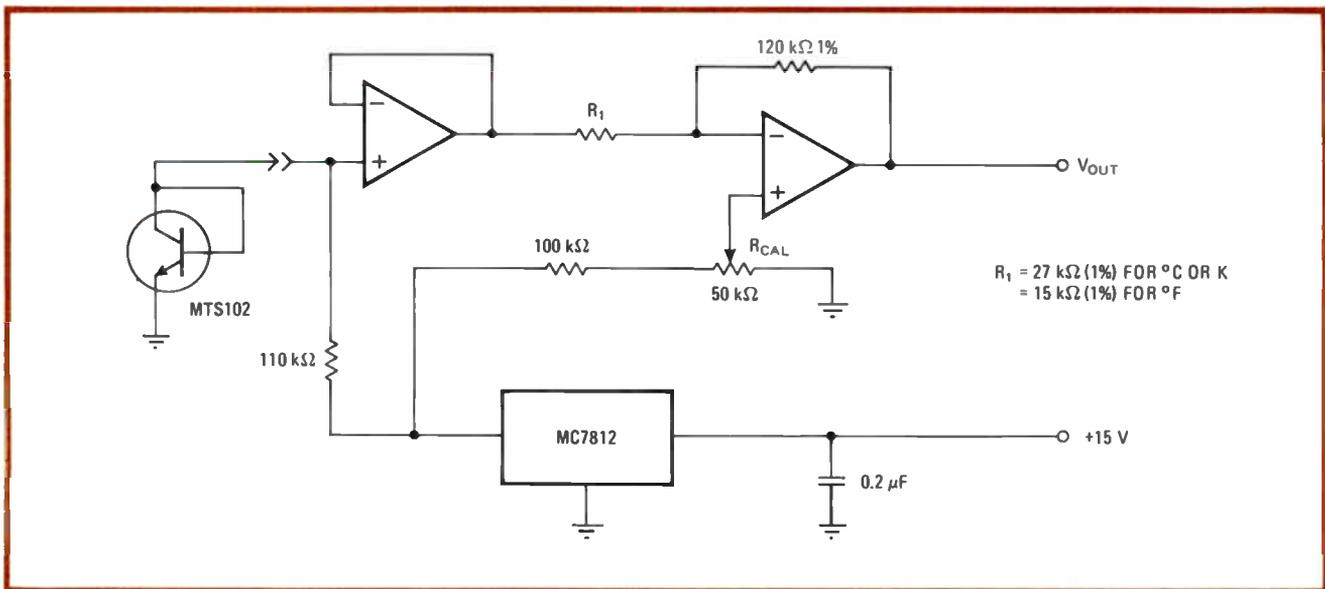
**5. Even simpler.** A single transistor version of the circuit shown in Fig. 4 requires even fewer components. Since the transistor itself is inexpensive, it and others like it can be left in place and the remaining circuitry built into a portable meter.
