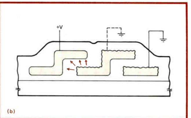
**3. Held and let go.** The program/erase line is raised, coupling the floating gate to a positive potential. In (a), the gate is charged as electrons tunnel through oxide from the first-level asperities. The floating gate potential is lowered in (b), and electrons tunnel off for erasure.
