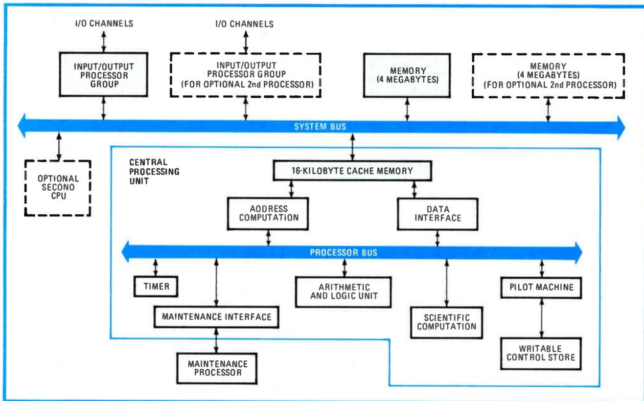
**Mass transit.** CII-Honeywell Bull has opted for a bus-oriented architecture for its new line of computers, which is compatible with the three previous lines of its predecessor companies. The central bus can handle data-transfer rates of up to 36 megabytes/s.
