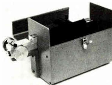
nal 12-V dc source. The dynamic range of the instrument is over 60 dB. Unterminated fibers of various sizes may be measured; if they are terminated, adapters for all major connectors may be ordered.
