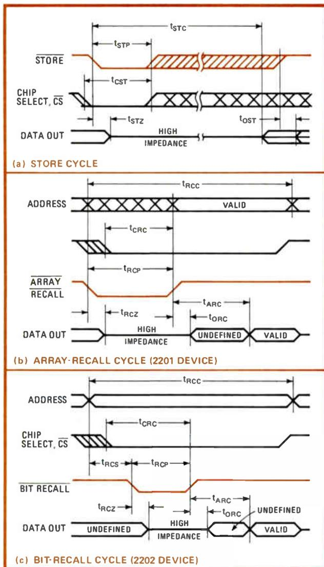
**7. Shadow timing.** Storage-function timing is shown in (a), the 2201's array-recall timing in (b), and the 2202's bit-recall timing in (c). To make RAM data nonvolatile, only one pin is signaled after the device is slated. The same is true of bringing data back into the RAM.
