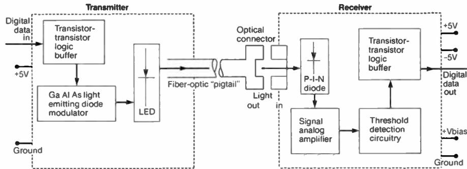
arsenide LED modulator forms the heart of the transmission module.
