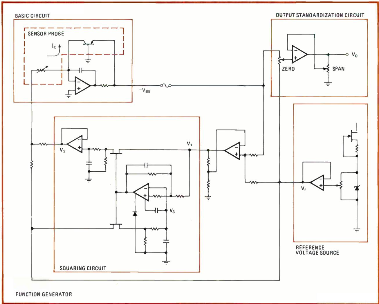
**3. High accuracy.** To obtain high performance, the collector current of temperature-sensing transistors can be varied in accordance with temperature (reflected by base-emitter voltage) raised to some power. The squaring circuit shown performs this function.
