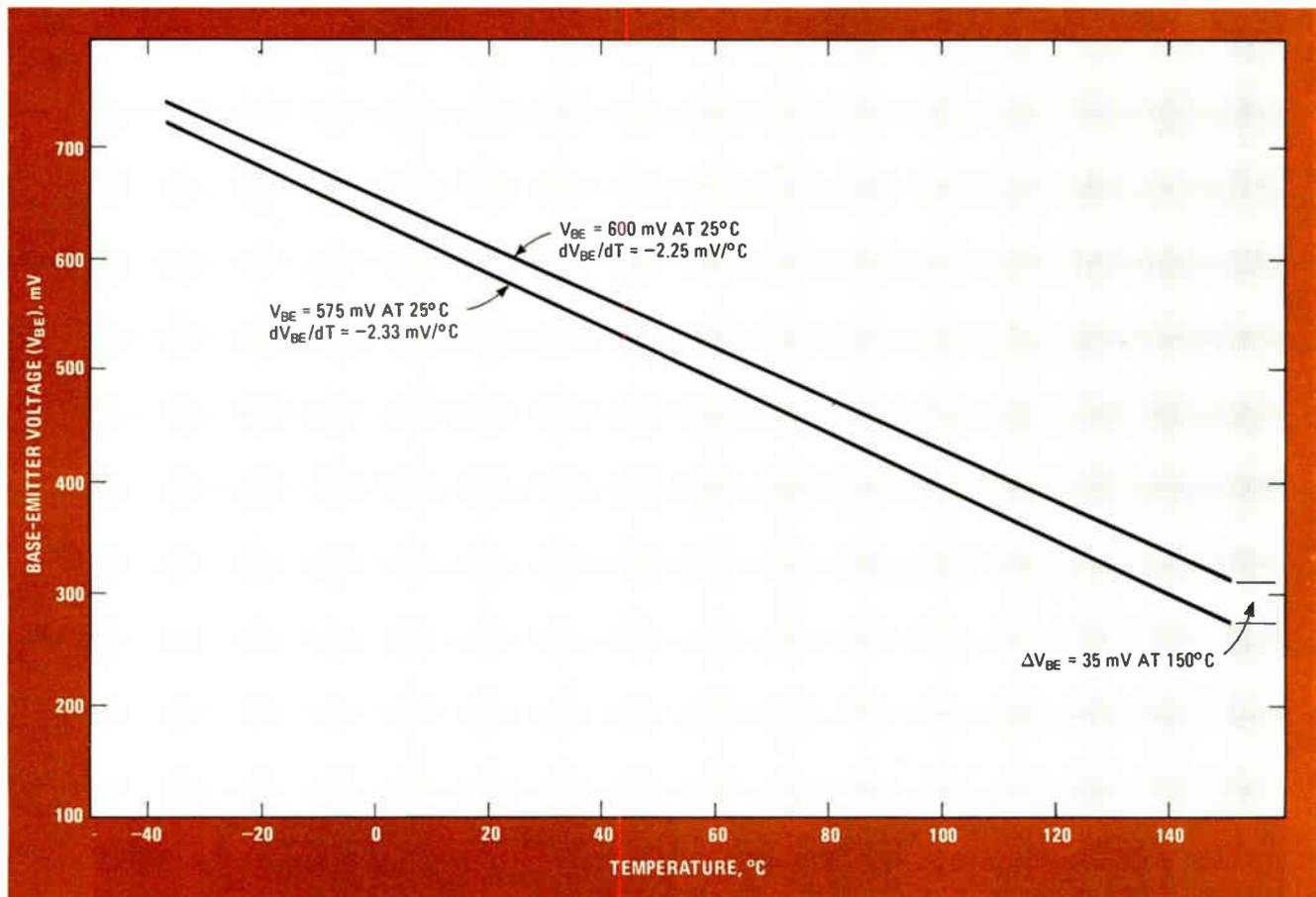
**1. Single-point prediction.** When transistors have the same dc gain, their performance across a range of temperatures can be predicted by measuring their base-emitter voltage at a specific temperature. Variation in  $V_{BE}$  can result in large errors.
