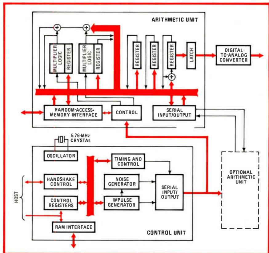
**Synthesizing speech.** Working with a host microprocessor, Telesensory Systems two-chip digital signal processor produces speech from phonemes encoded from a text.
