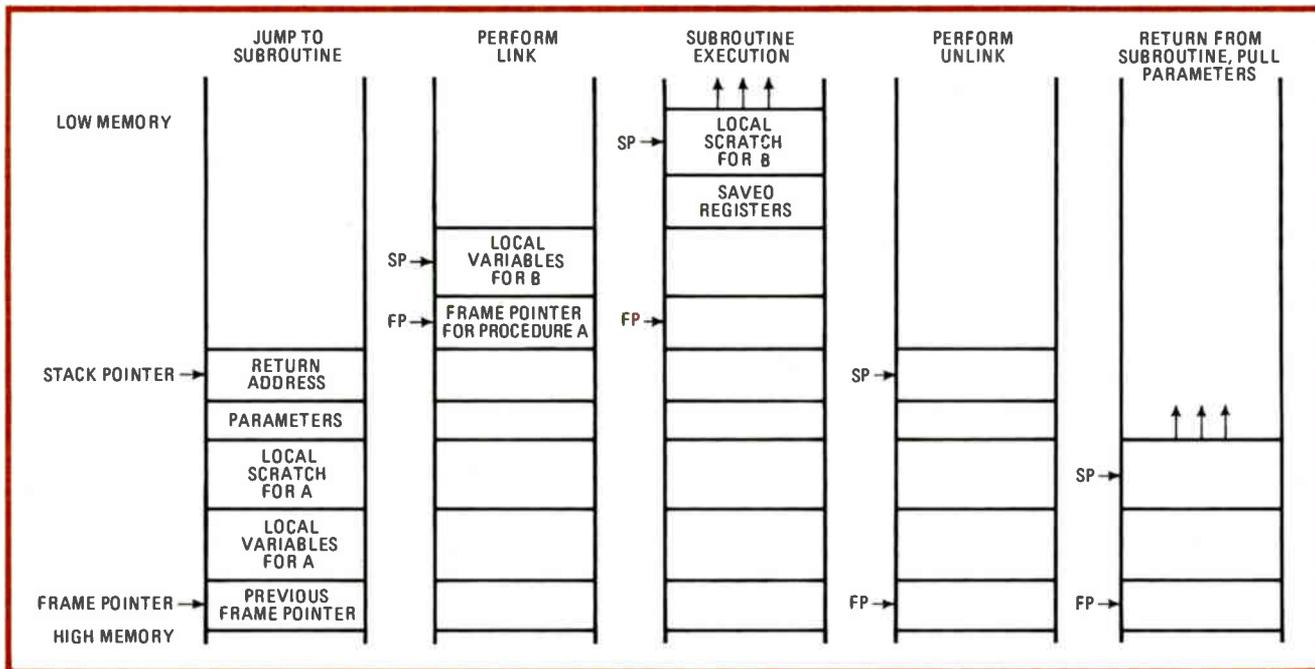
**4. High-level assembly.** Some assembly-language instructions for the 68000 do so much they could be termed higher-level instructions. The link-stack and unlink-stack commands, for example, allocate and deallocate, respectively, local storage for procedure calls.
