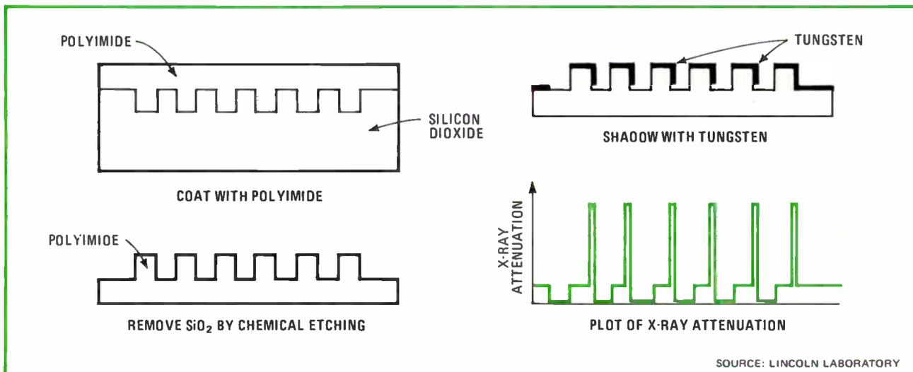
**Shadowed.** These are the steps in fabricating a shadowed polyimide X-ray mask with a square-wave profile. The SiO<sub>2</sub> square-wave structure is made by reactive ion etching. Masks of this type, combined with a carbon K X-ray source, have exposed 200-angstrom lines.
