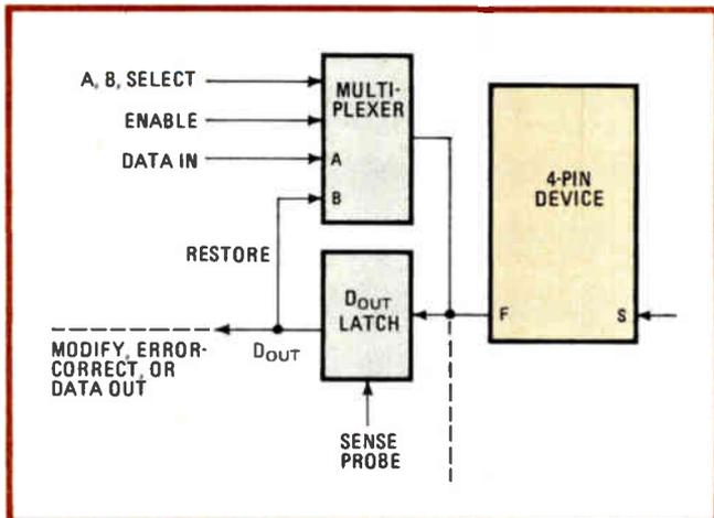
**5. External support.** The support circuits to drive the F pins are relatively simple. A multiplexer allows either addresses or data to flow over an F-pin line, and a latch receives data flowing out of the line. Select signals would derive from a master control board.
