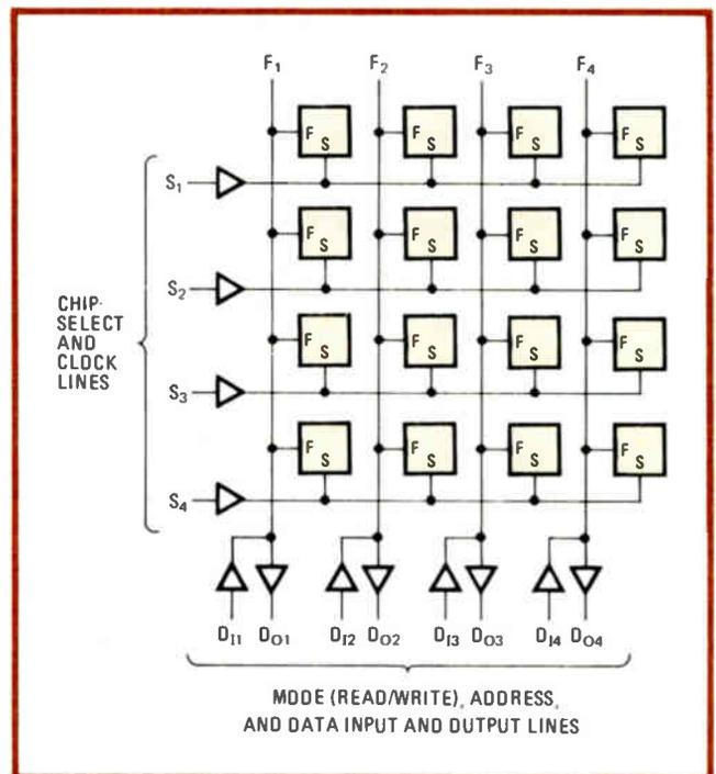
**2. Easy layout.** A four-pin memory would make circuit-board layout a cinch. On a square grid F lines run vertically to stack bit-wide blocks into words, while S lines run horizontally to chip-select the words. For clarity, supply rails V and G are not shown.
