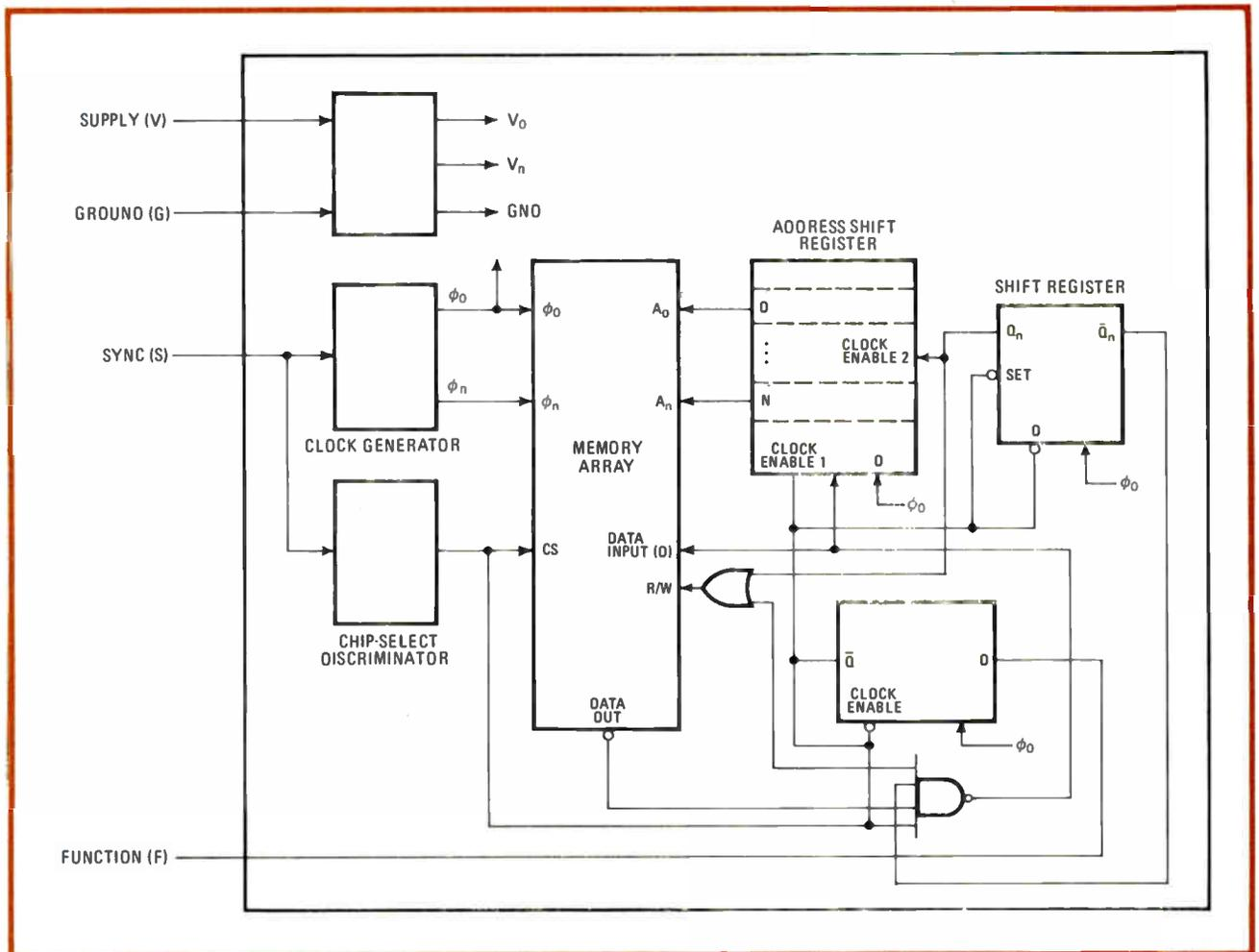
**3. Added intelligence.** The additional interface circuits for the four-pin memory might appear excessive, but would actually occupy little additional chip area. The reason is that the dozen or so bonding pads and associated driver circuits of conventional chips are eliminated.
