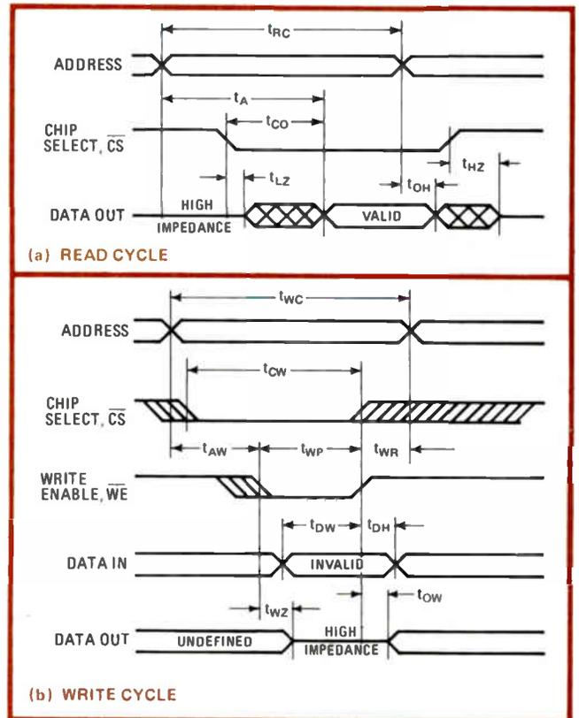
**5. Read/write RAM.** These timing diagrams apply when the Xicor devices are operated as standard static RAMs. Part (a) is for reading and (b) is for writing. Timing is almost identical to that of 2102-type 1-K-by-1-bit memories, and access time is less than 250 ns.
