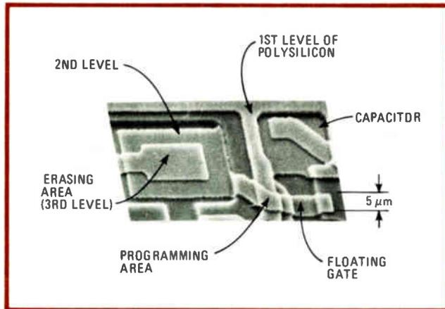
**2. Closer look.** A scanning electron microscope has captured most of a Xicor cell. It uses n-channel MOS technology and three polysilicon layers. The second forms a floating gate that collects and releases charge as the nonvolatile array is programmed and erased.
