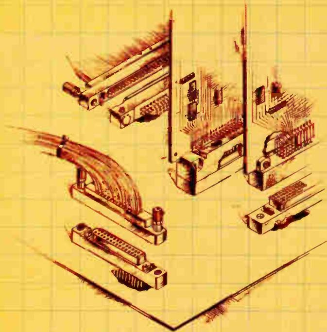
A low mating force connector with up to 400 contacts. 4 body styles. 3 contact variations with options. Superior electrical characteristics and long mechanical life. That's flexibility! And Bendix has one for your high-contact needs. The Brush Connector. Here's what you get.
