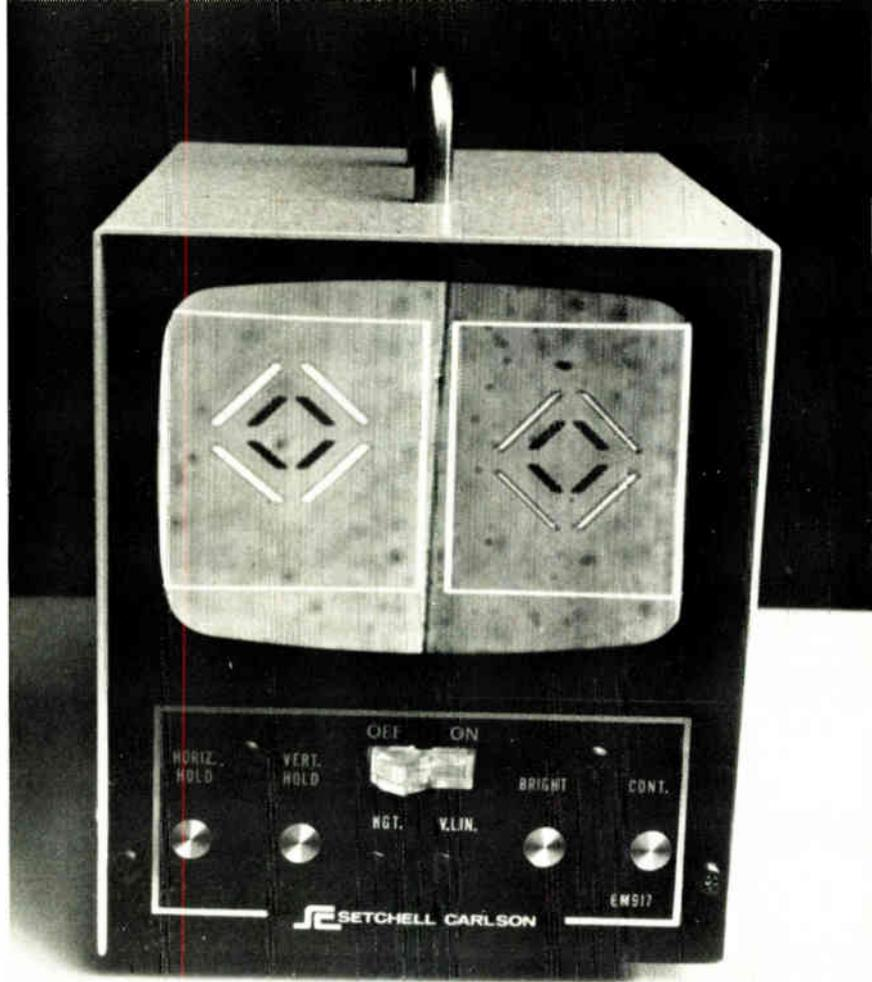
**Automatic alignment.** Pattern recognition and edge detection permit Perkin-Elmer system to get 0.25  $\mu\text{m}$  alignment accuracy on projection aligners also made by the company.
