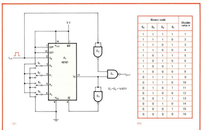
**Binary breakup.** Single counter and three gates simplify design of variable-modulo divider (a). Binary switches  $S_1 - S_4$  set counter to 16 - n, where n is desired divider ratio (b). Output of gate  $G_1$  is a pulse with a frequency equal to  $f_{out} = f_{in}/n$ , for  $1 \le n \le 16$ .
