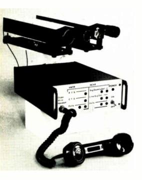
Many uses. A GaAs laser unit, designed for secure data transmission over fiber-optic cables, is serving as a line-of-sight teletype-writer link. It also can carry voice traffic.
