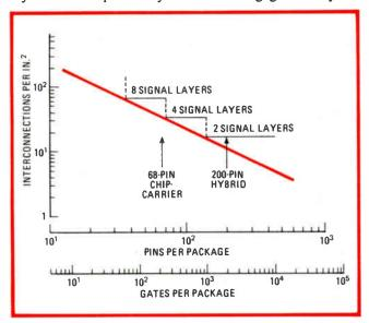
7. Circuit density. Four signal layers on the board are sufficient when 68-pin chip-carriers with leads on 50-mil centers are used; a simpler two-layer board requires the use of costly 200-pin hybrids. The chart is based on a board with an array of 25,000 gates.
