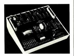
dual in-line package switch. Computer output can be converted to analog signals for meter display or motor speed control. The on-board analog-to-digital and digital-to-analog converters can also be used to bring in or send out control voltages directly on breadboarding terminals.
