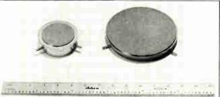
Systems for MBE growth over one and two inch wafers
