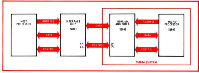
4. Complete system. The S6894 two-chip data-encryption and -decryption subsystem can be connected to a host processor through an S6821 interface chip or its equivalent. Encryption time can be as low as 5.5 milliseconds.
