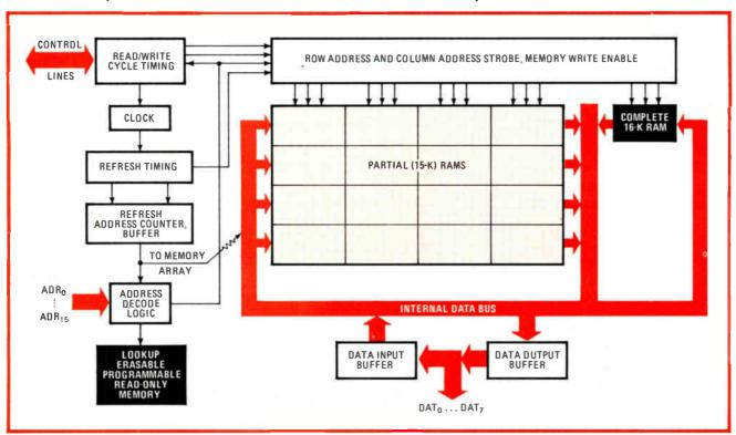
1. Partial devices, full capacity. A memory with 32 kilobytes of storage can be built with 16 15-K partial dynamic RAMs by adding a 16-K E-PROM and a full 16-K RAM. The E-PROM stores failed locations in the partials; the extra RAM provides substitutes for those locations.
