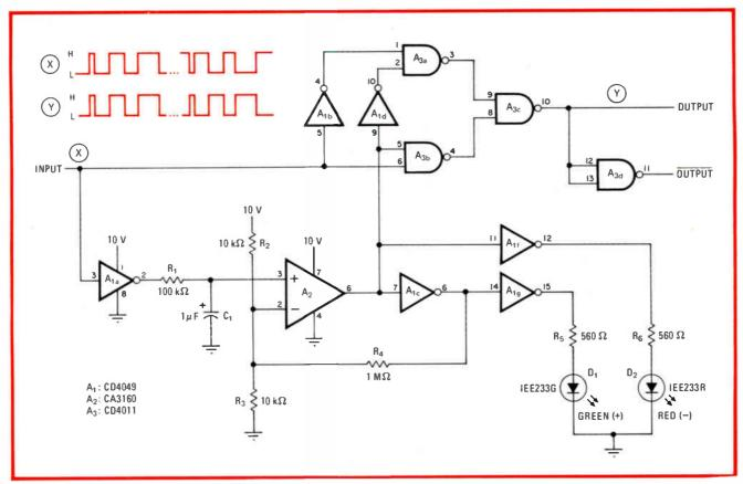
**Switch.** Three-chip driver accommodates both positive- and negative-going input signals, converting them both into positive-going output. Circuit propagates positive-going signals having a duty cycle less than 50% through to the output while inverting all other signals.
