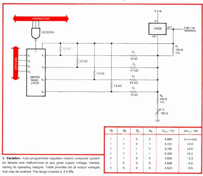
by pnp transistors much as they are in Fig. 1. Note that the resistors are in a binary-weighted proportion. To decrease  $V_{out}$  by 2%,  $Q_4$  is brought low from its normally high state. To increase  $V_{out}$  by 2%,  $Q_1$  is set high and  $Q_2$ – $Q_4$  is kept low. The range of voltages that may be ordered up is displayed in the chart.
