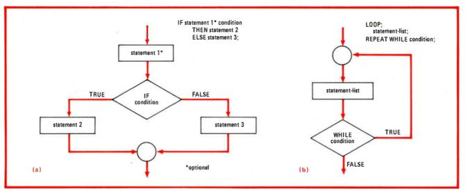
1. Structures. Two of the most beneficial of SMAL/80's structured control constructs are the if-then-else (a) and the loop-repeat-while (b). In the latter, statement-list refers to one statement or a group, and it may include next or break statements for exit control.
