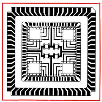
**6. Eye to the future.** A four-chip hybrid on a simple one-layer substrate not only is an immediately cost-effective package for SSI chips that lets all leads be directly wired to the board, but can also be replaced by one gate-array chip later without board redesign.
