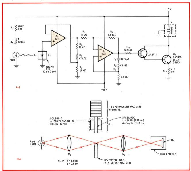
**Rising rotors.** Levitator circuit (a) suspends 1-in. steel spheres up to 2½ millimeters off reference surface. Optical arrangement (b) sets object distance. Details of levitation coil construction are outlined. Permanent magnets set ultimate levitation range.
