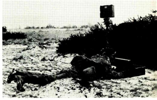
On display. British radar manpack, in development, features clear, continuous display of all moving targets within a broad azimuth sector. Range and bearing can be displayed digitally.
