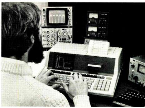
**Compact.** The typewriter-sized HP-85 personal computer for business and technical users has a high-resolution CRT display, thermal printer, and cartridge tape drive—all built in.
