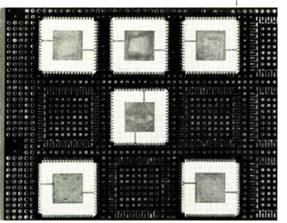
2. Standards in harmony. Chip-carriers with 50-mil lead spacing can be mounted on multilayer printed-circuit boards with the standard 100-mil grid of vias using a simple wiring pattern. Carriers with 40-mil spacing complicate wiring, requiring more board layers.
