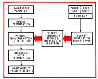
**2. Best choice.** The 16 subkeys required for the NBS data encryption standard are computed each time a new 56-bit data-encryption key is entered in the system. This approach minimizes the encryption time but uses most of the random-access memory.
