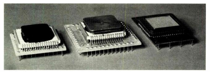
**4. DIP-like chip-carriers.** An adapter that makes a chip-carrier with leads on 50-mil centers look to the printed-circuit board like a DIP with leads on 100-mil centers can simplify the problem of designing boards for mixed arrays of SSI chips in DIPs and LSI chips in carriers.
