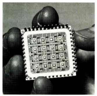
**5. Hybrid in carrier.** This multilayer, multichip hybrid is mounted in a 48-lead chip-carrier; it takes the place of 16 SSI chips in DIPs. The hybrid can be reworked quickly in response to system redesign, and leads to a dramatic drop in the number of boards in a system.
