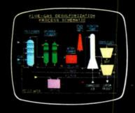
The FS 2500°: A dedicated display generator designed specifically for process control applications. Many special features for easy operator interaction.
