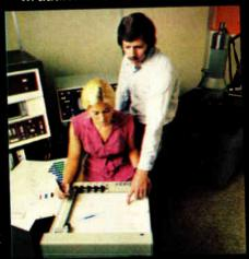
7220 Plotter, HP also offers the low cost Model 7225A, an A4 (812" x 11") high quality plotter with RS-232-C hardwire connection. And it uses the same plain-talking HP-GL language. A plug-in module customizes the plotter to your computer, desktop computer or intelligent instrument system.
