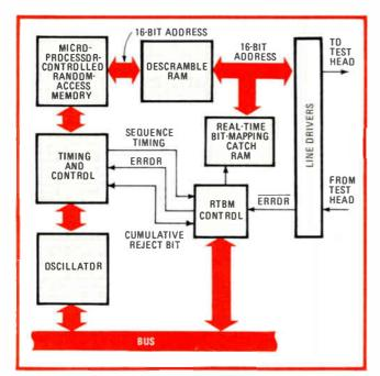
2. RTBM. Adding real-time bit-mapping hardware—the catch RAM and control logic board—to the J387 test system enables thorough testing of partials. At the control logic's command, the RAM stores 1s in locations corresponding to failed bits in memory under test.
