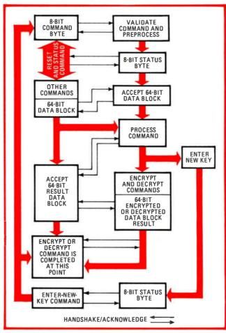
3. Data flow. All input/output signal transfers are individually acknowledged by handshake signals in the S6894 data-encryption system. The set will not proceed to the next step in an operation unless each step is acknowledged by the host processor.
