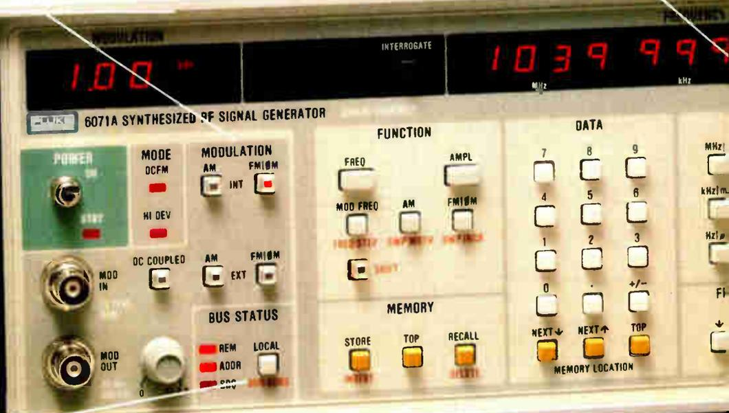
*Built-in, easy-to-program IEEE-488 interface ties the signal generator capability of the instruments to the power of automated system control. Talk/listen capability provides "learn" and "teach" modes*
