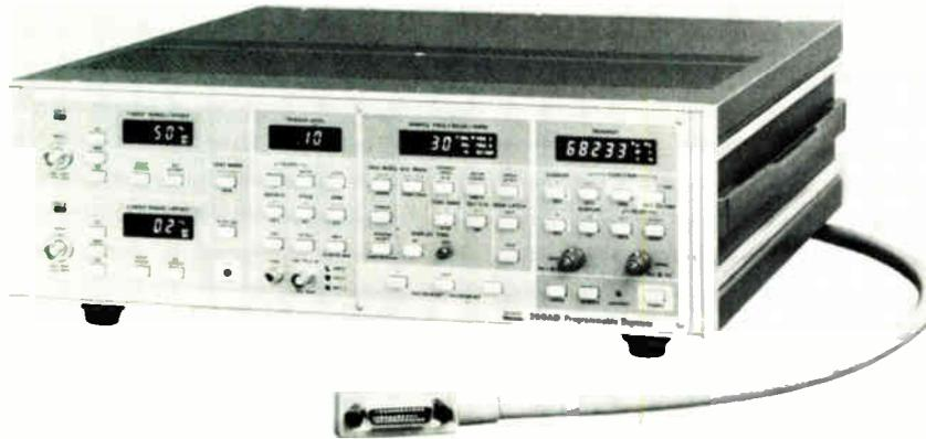
**Options.** The Sony/Tektronix 390AD programmable digitizer can display its output on its own digital readouts or drive external monitors or recorders.
