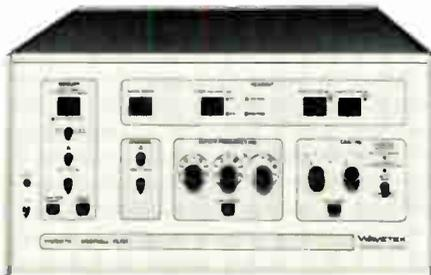
frequencies from 1 Hz to 100 kHz, and 2-digit resolution for 400 discrete frequencies per channel. The passband and stopband characteristics are near-ideal, and you can pair up channels to get band-pass, band-reject or double rolloff (230 dB per octave). Phase match is tight between channels, typically  $\pm 0.5^\circ$ . And the 716 offers even more features, such as sophisticated automatic overload detection and a self-test capability.
