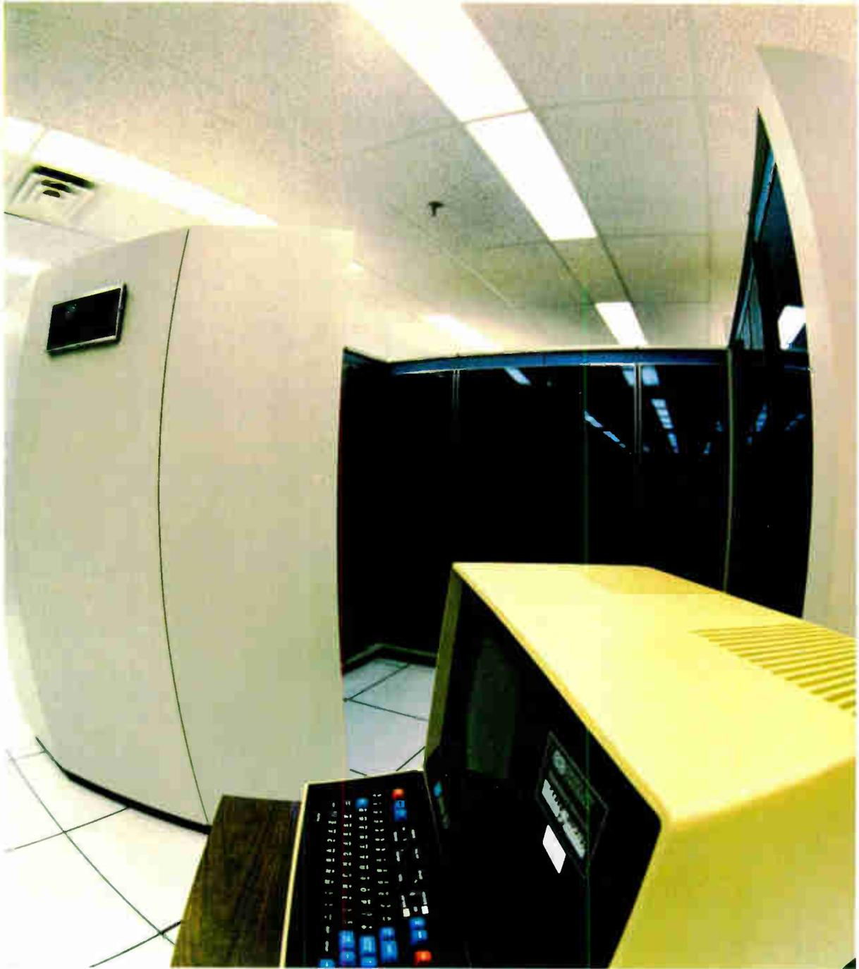
**Supercomputer.** Cyber 205 computer from Control Data is the fastest commercially available. The CPU has two specialized units, one for vector stream (parallel) processing and the other for scalar (serial) processing. The vector processor can operate on 64-bit or 32-bit operands at the exceptionally high rates of 200 and 800 megaflops, respectively.
