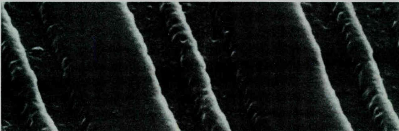
1.0 micron lines over 0.8 micron aluminum steps.
