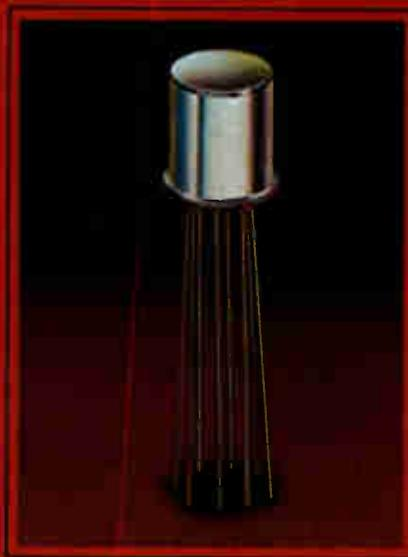
When we first told you about the inherently low inter-contact capacitance and low contact circuit losses of our TO-5 relays, you agreed that they were ideal for RF switching. And you began designing them in immediately. They provided high isolation and low insertion loss up through UHF (typical performance 45 db isolation and 0.1 db insertion loss at 100 MHz).
