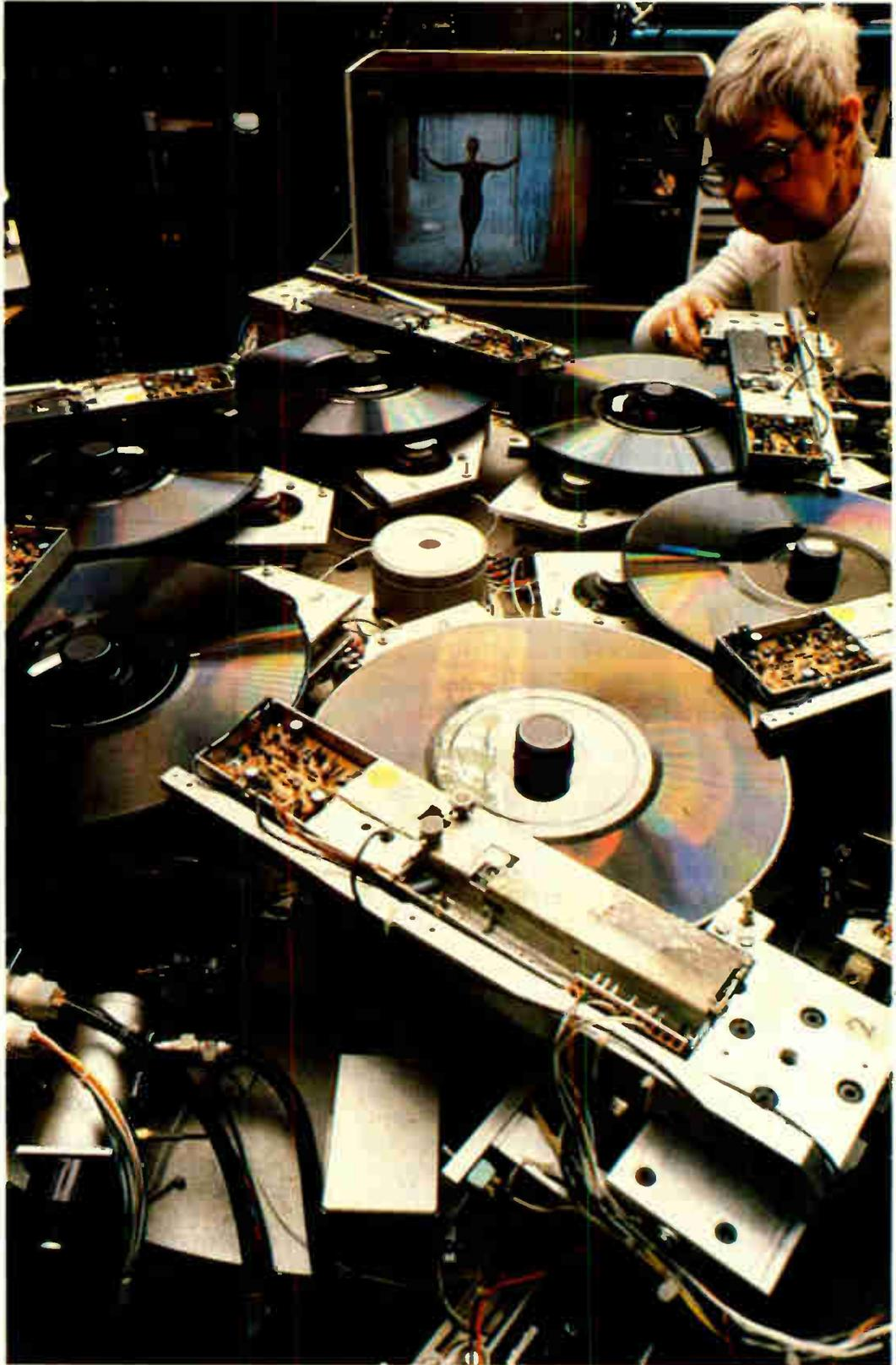
**Video disks.** Fueling the race to develop a consumer video disk system is the lower cost of producing the vinyl disks, compared with magnetic tape cassettes. As shown here at RCA, both the grooved, capacitance electronic disk and the electromechanical pickup stylus are tested to maximize longevity and wear resistance.
