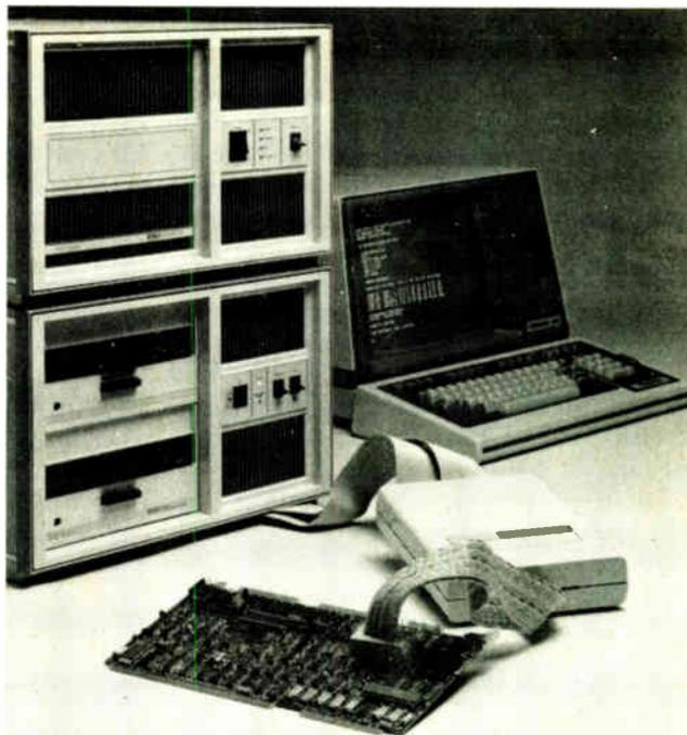
**Development lab.** Design and debugging of hardware and software plus real-time emulation is supported by this Tektronix development system, 8550. It supports 23 different 8-bit processors and several 16-bit processors; multiuser capability will be added soon.
