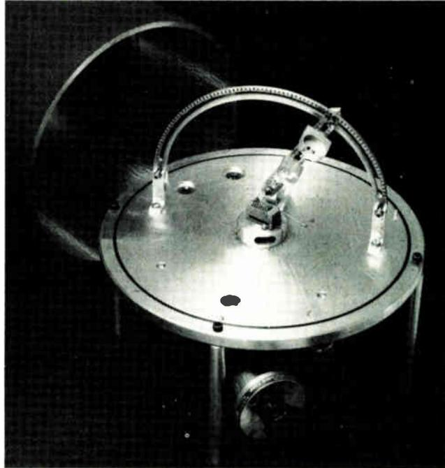
**No air.** When the alpha-error test fixture's vacuum cap (rear) is in place, glass-to-metal feed-throughs allow wires from the chip's socket to be brought out to an integrated-circuit tester that analyzes the data.
