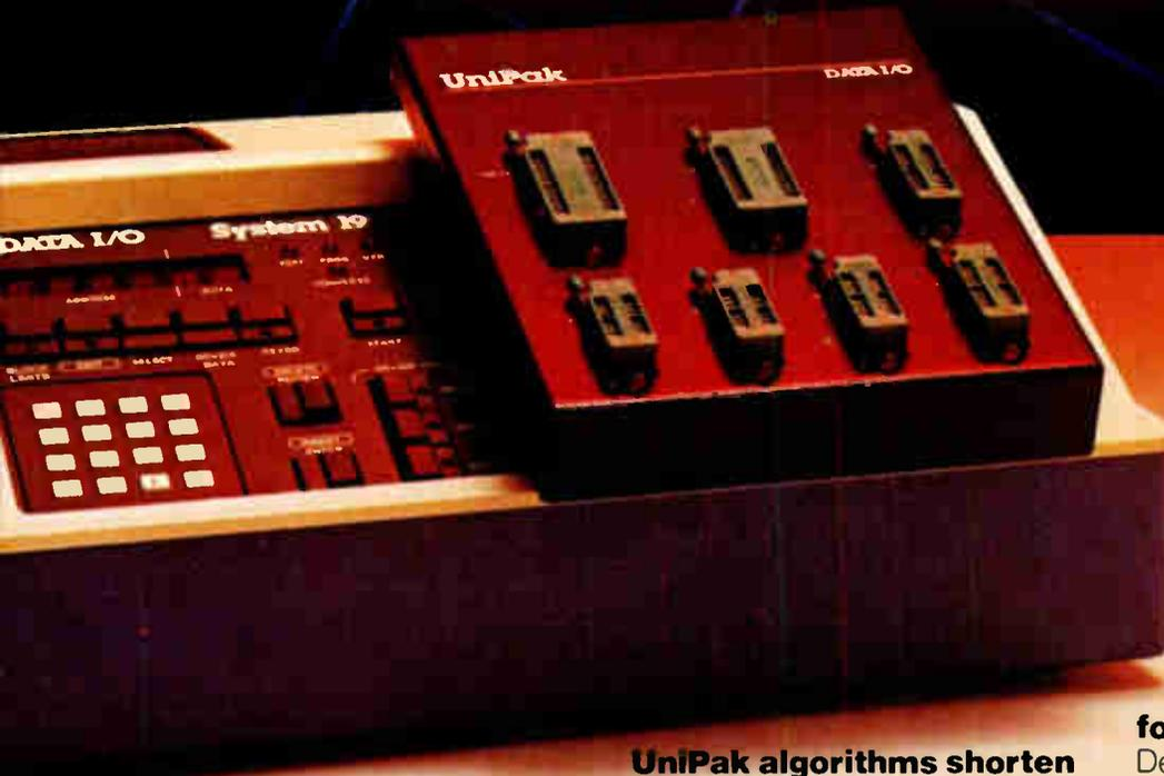
**Our new System 19/UniPak lets you program most MOS and bipolar PROM'S from AMD, Fairchild, Harris, Intel, MMI, Motorola, National, Raytheon, Signetics and Texas Instruments.** UniPak's software assembles the programming algorithm and selects the correct socket for 16, 18, 20, 24 and 28-pin PROMS.
