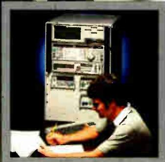
*Output level adjustable in 0.1 dB steps from +19 dBm (13 dBm above 520 MHz) to -140 dBm — displayed in dBm or volts and in relative or absolute units.*
