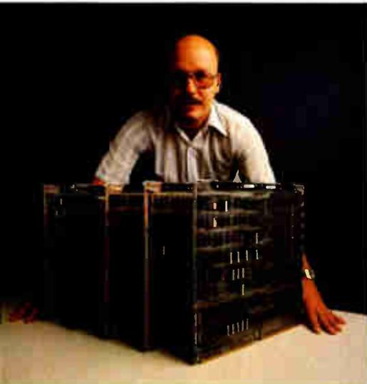
**New this year.** Striving to keep things simple led Hewlett-Packard to design its 100-MHz, 1980A oscilloscope (top) with a single knob whose function is set by depressing a function key. Data General, in its first 32-bit computer, the Eclipse MV/8000 (above), fits the entire central processing unit on just five circuit boards. C-MOS is entering microcomputers like RCA's 1804 8-bit device (right) on sapphire.
