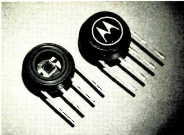
**Practical.** The X-ducer pressure-sensing silicon chip from Motorola Inc.'s Semiconductor Group has made inexpensive pressure-sensing components practical. A single X-shaped silicon element is used for sensing and is housed in a plastic package.
