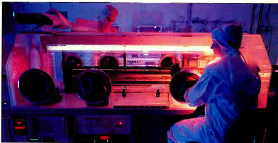
MADE IN N. J. Lytel designed a liquid-phase epitaxy system to make GaAs LEDs and FETs.
