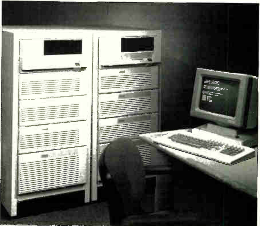
1. ONLINE. Tolerant's Eternity system does fault-tolerant transaction processing at low cost. It executes four transactions a second per building block.
