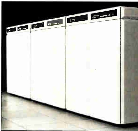
20/20 Teradata's 20-processor DBC/1012 model 2 data-base computer runs at 20 mips and stores 12.4 gigabytes.
