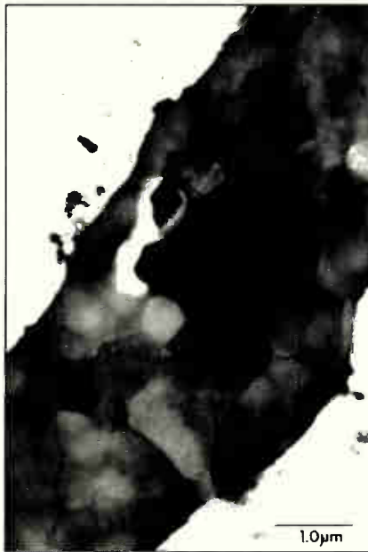
REVEALING. Transmission electron microphotographs of an aluminum metalization line show the large discrepancy in grain size.
