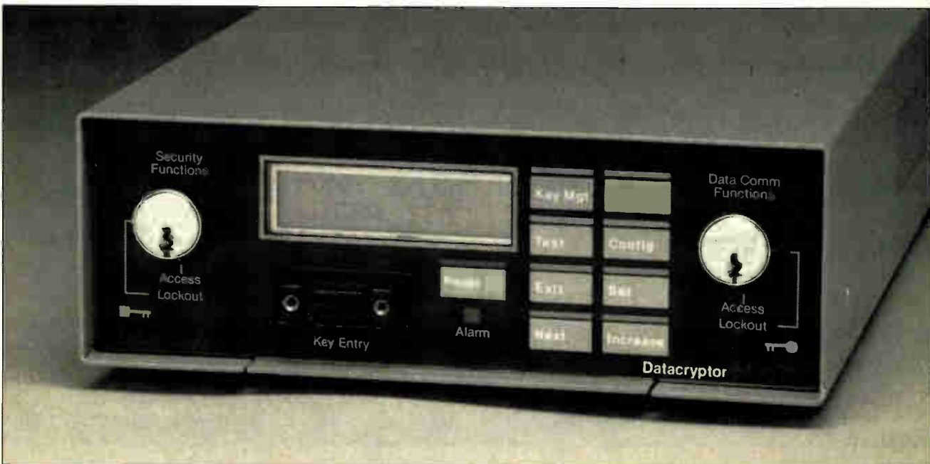
4. CRYPTO BOX. Racal-Milgo's Datacryptor 64-1027 won NSA approval for physical security. The encryption unit includes a tamper-proof housing with dual locks, the automatic rezeroing of the cipher keys during an attempted break-in, and an external alarm.
