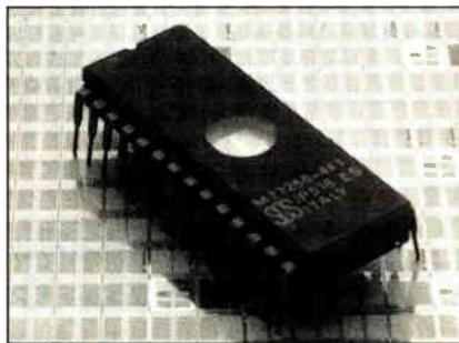
with microprocessors that have 1-mega-byte addressing capabilities, such as Zilog Corp.'s Z family. In standby mode, the TTL-compatible chip reduces power use by 60% without increasing access time. The active current is 100 mA; maximum standby current, 40 mA.
