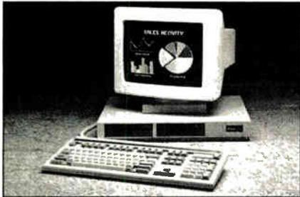
the WYSEpc+ include: 9.54-MHz and 4.77-MHz clocks; a monochrome/color graphics adapter; a 256-K-byte CPU board, expandable to 640-K bytes of RAM; two serial ports and one parallel port; a real-time clock with battery back-up; and a choice of IBM PC AT-style or enhanced-style keyboards.
