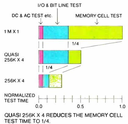
page mode, CAS-before -RAS refresh, and sophisticated test circuitry. NEC have integrated a 4-bit wide test mode that cuts total testing time by up to half. This keeps testing costs down, but maintains a high level of product reliability – essential factors in volume production of large capacity memory chips.
