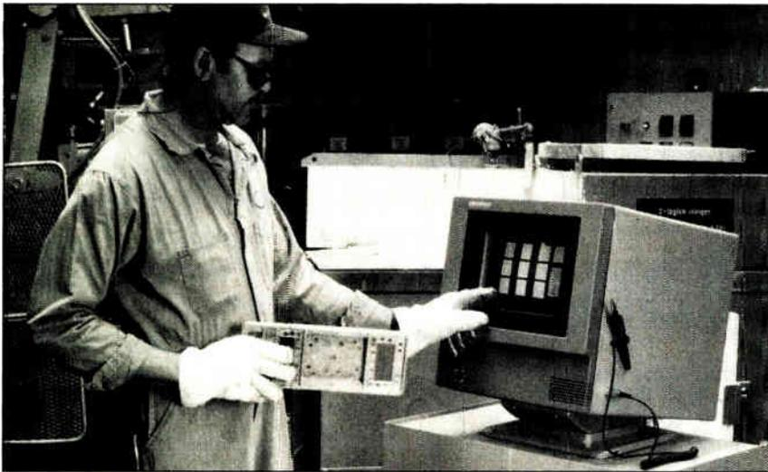
**HARD-HAT INTERFACE.** Rugged, sealed unit has high-resolution graphics and is easy to use.
