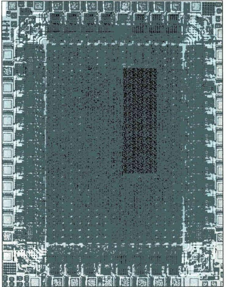
**NO CHANNELS.** This chip was developed using California Devices' channelless gate array router for maximum compaction.
