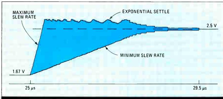
**3. ALL POSSIBILITIES.** The Sierra simulator approximates an amplifier's ramp up in output voltage by considering all the ramp slopes the amp might experience.
