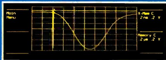
Top: Dual Zoom and time cursors are applied to measure delay between double pulses with 100 ps resolution and 0.002% precision.
