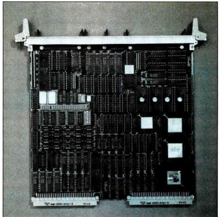
**BUS BOARD.** Heurikon Corp.'s first Multibus II offering, the HK68/M220 board, allows direct memory accesses at 16 megabytes/s in 16.5-MHz systems.
