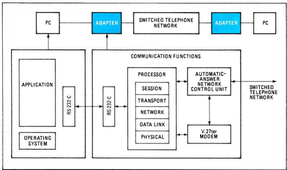
**SIMPLE.** Computer, seeing JUST-PC adapter as a communication function, sends through RS-232-C port.
