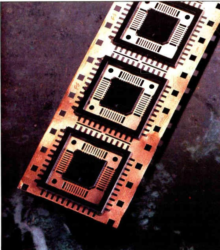
**TAPE PAK.** National Semiconductor's Tape Pak is a small molded package, whose leadframe is a copper tape, with gull-wing leads on 20-mil centers.
