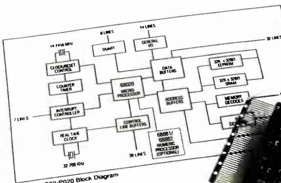
Figure 1. C32-P020 Block Diagram
