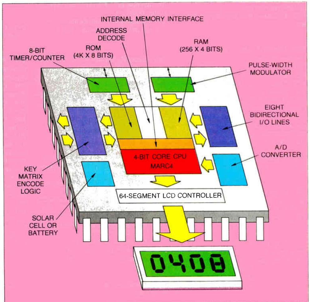
**MARC4 holds a CPU, program and data memory, I/O ports, and such peripherals as LCD drivers; a system can be configured on a single chip.**
