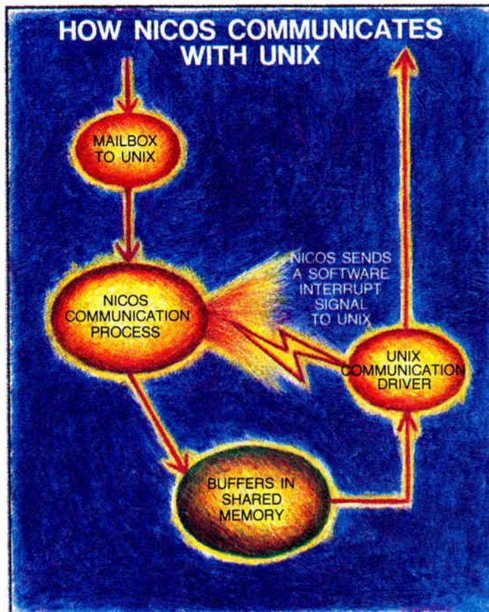
*To send a message to Unix, Nicos copies data into a buffer in shared memory and also sends an interrupt signal.*
