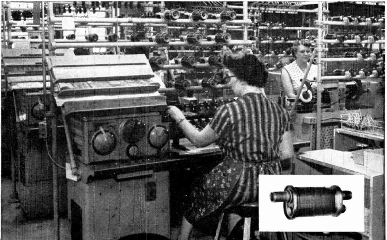
Leeson No. 108 Coil Winders wind coils for the ignition system of the Wright Cyclone Model R-3350 Engine. The system is designed and manufactured by the Scintilla Division of the Bendix Aviation Corporation in Sydney, New York.
