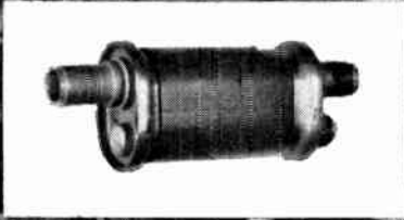
Leeson No. 108 Coil Winders wind coils for the ignition system of the Wright Cyclone Model R-3350 Engine. The system is designed and manufactured by the Scintilla Division of the Bendix Aviation Corporation in Sydney, New York.
