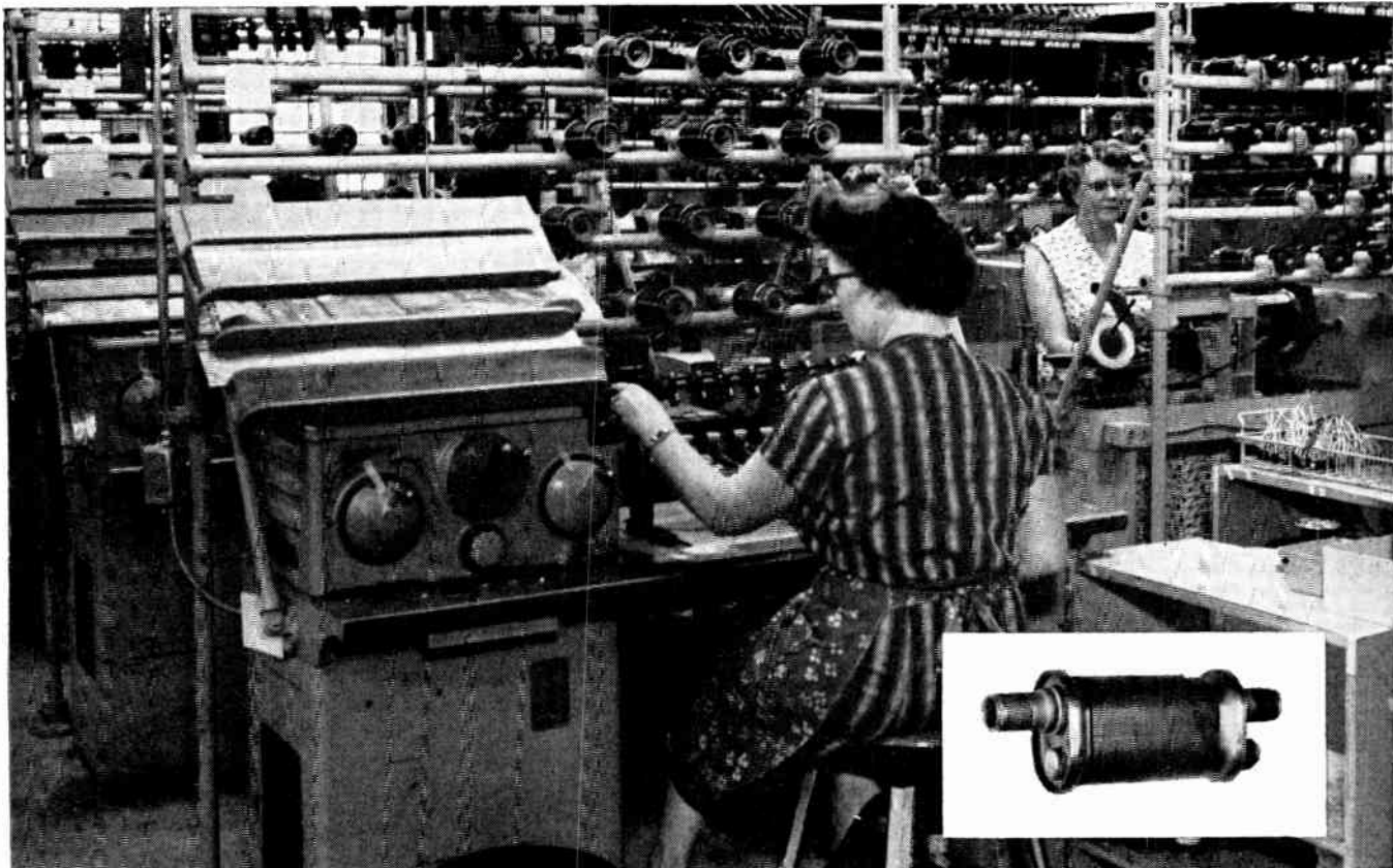
Leesona No. 108 Coil Winders wind coils for the ignition system of the Wright Cyclone Model R-3350 Engine. The system is designed and manufactured by the Scintilla Division of the Bendix Aviation Corporation in Sydney, New York.
