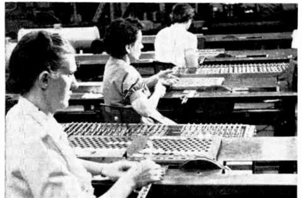
Conveyor for transistor assemblies (Motorola)
