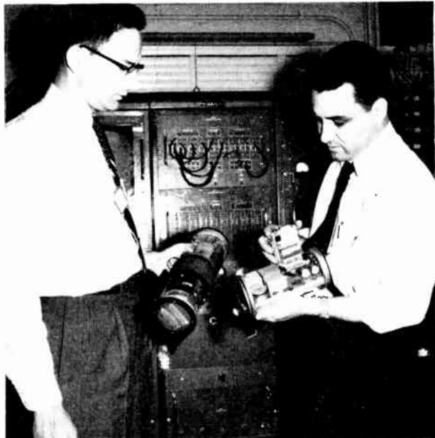
Multicoder by ASCOP responds to 7.5-mv inputs
