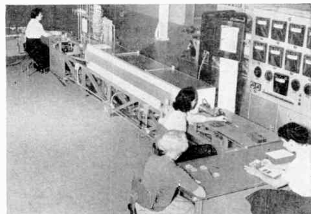
Continuous alloying furnace (RCA)
