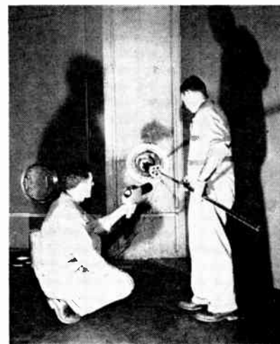
Removing irradiated semiconductor specimens from one of the six-inch beam tubes of the 1,000,000-watt Battelle reactor
