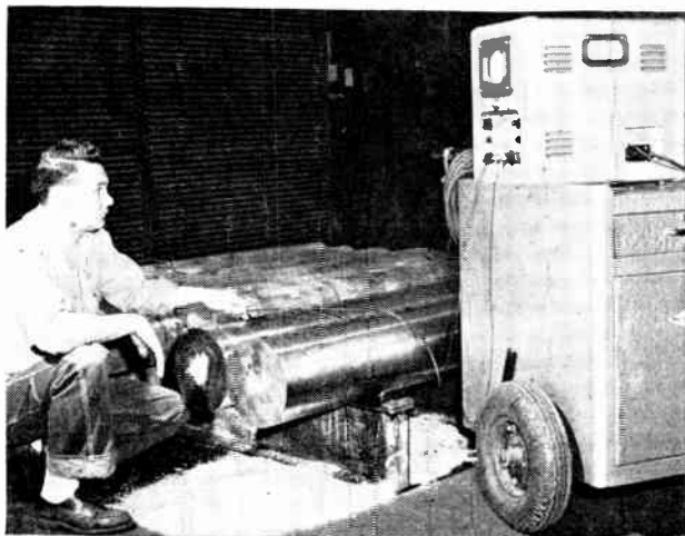
Ultrasonics inspects steel rounds for internal defects
