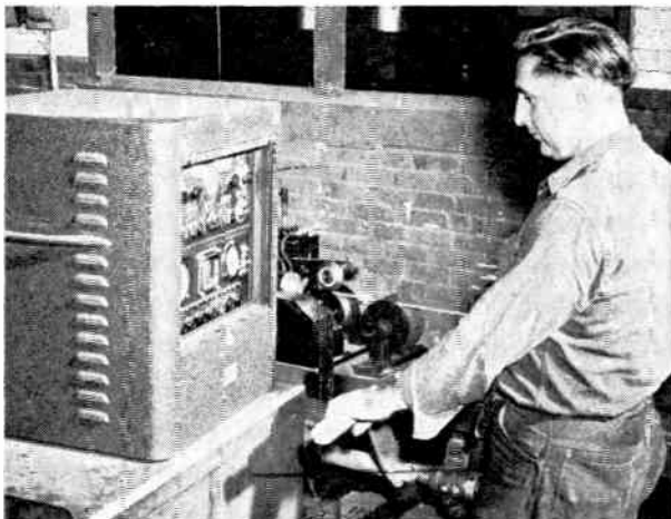
Magnetic analyzer checks bar stock for surface flaws
