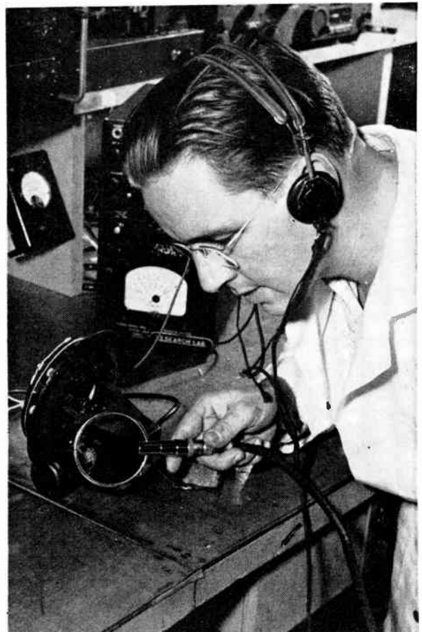
RI from safety-valve motor used in jet fighters is checked by AiResearch technician with stethoscope-like apparatus including probe, amplifier and earphones
