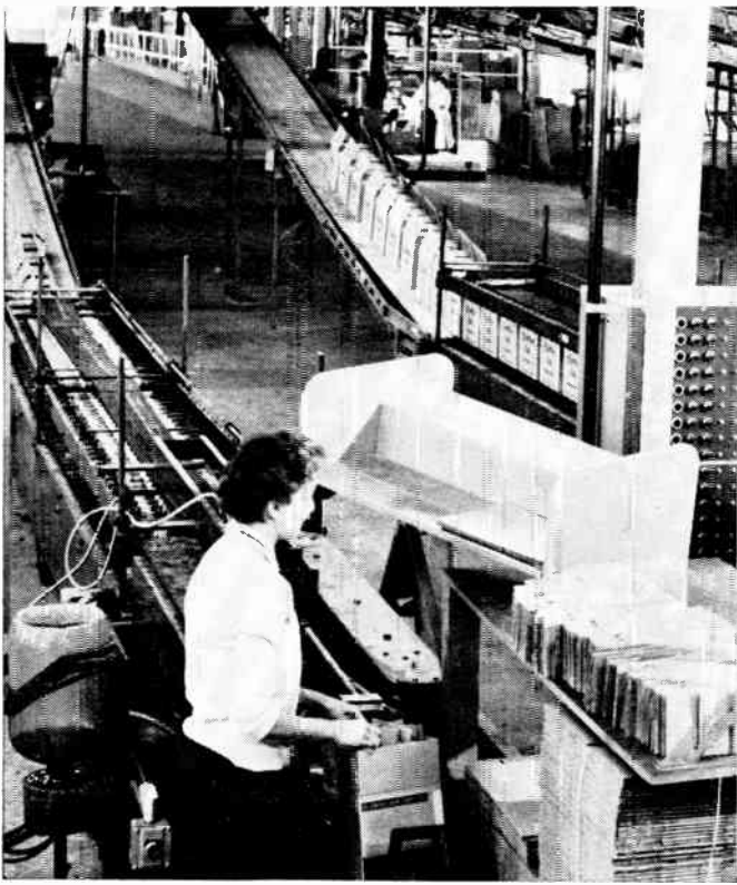
Panels (left) show demand for cartons; photocells (right) rout them along conveyors
