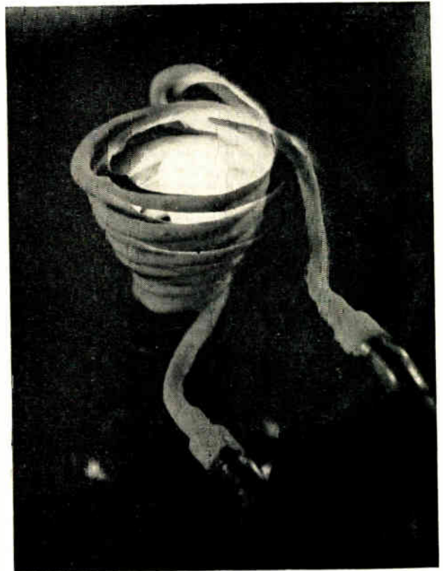
Niobium ball floats and melts in h-f field
