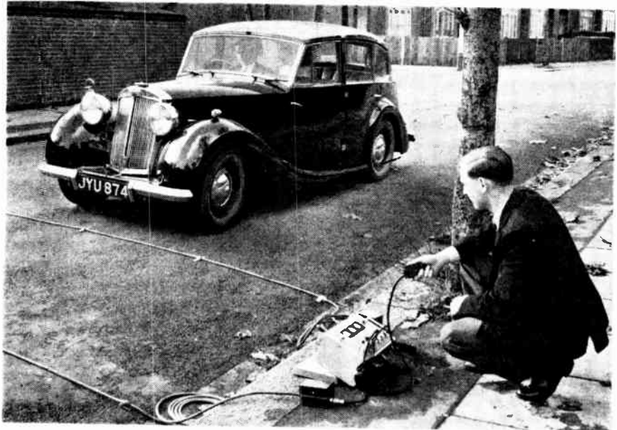
Elapsed time system uses fifty-four transistors to measure automobile speed
