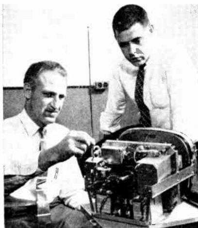
Completely portable all-transistor tv set uses rechargeable nickel-cadmium batteries
