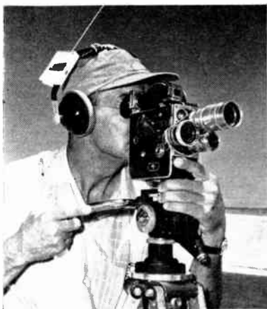
Two pencil flashlight cells power transistorized receiver mounted on ear-protector headset. Cameramen and other employees of Chance Vought Aircraft are kept advised of missile count down and aircraft test flights with small size receiver
