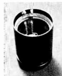
45X magnification and measuring reticle let inspector check winding tap-off gap to .5° (.001"). Potentiometer shown below, actual size . . . tap-off leads at top.
