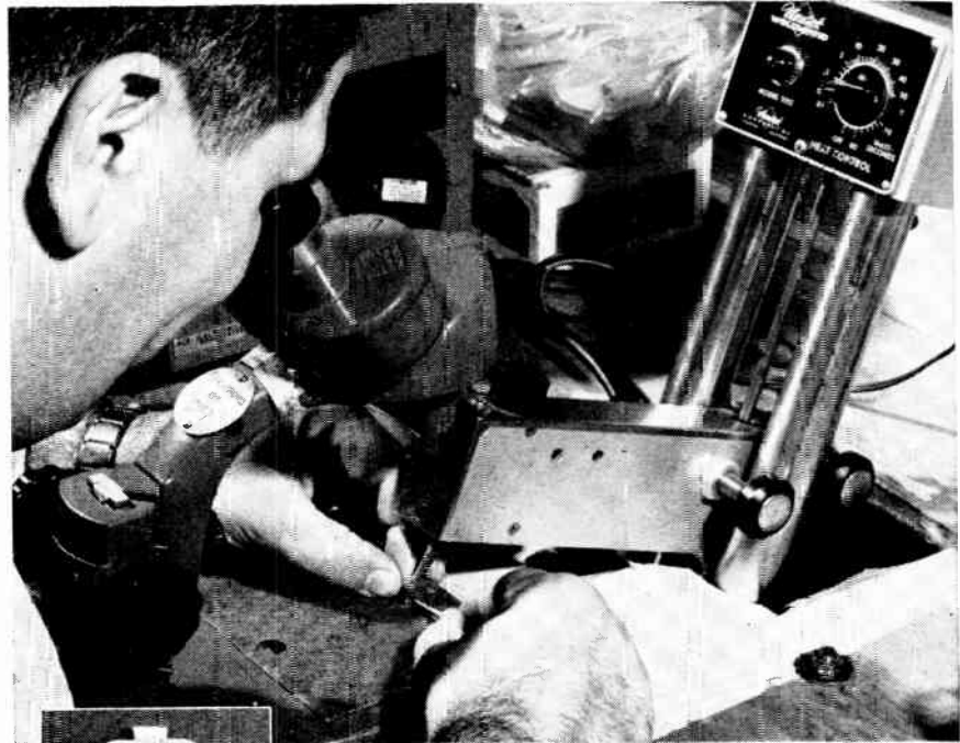
Welding .008" diameter wire to a part the size of a fly's wing—3-D micro-vision makes precision possible.
