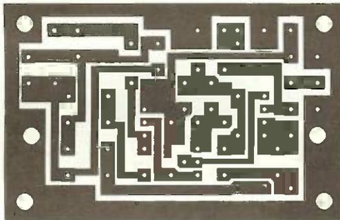
5 LE CIRCUIT IMPRIMÉ DU MILLIVOLTMÈTRE.
