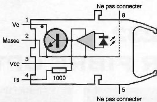
3 LE SCHÉMA DU RÉCEPTEUR OPTIQUE.
