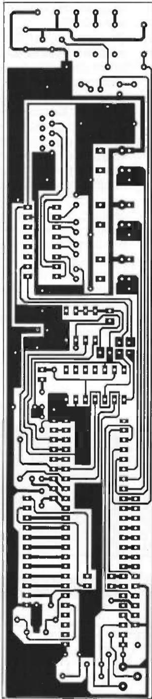
**5a/b** TRACÉ DU CIRCUIT IMPRIMÉ ET IMPLANTATION DES ÉLÉMENTS DE LA PLATINE PROCESSEUR.
