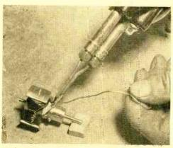
With the armature wound, cleaned and twisted leads from start of one pole to finish of next are soldered to commutator segment.
