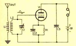
Fig. 5. Detection of audio signal from RF carrier in this triode is termed plate detection.
