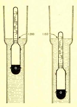
Fig. 4. Hydrometer float in barrel displaces more electrolyte when battery is dead (1.150).
