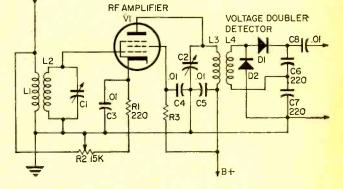
Fig. 16. In this receiver, the desired station frequency is tuned with the variable bandpass filter; the RF amplifier receiver stages are untuned.
