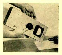
improve on the xenon flashtube reflector and add a collimator/lens assembly to efficiently beam the light to confined areas. Whatever changes you make, avoid repackaging the unit until you have bread-boarded the circuit. The trigger transformer, T2, should always be close to the flashtube so that the trigger wire is as short as possible.
