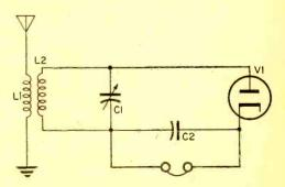
Fig. 7. In this AM detector circuit, capacitor C2 functions as an RF bypass for the headset.
