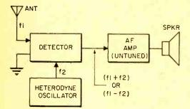
Fig. 1. In the heterodyne receiver, detected signal is passed directly to audio amplifier.
