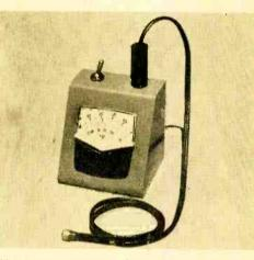
Meter cases are home-brew favorites; this one holds meter scaled for temperature readings. The sensor, plugged into the circuit housed in the meter case, is immersed in photographic fixing baths to monitor their temperature.
