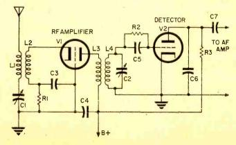
Fig. 19. The grounded grid amplifier shown here is tuned by series combination of L1 and C1. The detector is tuned by parallel resonant circuit L4-C2.
