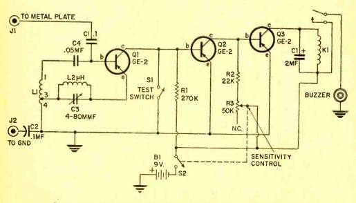
Capacitance between an intruder and the metal plate or strap is coupled to oscillator transistor Q1 through jack J1 to trigger the circuit.
