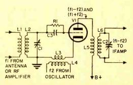
Fig. 3. In this circuit, triode V1 is the converter where frequencies f1 and f2 are mixed.
