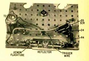
The stroboscope is wired into a flat, long, aluminum chassis box permitting uncrowding of parts. Perforated circuit board (above) mounts on meter screw posts (see below). Except for resistor R9 (hidden under capacitor C2) all parts are shown in photos.
