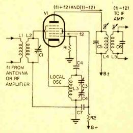
Fig. 5. Pentagrid converter tube V1 combines functions of converter and local oscillator.
