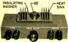
Top mount and heat sink dissipate Q2's heat.
