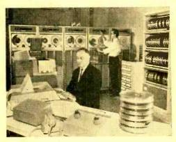
Credit checks on subscription lists transmitted by telephone line facilities from distant centers are automatically processed by computer and transmitted back.
