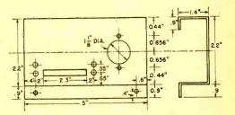
The dimensions for the overall size of the control chassis is not critical except for mounting holes for relay K2 and 6-terminal barrier strip J1 where cables connect.
