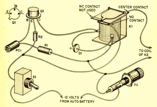
Pictorial diagram of the Auto-Dimmer showing how wires interconnect the various parts. Exact parts placement and lead lengths are not critical. However, it is suggested that the builder follow construction details in this article carefully.
