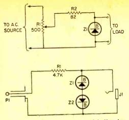
Fig. 12. Limiting one or both of half-cycles.
