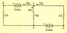
Fig. 3. When solving Kirchhoff's voltage law for closed loop circuits, remember that if the resulting current value is negative, current's flowing opposite from direction you assumed.
