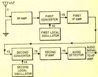
Fig. 7. The dual-conversion superheterodyne receiver has two frequency converters. Two IF frequencies, f3 and f5, are produced, f5 being an even lower frequency than f3 to minimize possibility of image problems.
