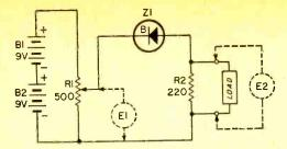
Fig. 9. Schematic diagram shows use of Zener diode in the series voltage regulator circuit.
