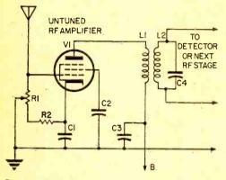
Fig. 18. The RF amplifier of this circuit is untuned—the signal from the antenna is fed directly to the control grid of the pentode. But the detector stage is tuned, however.
