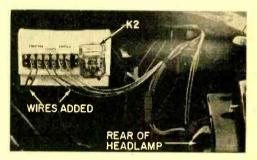
View of the control chassis installed under the hood of the author's car. Mount where the unit will be accessible for inspection.
