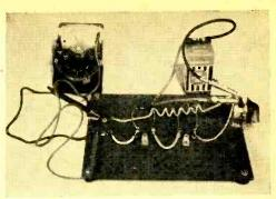
Fig. 6. Ammeter hooked to Fahnestock clips.
