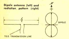
wavelength. Something known as "end effect" electrically shortens the antenna, so it must be shortened physically to be electrically correct. For this reason, a dipole's length is calculated from the modified formula.
