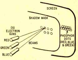
Fig. 8. Conventional color tube uses three guns, shadow mask, and phosphor-dot screen.
