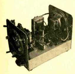
Orderly component layout characterizes this unit built around clock-timer mechanism.
