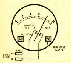
Fig. 1. Basic voltmeter circuit showing the resistor and the moving coil loading effect.
