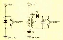
Fig. 1. (left) Selectivity of basic TRF is low. Fig. 2. (right) More selective tunable circuit.
