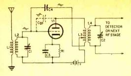
Fig. 10. Cancelling feedback signal through Cgp with output sample prevents oscillation.
