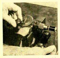
Hand drill used as shown helps speed the winding of 300 turns of wire on the field coil—a spool that measures 5/16x1-3/32 in.
