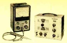
Fig. 8. VTVM and signal generator are all you need to align superheterodyne receivers.
