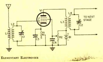
Fig. 12. Addition of a third grid results in pentode which has improved gain over lesser element tubes, and easier control of gain. Choice of control gives remote or sharp cutoff.
