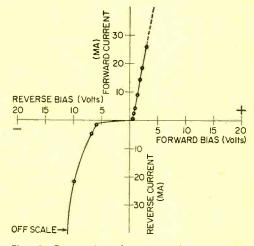
Fig. 8. Forward and reverse characteristics.
