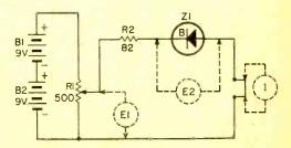
Fig. 7. Diagram for the reverse characteristics.
