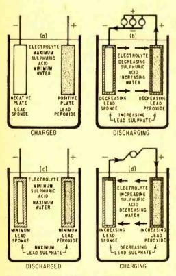
Fig. 1. These graphic illustrations trace the cycle of chemical reactions in storage batteries. Sulphuric acid, H<sub>2</sub>SO<sub>4</sub>, breaks down to water H<sub>2</sub>O, during discharge; lead forms PbSO<sub>4</sub>.
