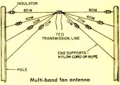
as you can make it. If you suspect a high harmonic output, utilize an antenna tuner between the transmitter and the antenna system; the tuner will stop harmonic energy before it is radiated.
