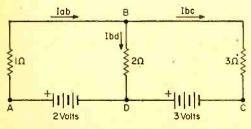
Fig. 2. Kirchhoff's voltage law analyzes closed path circuits; two here are DABD and DBCD.
