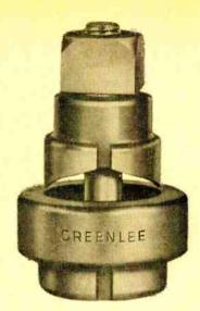
Chassis punches are available in many shapes; above is "key" punch for keyed radio sockets.
