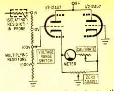
Fig. 4. Basic VTVM circuit showing the zero adjust and calibrate potentiometers.
