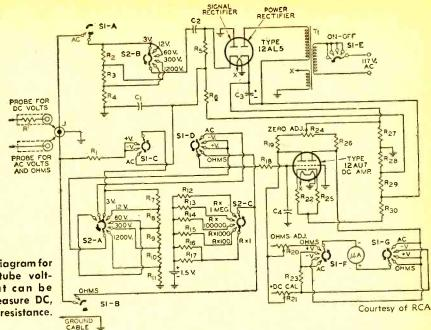
Schematic diagram for a vacuum-tube voltmeter that can be used to measure DC, AC, and resistance.
