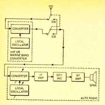
Fig. 8. Dual-conversion in a superheterodyne has many applications. Here a short-wave or marine band converter is used with an automobile broadcast band radio to give listener choice of either band.
