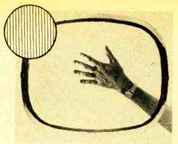
Fig. 1. Conventional color tubes use a dot-pattern shadow mask (left) that consists of many fine holes; Chromatron uses fine, evenly spaced grid wires (right). Note difference in transparency of the masks which increases brightness.
