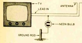
Lightning can ruin a TV set, even one with a lightning arrestor. For added protection connect a glow lamp (NE-7) between the set's antenna terminals and ground rod as shown. Voltages over 55 volts will then pass through the bulb to ground, thus bypassing the set.
