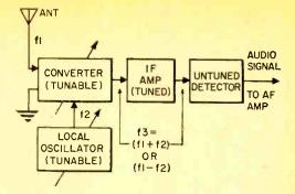
Fig. 2. The superheterodyne receiver is characterized by its one or more IF amplifiers.
