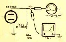
Fig. 5. Voltmeter presents a greater load to the tube's plate circuit than the VTVM.
