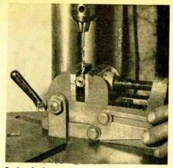
Each of three pole end pieces is drilled with a countersunk hole and tapped to take 10-32 flathead machine screws filed flush.
