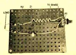
Fig. 10. Series voltage regulator breadboard.
