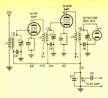
Fig. 14. Tuned radio frequency stage employing an automatic volume control circuit. The circuit maintains constant signal strength to AF amplifier despite strength of incoming RF.
