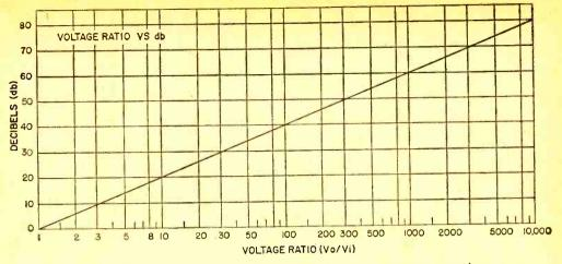
Fig. 4. The above graph can be used to find db when voltage ratios are known.
