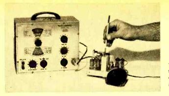
With the signal generator set to internal modulation, good alignment is achieved by peaking the IF amplifiers for maximum signal output heard.
