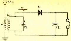
Fig. 3. Parallel resonant tuning of this receiver is effected by adjusting capacitor C1.
