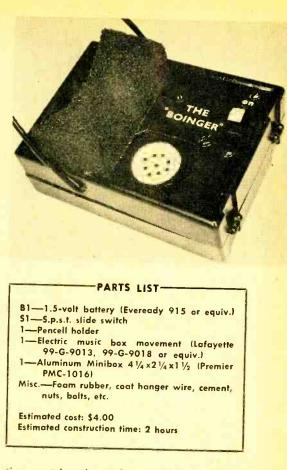
tine must be triggered from below, or it will break off in a short time. If the drum is turning in the wrong direction, that is, triggering the tine from above, then turn the battery over in its holder. When the proper direction has been found, put a dab of red nail polish on the positive battery holder terminal so that you will know which end of the battery goes where when you replace the battery at some future date.
