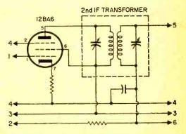
Fig. 5. IF amplifier tube 12BA6 boosts signal; second IF transformer increases selectivity.
