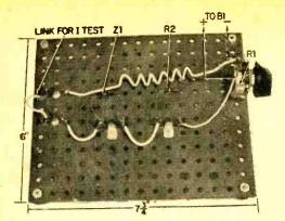
Fig. 5. Components are mounted on Masonite.
