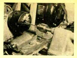
Lathe setup is used to drill .128-in. hole through center of hexagonal center core of mild steel which serves as motor armature. A drill press can do this job if a lathe is not available—be sure to hit center,
