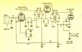
Fig. 6. "Front end" of a standard AM broadcast receiver is shown here in schematic diagram. The circuit combines the individual elements that have been discussed: the converter and local oscillator, the IF amplifier, and the detector. But note the addition of the feedback circuit, marked AVC, which maintains automatic volume control of receiver.
