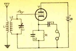
Fig. 6. The audio signal in the infinite impedance detector is developed across resistor R1.
