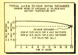
Fig. 6. Association of Automobile Battery Manufacturers established the 20-hour yardstick.
