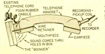
The Boinger attaches directly to the mouthpiece of your telephone, and puts out an audible "boing" every 15 seconds. It is used when recording a telephone conversation to remind both parties that the conversation is being recorded. This is a Federal law on interstate calls and is also a law on local telephone calls in a large number of our 50 states.
