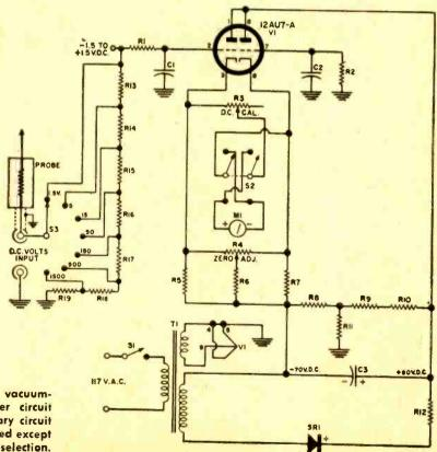
Here is a simple vacuumtube DC voltmeter circuit with all unnecessary circuit switching eliminated except on/off and range selection.
