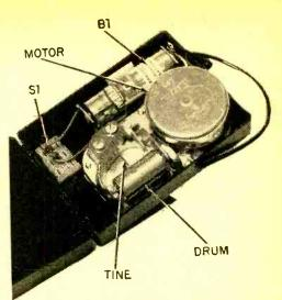
Small size of the music box movement makes Boinger feasible for use on telephone handset. Note the removal of all tines but one.
