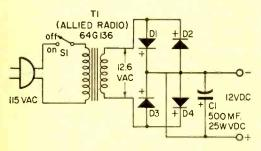
Fig. 4. This power supply is easy to build.
