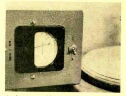
A phono turntable and strobe disc (above) calibrate the stroboscope. Below, strobe measures unloaded speed of a power tool.
