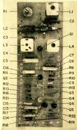
Top view of circuit board that holds almost all the components for an SCA-FM adapter project; rat's nest wiring is eliminated.
