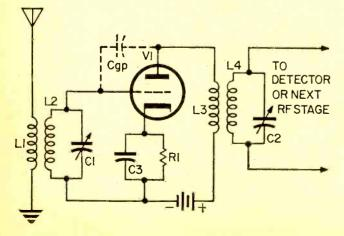
Fig. 9. Feedback from plate to grid through the effective capacitance, Cgp, in this RF amplifier stage occurs easily and results in oscillation. The oscillation-producing positive feedback is actually desired in a tuned plate-tuned grid circuit.
