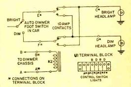
Schematic diagram for the control chassis mounted under the automobile's hood. The hot leads to the bright and dim headlamps are cut. Then, ends that trace back to the dimmer switch connect to terminals E\* and F\*. The ends that trace back to the headlamps connect to terminals C\* and D\*. ply by pushing the footswitch. The reverse is also true—if the lights dim when they should remain bright, the footswitch will override the automatic dimmer and restore the lamps to high beam.
