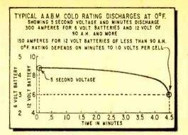
Fig. 7. Another important criterion for rating a battery is its auto engine cranking ability.
