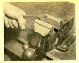
Field side pieces are made of soft, flat steel stock. Their curved partians are bent around the pipe coupling held in a vise as shown.
