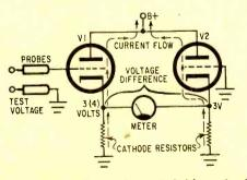
Fig. 3. Simplified balanced bridge circuit that is usually used in modern VTVM devices.
