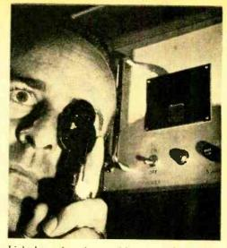
Light heam from laser welder is aimed by holding the compact ophthalmoscope-like instrument to doctor's eye.
