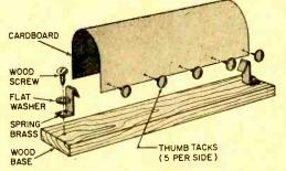
Assemble the battery holder by first determining the distance required between the spring brass end terminals. Do this by laying out the number of dry cells the holder will mount and scribe lines at ends.
