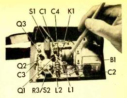
Transistor oscillator coil L1 is the fixed coil in the oscillator circuit. L2 is adjustable to provide increased sensitivity. The trimmer screw of oscillator circuit capacitor C3 is conveniently located on the front panel to provide easy adjustment to bring on oscillation.
