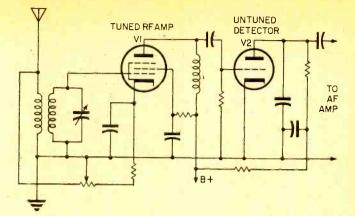
Fig. 17. Another circuit illustrating operation without all stages tuned. Here only the RF amplifier need be tuned to select and detect the desired frequency.
