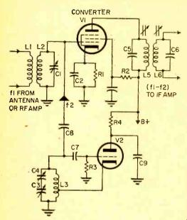
Fig. 4. This converter stage utilizes pentode tube V1 and the local oscillator triode V2.
