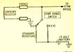
Fig. 7. Simplified input circuit to VTVM bridge circuit for measuring resistance values.
