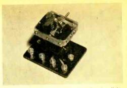
Close-up view of motor reveals simplicity of construction. Of an extremely compact design, the motor stands only  $2\frac{3}{8}$  in. high.
