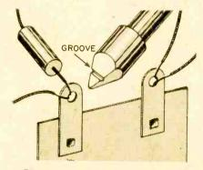
File a groove in one side of your soldering iron for "pouring" solder on connections of a crowded chassis.
