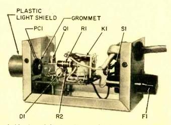
Inside view of the Auto-Dimmer showing location of parts. Relay K1 is isolated from metal case by phenolic board.
