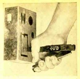
"Nibbling" tool cuts any shape hole in steel or aluminum chassis; costs about four dollars.
