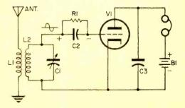
Fig. 4. Triode tube replaced the crystal diode combining detection and audio amplification.
