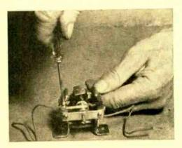
An insulated wire is connected under each brush screw; the other ends are connected to the terminals marked A on base of the motor.
