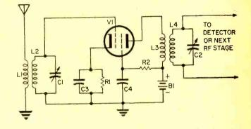
cathode resistors which are bypassed by capacitors for RF. Their tuned circuits are equipped with RF bypass capacitors (C2 and C4) which are large enough to not affect the tuning by C1 and C3 and, at the same time, to increase the AVC time constant so as to prevent too fast a change in AVC voltage.
