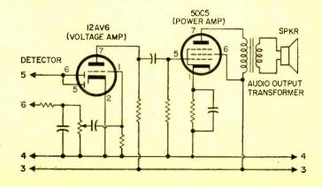
Fig. 6. The audio amplifier section of the receiver combines detection and voltage amplification in the 12AC6 tube, and power amplification in 50C5.
