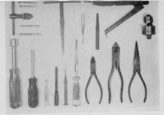
METAL-WORKING TOOLS for electronics include an assortiment of taps and a tap-handle, a reamer, tweezer, center punch, hand nibbler, chassis punches, nut-drivers, screwdrivers, wire cutters and pliers. Have tools on hand.
