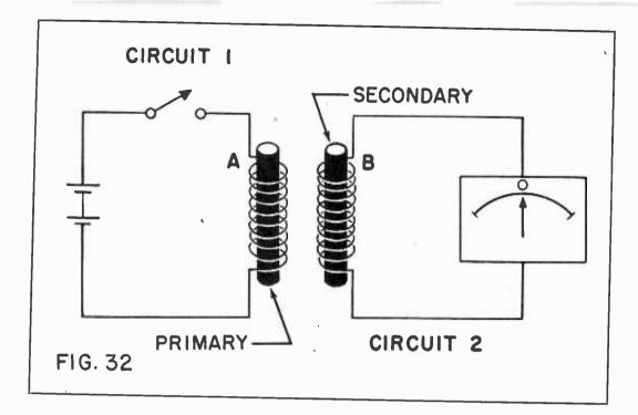
mary of the transformer produces variation in the magnetic flux circulation in the transformer core which tends to oppose the current flowing in the primary winding by virtue of self-induction. This counter EMF is just about equal to the voltage applied to the primary winding when no load is connected to the transformer's secondary winding. This accounts for the fact that very little current flows through the primary winding when no load is connected to the secondary. The negli-
