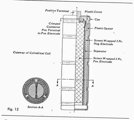
The mercury cell offers the highest efficiency of any primary cell, converting between 80% and 90% of its active chemicals into electrical energy.
