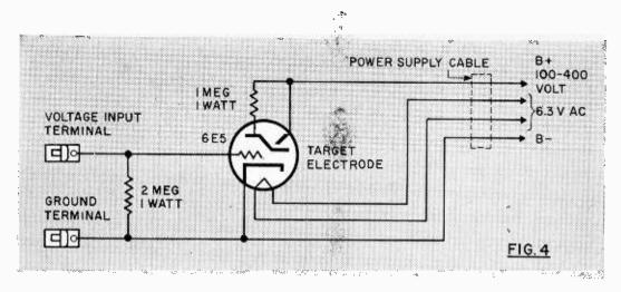
ring to the diagram will show the connections, and it may be used with any amateur transmitter that employs coaxial cable output. The power consumed by this indicator is in the microwatts, and negligible by any ordinary standards, so it does not waste valuable RF watts. It also indicates relative degree of modulation.
