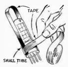
cured around the bottom with another strip of tape. Don't use tape on tubes that heat up excessively, because of the possible danger of fire due to tape igniting. *Never* use plastic tape for this purpose as it ignites easily.
