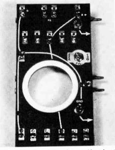
Fig. 10: Basic unit seen from the top with no insert. Lines indicate commonly-connected clips. Note plug and jack positions.
