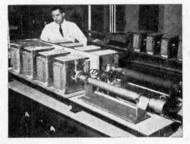
ZONE REFINING furnace is what this device is called. It's used for purifying Germanium in producing transistors. Selected blanks are heat-treated.
