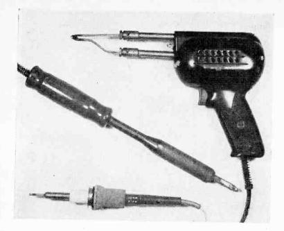
SOLDERING TOOLS are very important. The three most commonly used varieties are in the photo at left. The soldering gun, the standard iron and pencil iron.
