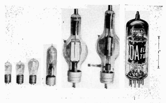
HOW'S THIS FOR PROGRESS? Early vacuum tubes were big and bulky. Filaments were so bright you could read by their light, and they weren't very efficient either. They were assembled one at a time, cost was outrageous.
