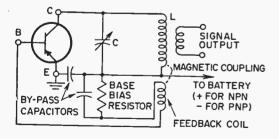
ONE TYPE OF TRANSISTOR OSCILLATOR
