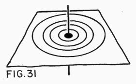
dependent upon the number of turns in the coil; a coil with many turns will have greater inductance than a coil with few turns. Also, if an iron core is inserted into the coil, the inductance of the coil will increase sharply. The unit of inductance is known as the Henry.
