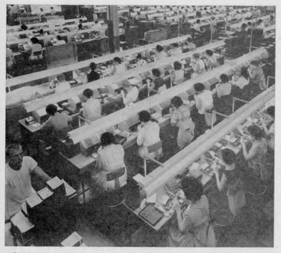
MINIATURE TUBE PRODUCTION is carried on in almost sterile conditions. Tubes are assembled from the insideout, using small tack-welders. After assemble of parts, all metal parts are heat-cleaned, then assembled in glass. dollar industry, largely based upon this "impractical" device.
