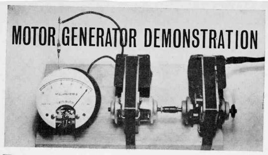
WO old phono motors, salvaged from junked 78-rpm record players, can be used to demonstrate the fundamentals of a motor-generator set. Two motors are strapped to a piece of board, and the shafts are coupled with tape so that one motor drives the other. The captive motor generates a small ac current which is rectified to dc by a germanium diode and then registered on a dc milliammeter.
