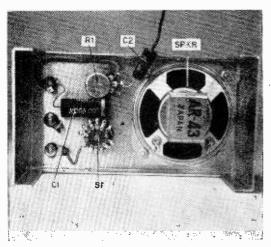
FIG. 4: Chassis-mounted parts inside the box cover include the speaker, switch, potentiometer, jacks and two capacitors. Wire these in place separately.
