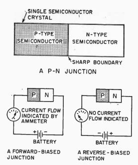
RULE FOR JUNCTION BIASING: WHEN THE POSITIVE TERMINAL OF THE SOURCE IS CONNECTED TO THE P-MATERIAL AND THE NEGATIVE TO THE N-MATERIAL, THE JUNCTION IS FORWARD BIASED.
