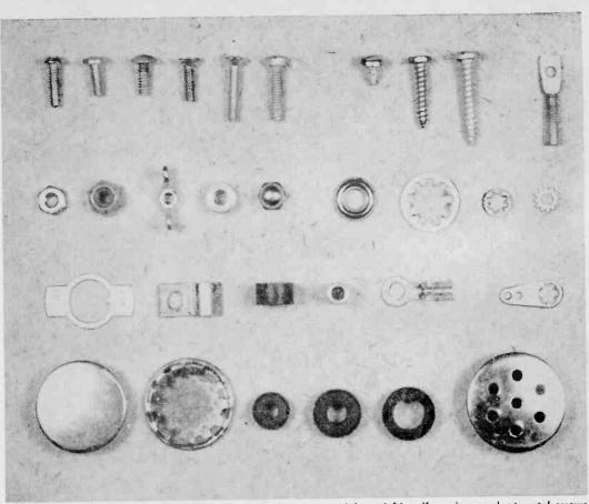
MORE HARDWARE YOU'LL SEE includes assorted machine screws (above left), self-tapping or sheet metal screws, spade bolts, various nuts, lockwashers, switch plates, cable clamps, solder lugs, grommets and snap-hole plugs.
