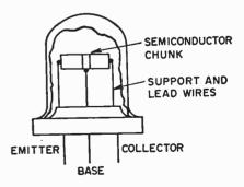
CUTAWAY VIEW OF ONE TYPE OF TRANSISTOR Actually a transistor is a semiconductor sandwich. The NPN transistor consists of two regions of N-type semiconductor, as the bread of the sandwich, and a very thin region of P-type semiconductor as the meat. In the PNP transistor the bread is P-type semiconductor and the meat is N-type. The central
