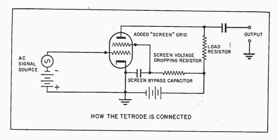
From what has been said, it might be inferred that the triode is the only kind of amplifying vacuum tube. This is by no means the case. In fact it might not even be the mostcommonly used type today. In the late twenties it was discovered that the addition of a second grid, between the already-present grid number one and the plate, would give the tube superior amplifying properties. Thus the tetrode or four-element tube was born.
