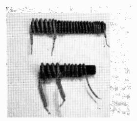
Fig. 4: The coils, wound on ferrite with insulated wire.
