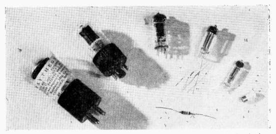
FAMILY PORTRAIT. Here is a sum total of 25 years of tube development. At the far left is a BH Rectifier tube, then an octal-base tube followed by a miniature, two sub-miniatures and a germanium diode. At far right is transistor.
