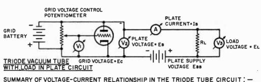
WHEN THE READING OF VI INCREASES (GRID BECOMES MORE NEGATIVE) THEN READING OF <u>A</u> WILL DECREASE, V2 WILL INCREASE, AND V3 WILL DECREASE. THE READING OF V3 AND <u>A</u> WILL INCREASE AND DECREASE TOGETHER SINCE V3 = IBX RL, THE READING OF V2 AND V3 WILL CHANGE OPPOSITELY SINCE EB + EL = EBB, AND EBB IS CONSTANT
