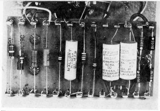
TERMINAL BOARD MOUNTING was pioneered for the military. It's easy to make a chassis look neat this way! Wires lead to and from the board, component parts mount on the board, are easy to service or replace.
