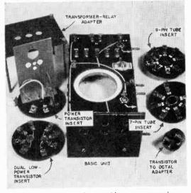
Fig. 9: The basic unit shown with some accessories. These fit the large center hole and permit breadboarding circuits.
