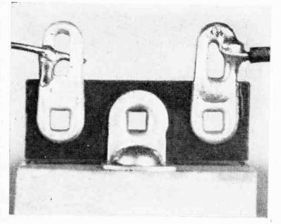
GOOD AND BAD soldering techniques illustrated. Wire at left is simply poked through and tacked. Wire at right is first made mechanically sound, soldered. enough to permit the teeth to press against the nut if regular nuts are used. Both internal and external lock washers are used, and some are large enough for use with controls and switches.
