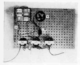
FIG. 4: Follow the parts p.acemen: indicated in the photograph above. Switch is a Mueller Minigator clip.
