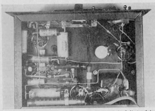
NEATLY WIRED CHASSIS may look like a rat's-nest maze to a neophyte, but notice that all wiring is neatly dressed, and squazed off. No loose components to flop around here! All filament wires twisted help avoid hum.
