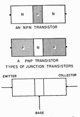
CONNECTING - POINTS, OR "ELEMENTS" OF THE TRANSISTOR (THESE ARE THE SAME FOR BOTH NPN AND PNP UNITS)
