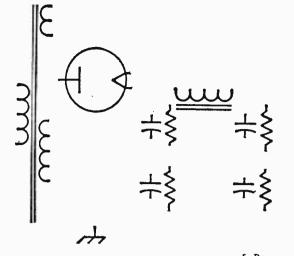
5. Draw a schematic diagram of a pentode audio power-amplifier stage with an output coupling trans-former and load resistor, showing suitable instruments connected in the secondary for measurement of the audio-frequency voltage and current, and naming each component part.
