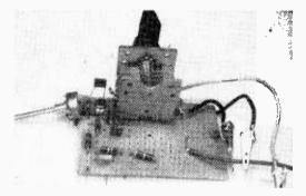
Fig. 2: Tap view of the tuner. Note that the potentiometer is supported to the mounting board only by its connections.
