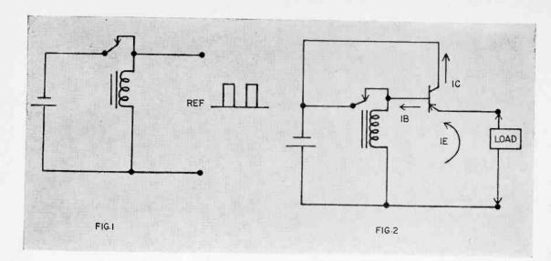
though a voltage of only about 1 volt rms is available from the circuit arrangement of Fig. 2, the desired voltage output is 600 to 1500 volts. The power available at a transformer secondary is never more than the power into the primary. Therefore high current is required in the primary although the secondary current is small.
