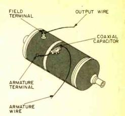
A generator's high whine can often be silenced by installing a coaxial capacitor at the armature terminal of the generator.
