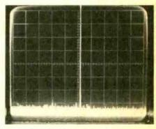
Is it clean? This 'scope trace off our spectrum analyzer shows only the signal, and the analyzer's noise as "grass" some 55 to 60 dB down. Each horizontal division is 5 MHz, so you're looking at 25 MHz either side of the carrier. We couldn't find any trace of a second harmonic in the "grass" so we're not showing a photo because there's nothing to show.
