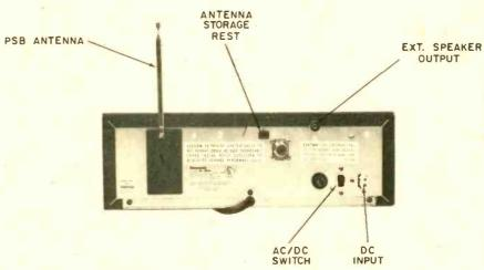
The telescopic PSB antenna can be pivoted so it lies horizontal for storage on a locking rest. For portable or mobile operation a 12 to 15 VDC power supply is connected to the DC input jack and the AC/DC switch is set for DC.
