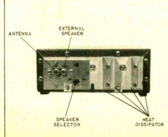
This photo shows the rear apron of the Heathkit HW-2036. As you see, the antenna connector and the external speaker connector are both phono plugs. You must be careful not to confuse the two, even though they are both clearly marked. The photo also shows the ample cooling fins for the RF output transistors.
