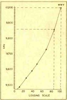
Note how WWV, 10,000 kHz, corresponds to 100 on the logging scale and a station known to operate at 9,850 kHz is found to correspond to 85. The points plotted on the middle and low sections help insure the graph's fidelity throughout it's range.
