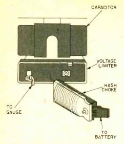
An erratic scraping noise may point to your vehicle's noise limiter. Try installing a hash filter in series with the limiter and battery; also install either a pigtail or a coaxial capacitor at the terminal.
