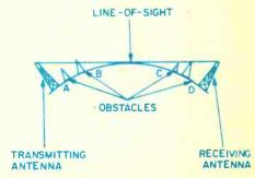
There are four possible ways obstacles may be positioned between a receiving and a transmitting antenna. Note that A and C are below line-of-sight between the antennas.
