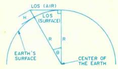
This figure illustrates the geometry on which the charts and diagrams are based. Note that r is measured from the center of the earth and H is the height of the antenna. count for less than a 10% increase in overall range. The antenna heights calculated here will guarantee reception of a clean signal which is caught "on the
