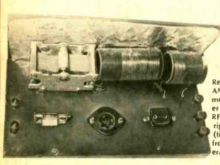
Rear view of the Breadboard AMer shows grid-leak resistor mounted atop capacitor (lower left) next to tube socket, RF bypass capacitor at lower right. Note that right-hand (tickler) coil is rotated from front panel to adjust regeneration (squeal).
