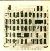
Video Display Board—Zilog's Z80-VDB Video Display Board interfaces the company's standard Z80-MCB directly to TTL horizontal, vertical and video drives of a standard TV monitor. The unit contains 256 bytes of dynamic RAM for line buffering to the MCB, and accommodates 64 upper case ASCII characters and display size of 24 lines, 80 characters per line. Price of the Z80-VDB Is \$475. Circle 61 on Reader Service Coupon for more information about this product or others by this manufacturer.
