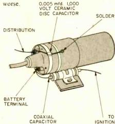
Those annoying popping sounds, which can be traced to the ignition system, can be readily cured. Install a coaxial capacitor at the coil's battery terminal and a .005-uF, 1,000 VDC, disc capacitor to distributor.
