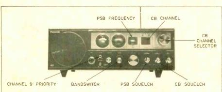
Though the Panasonic RJ-3660 combines an FM PSB receiver and an AM CB transceiver in the same cabinet, the front panel isn't cluttered or complicated. Major differences is a PSB tuning dial in addition to the digital CB channel indicator, and separate squelch controls for each receiver. You'll be sure to find the PSB receiver a useful addition, especially in time of emergency when your CB is most important. For more information circle No. 67 on the Reader Service Coupon.
