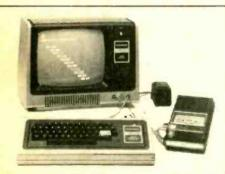
Radio Shack System—Radio Shack's TRS-80 microcomputer system consists of a 53-key professional type keyboard and microcomputer plus regulated power supply, a computer-controlled data cassette recorder and a 12-inch video display monitor. The complete system is priced at \$599.95 but the microcomputer alone is available for \$399.95. The microprocessor is an advanced Z-80 8-bit processor. The video display is memory mapped, all graphics and alphanumerics controlled by BASIC
