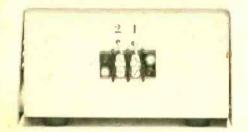
This back view of the Changer shows the barrier terminal strip and its two interconnection points to connect to the scanner.
