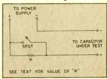
The resistor value R in this test circuit to find leakage is explained in the text.
