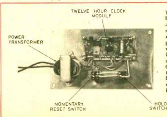
The Midget Digit is built around a standard twelve hour clock module. The module consists of a small printed circuit board with an oversize red filter that conceals several relatively large 0.5-inch LEDs. Though the LEDs are rather bright when on, they will not normally fog B&W enlarging paper.
