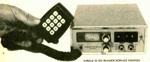
The Heathkit HW-2036 with the optional Micoder. The Micoder combines its microphone with a touchtone pad for accessing an auto-patch. The pad can only be used when the PTT switch is held down. A small LED directly above the "2" glows to indicate a numeral has been keyed into the transmitter, producing a tone.
