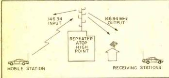
Basic repeater operation is very simple. Here we have a repeater operating 34/94. A mobile station may transmit on the input of 146.34 MHz and the repeater will retransmit on 146.94 MHz with a higher powered signal.
