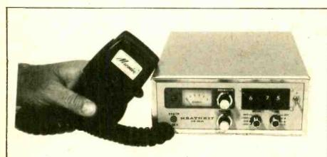
Front view of the HW-2036 with the Micoder shown on its speaking side. Inside the Micoder, besides its touch-tone pad crcuitry, and its 9-volt battery, is an exceptionally sensitive and high-quality electret microphone element. This combination of mike element and audio circuitry makes for some really great audio quality.
