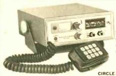
Heath's popular HW-2036 is a synthesized two-meter rig which offers hundreds of channels. Available accessories include a PL encoder built into a microphone, and an AC power supply for use in the home.
