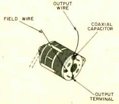
An alternator can often be stopped from whining by the installation of a coaxial capacitor at the alternator's output wire.
