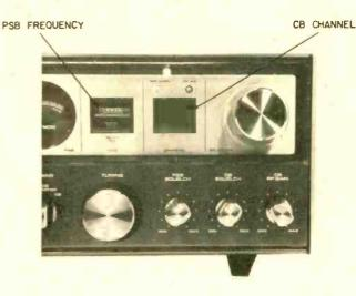
The blackout window displays the CB channel when the CB section is switched in for operation or monitoring. The window blacks out when the channel 9 priority switch is activated. Note the separate squelch controls for PSB and CB. This keeps the background quiet when monitoring PSB with CB override switched in.
