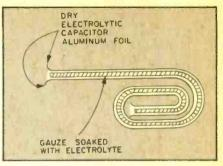
Cross section showing the internal construction of a "dry" electrolytic capacitor. Two sheets of aluminum foil are rolled up with a strip of electrolyte-saturated gauze between.
