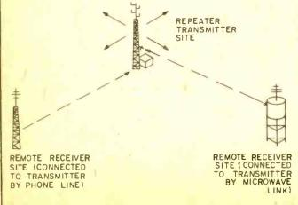
More complicated repeater arrangements may involve more than one repeater site. The repeaters may be twenty or more miles apart. All the remote receivers transmit their signals simultaneously to the main repeater (via the phone line or microwave). A switching device at the main site chooses, and then rebroadcasts the best signal from the remote stations.
